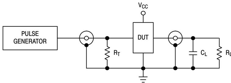
$C_L = 50$  pF or equivalent (Includes jig and probe capacitance)
