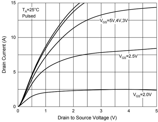
Fig. 2 - Transfer Characteristics
