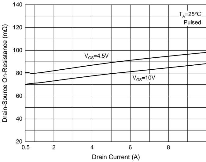
Fig. 4 -  $R_{DS(ON)} - V_{GS}$
