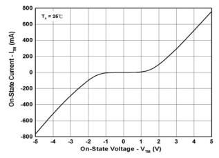
Fig 2 On-State Characteristics
