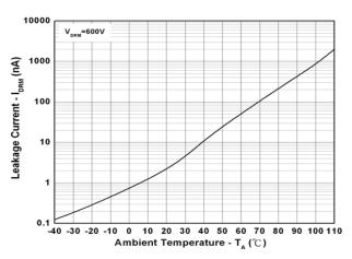
Fig 7 Leakage Current vs Ambient Temperature
