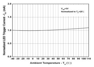
Fig 4 Normalized LED Trigger Current vs Ambient Temperature
