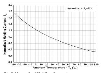
Fig 5 Normalized Holding Current vs Ambient Temperature
