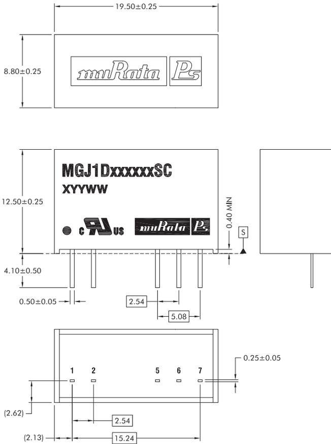
All dimensions in mm. All pins on a 2.54 pitch and within ±0.1 of true position from pin 1 at seating plane 'S'.
