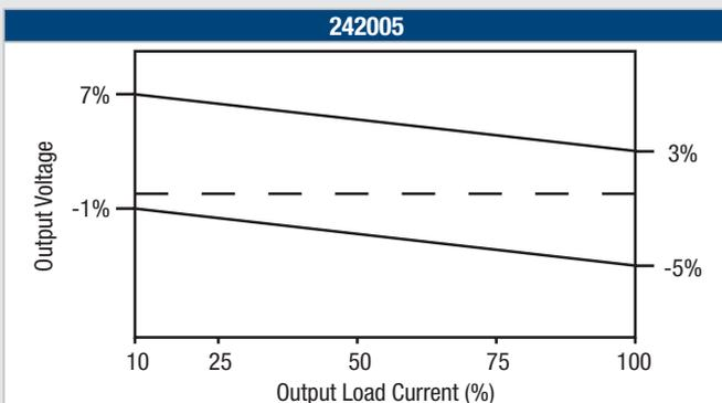
**NEGATIVE OUTPUT VOLTAGE TOLERANCE ENVELOPES**
