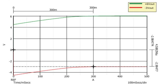
To avoid spurious gate pulses it is recommended that the PWM gate signal is not applied until after the settling time has ended.
