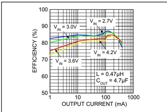
**FIGURE 2-2:** Efficiency ( $V_{OUT} = 1.8V$ ).
