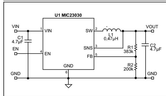
**FIGURE 4-1:** MIC23030-AYMT Schematic.
