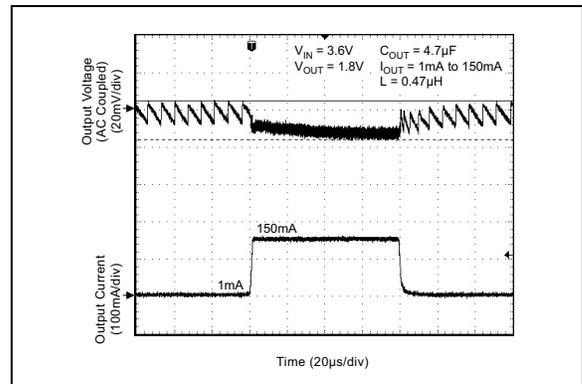
**FIGURE 2-23:** Load Transient.
