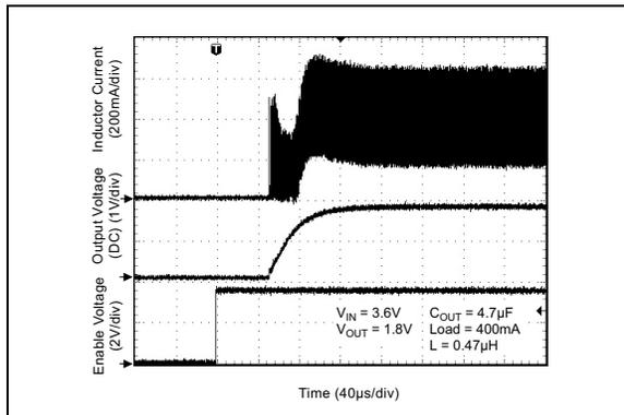
**FIGURE 2-21:** Start-Up Waveform.
