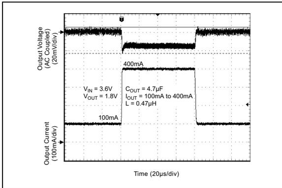
**FIGURE 2-26:** Load Transient.
