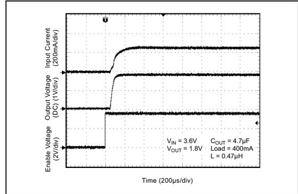
**FIGURE 2-22:** Start-Up Waveform.
