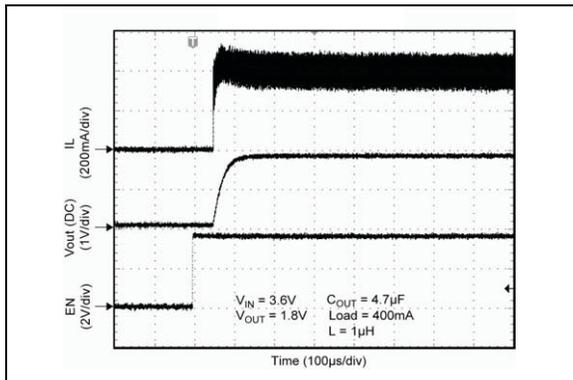
**FIGURE 2-21:** Start-Up Waveform.
