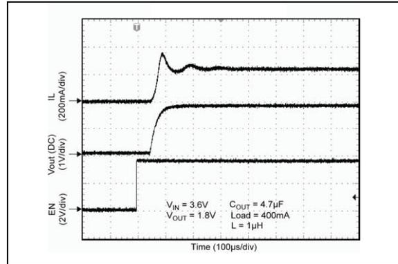
**FIGURE 2-22:** Start-Up Waveform.
