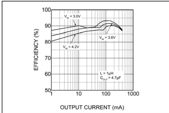
**FIGURE 2-1:** Efficiency ( $V_{OUT} = 2.5V$ ).
