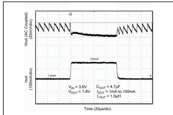
**FIGURE 2-23:** Load Transient.
