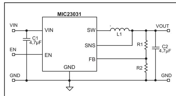
**FIGURE 4-1:** MIC23031-AYMT Schematic.
