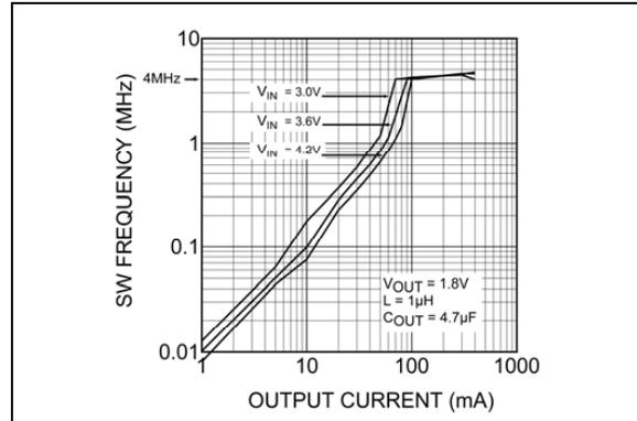
**FIGURE 2-10:** Switching Frequency vs. Output Current.
