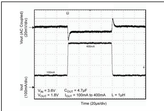
**FIGURE 2-26:** Load Transient.
