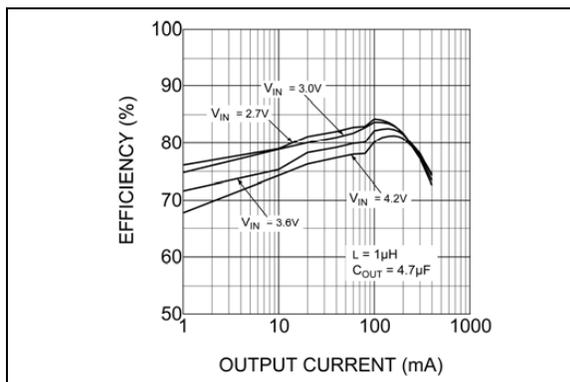
**FIGURE 2-3:** Efficiency ( $V_{OUT} = 1.2V$ ).
