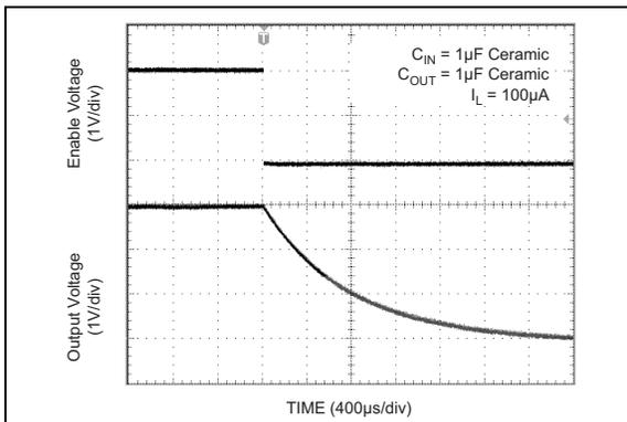
**FIGURE 2-21:** Shutdown Delay.
