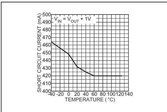
**FIGURE 2-14:** Short-Circuit Current.
