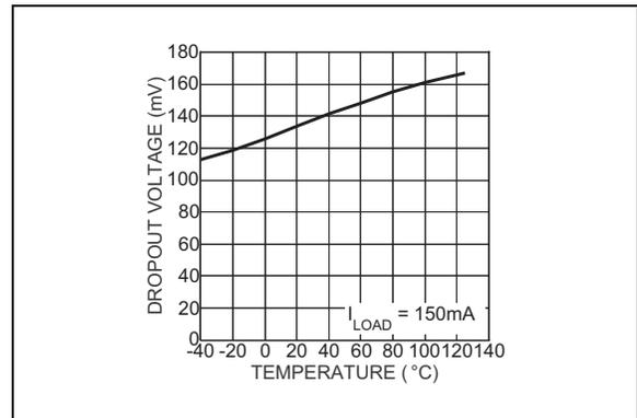
**FIGURE 2-11:** Dropout Voltage.
