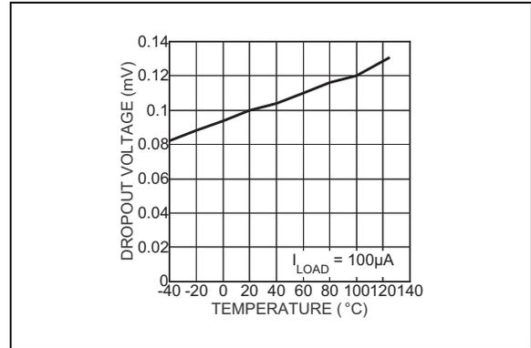
**FIGURE 2-10:** Dropout Voltage.
