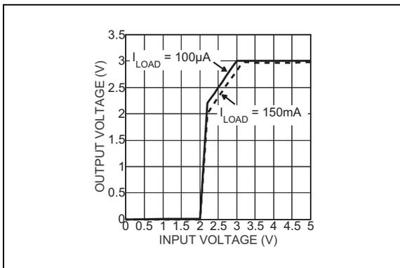
**FIGURE 2-9:** Dropout Characteristics.
