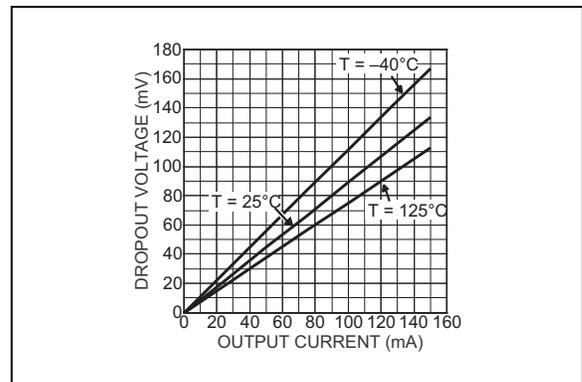
**FIGURE 2-12:** Dropout Voltage.
