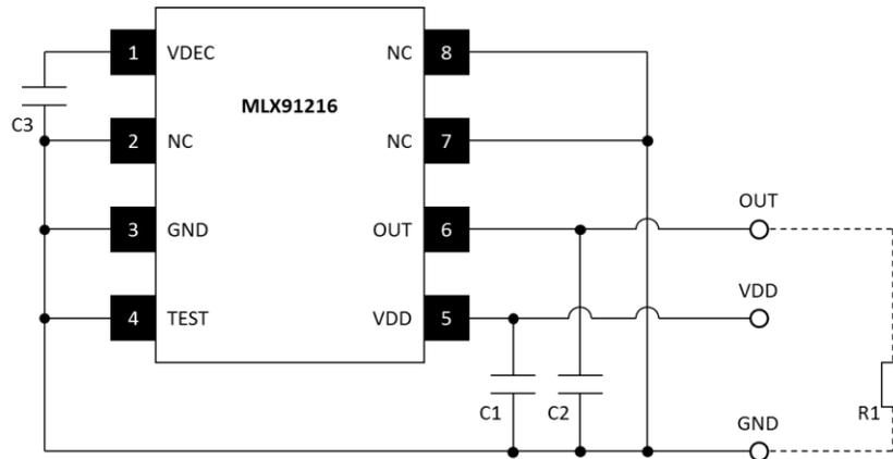
Figure 4: Application Diagram with external Pull-Down resistance
