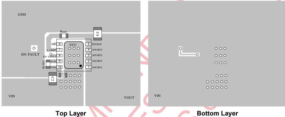
**Figure3 — PCB Layout**
