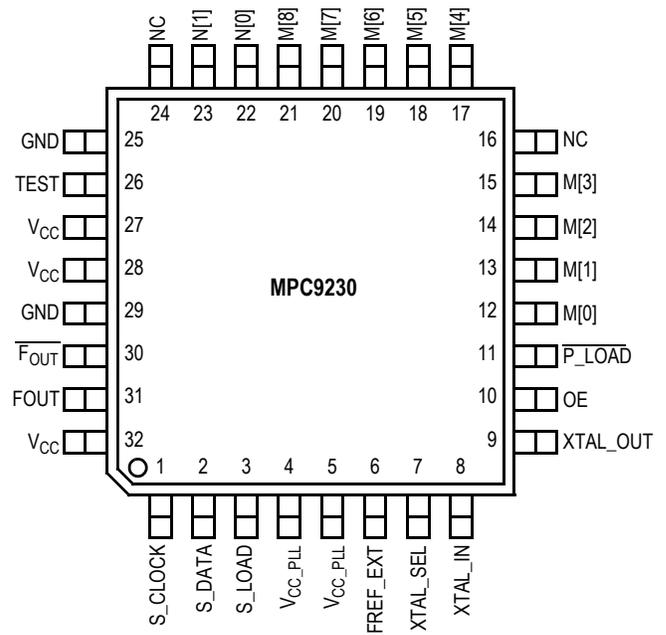
Figure 3. MPC9230 32-Lead Package Pinout (Top View)
