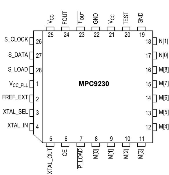
Figure 2. MPC9230 28-Lead PLCC Pinout (Top View)
