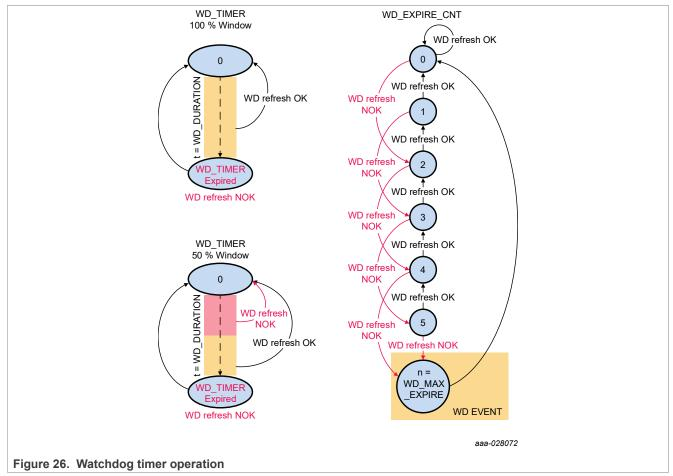
The watchdog function can be enabled or disabled by writing the WD\_EN bit in the  $I^2$ C register map. When the I2C SECURE EN = 1, a secure write must be performed to change the WD\_EN bit.
