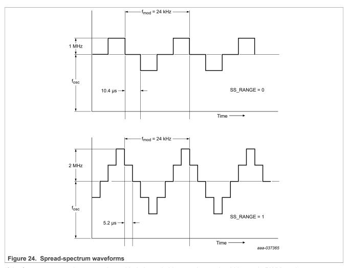
If the frequency spread-spectrum is enabled, the switching regulators should be set in PWM mode to ensure clock synchronization at all time.
