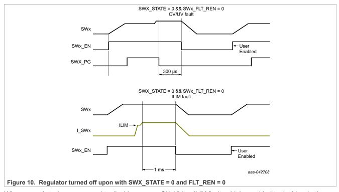
When a regulator is programmed to disable upon an OV, UV, or ILIM fault, a bit is provided to decide whether a regulator can return to its previous configuration or remain disabled when the fault condition is cleared.
