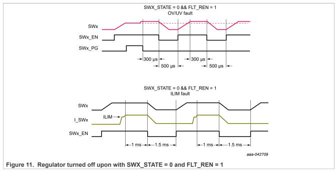
To avoid fault cycling, a global fault counter is provided. Each time any of the external regulators encounter a fault event, the PF5200 compares the value of the FAULT\_CNT[3:0] against the FAULT\_MAX\_CNT, and if it not equal, it increments the FAULT\_CNT[3:0] and proceeds with the fault protection mechanism.
