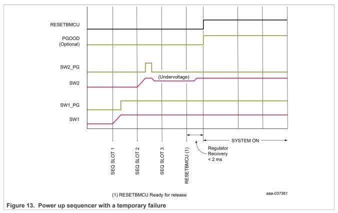
If the faulty condition is not cleared within the 2.0 ms timer, the power up sequence is aborted and the PF5200 turns off all voltage regulators enabled so far as shown in <u>Figure 14</u>.
