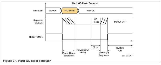
Every time a WD event occurs, the WD\_EVENT\_CNT[3:0] nibble is incremented. To prevent continuous failures, if the WD\_EVENT\_CNT[3:0] = WD\_MAX\_CNT[3:0] the state machine will proceed to the fail-safe transition. The MCU is expected to clear the WD\_EVENT\_CNT[3:0] when it is able to do so in order to keep proper operation. Upon power up, the WD\_MAX\_CNT[3:0] is loaded with the values on the OTP\_WD\_MAX\_CNT[3:0] bits.
