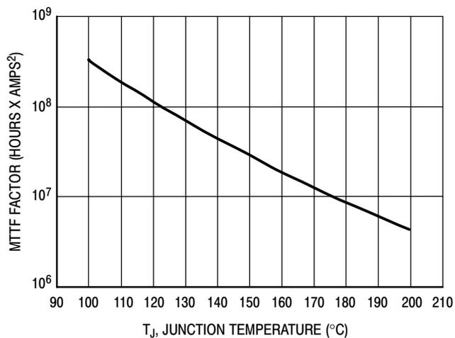
This above graph displays calculated MTTF in hours x ampere<sup>2</sup> drain current. Life tests at elevated temperatures have correlated to better than ±10% of the theoretical prediction for metal failure. Divide MTTF factor by  $I_D^2$  for MTTF in a particular application.
