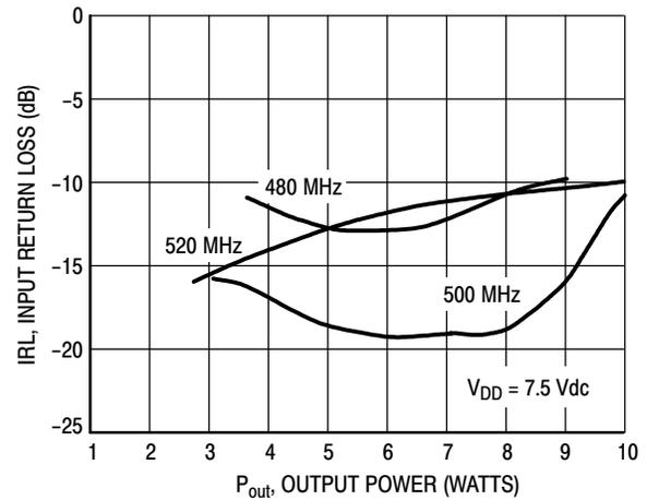
Figure 3. Input Return Loss versus Output Power
