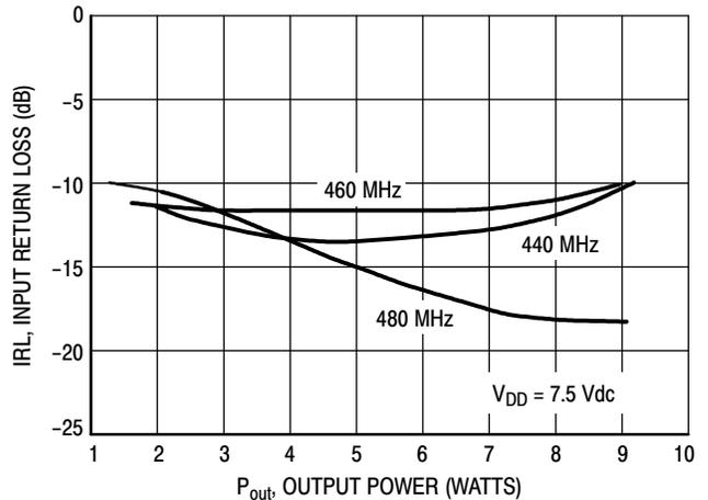
Figure 21. Input Return Loss versus Output Power
