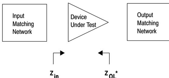
Figure 29. Series Equivalent Input and Output Impedance
