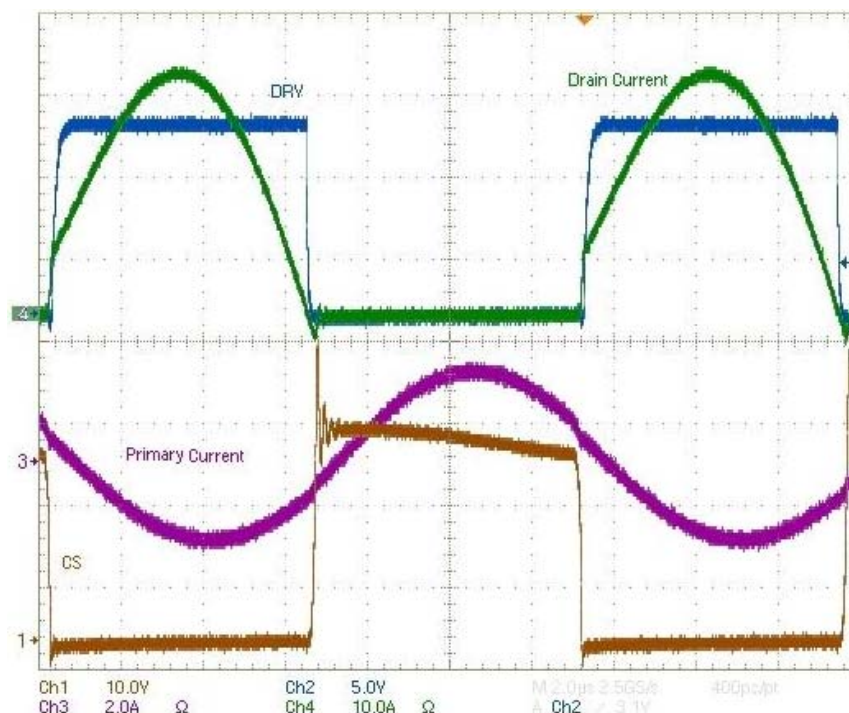
Figure 49. Waveforms from SR System Implemented in LLC Application and Using MOSFET in SMT Package with Minimized Parasitic Inductance – SR MOSFET Channel Conduction Time is Optimized
