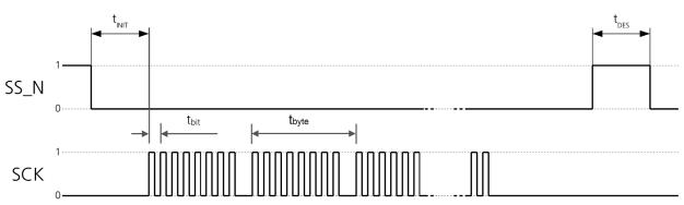
Figure 3: SPI timing diagram
