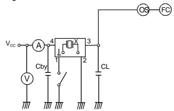
CL; 15pF MAX including input capacity of oscilloscope
