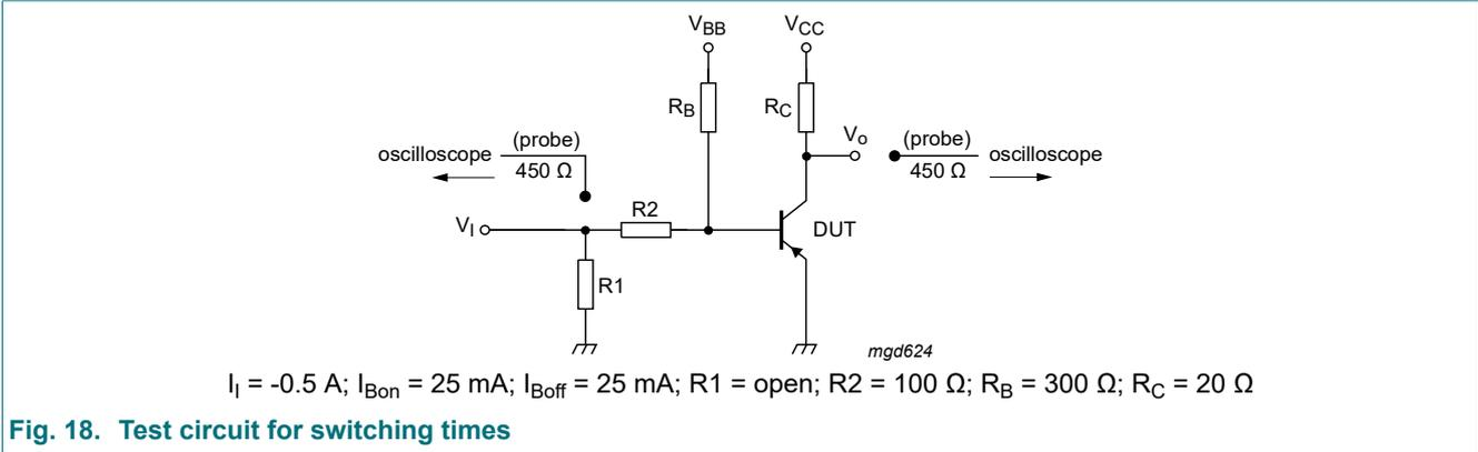
Fig. 18. Test circuit for switching times
