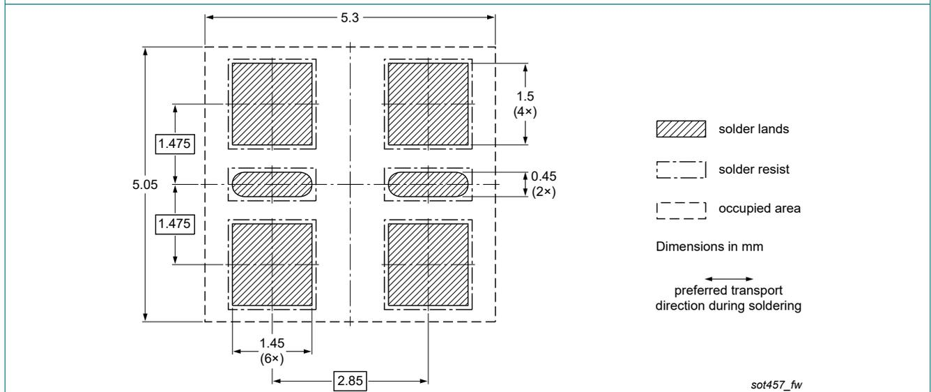
Fig. 21. Wave soldering footprint for TSOP6 (SOT457)
