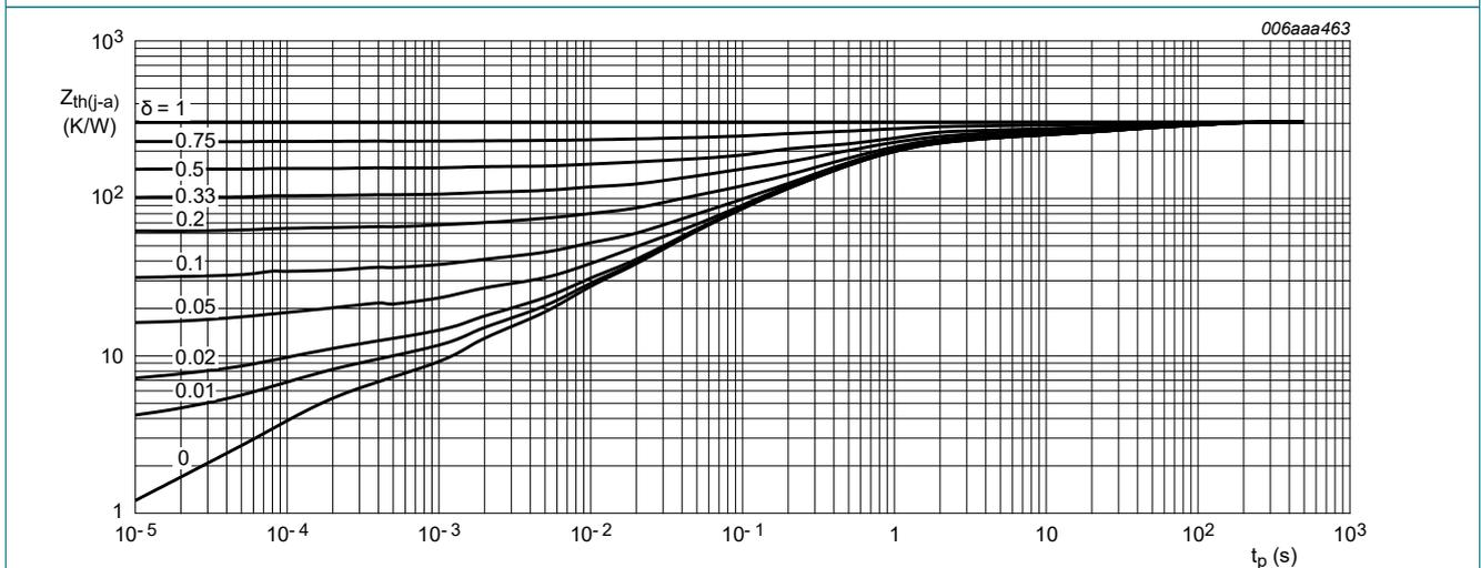
Fig. 3. TR1 (PNP): Transient thermal impedance from junction to ambient as a function of pulse duration; typical values
