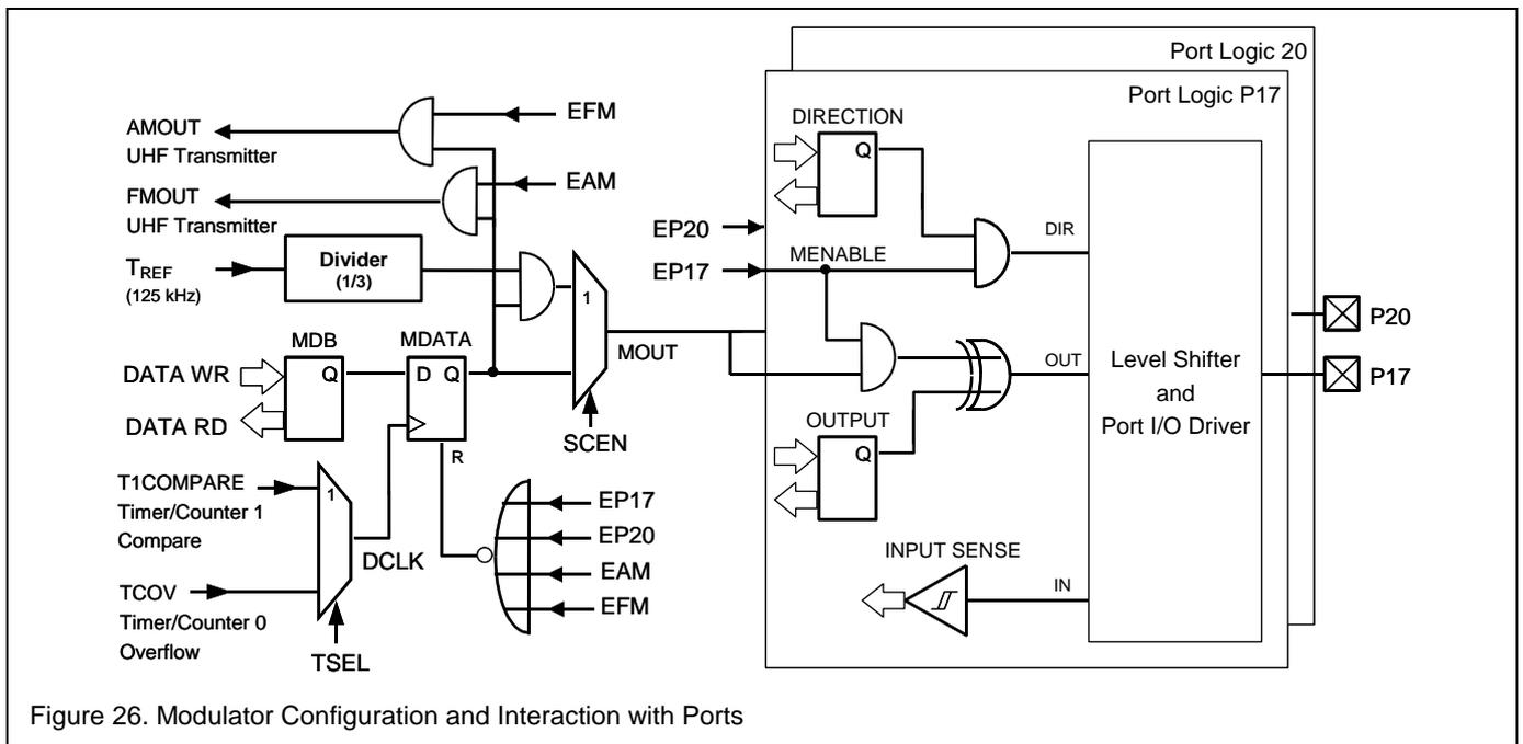
Figure 26. Modulator Configuration and Interaction with Ports
