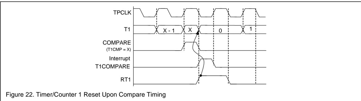
Figure 22. Timer/Counter 1 Reset Upon Compare Timing
