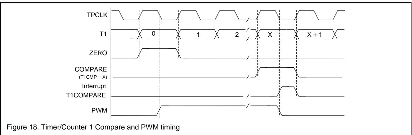
Figure 18. Timer/Counter 1 Compare and PWM timing
