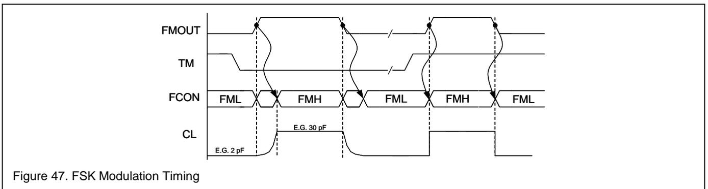
Figure 47. FSK Modulation Timing
