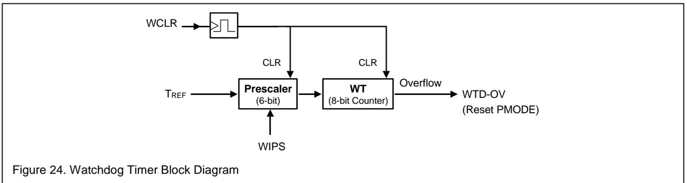
Figure 24. Watchdog Timer Block Diagram
