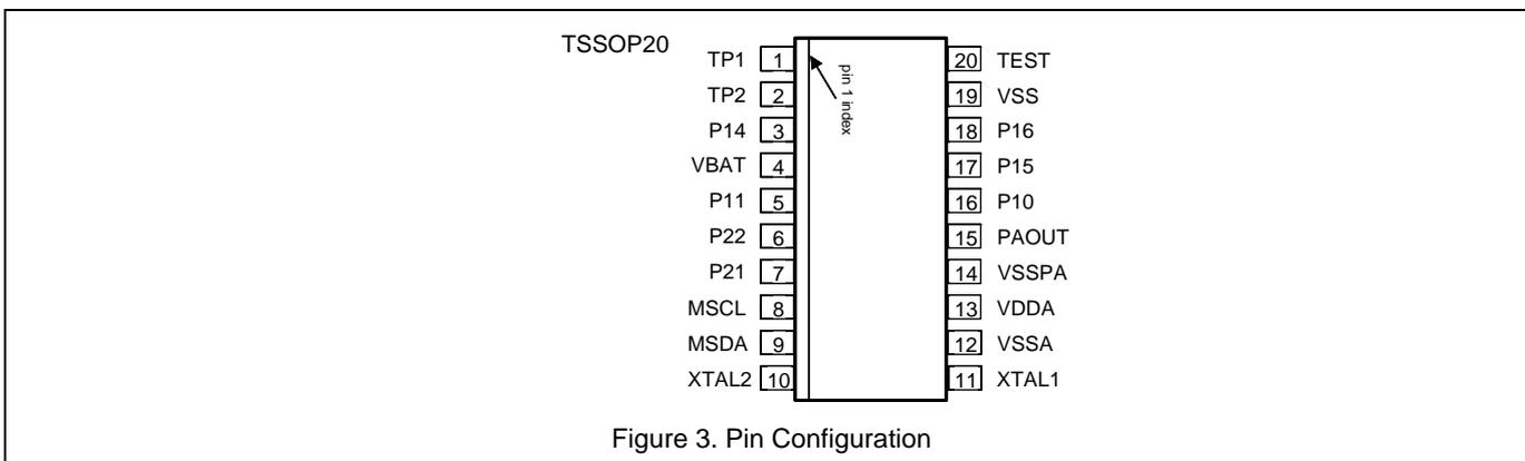
Figure 3. Pin Configuration
