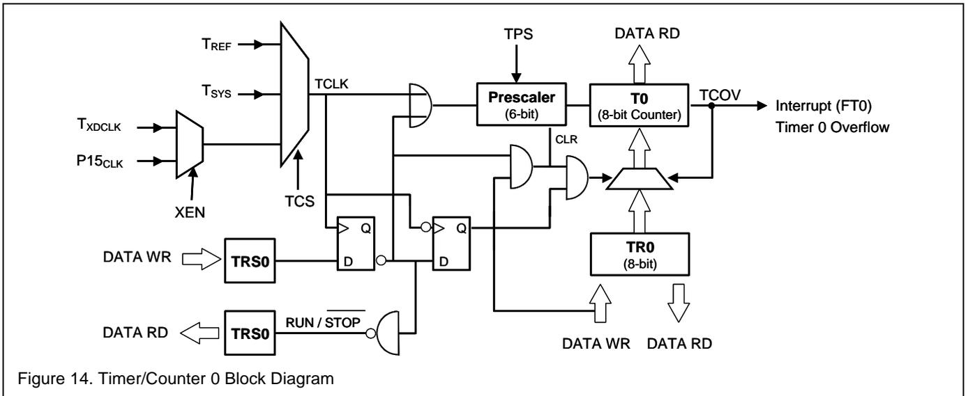
Figure 14. Timer/Counter 0 Block Diagram
