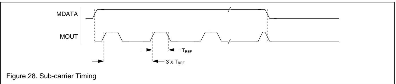
Figure 28. Sub-carrier Timing
