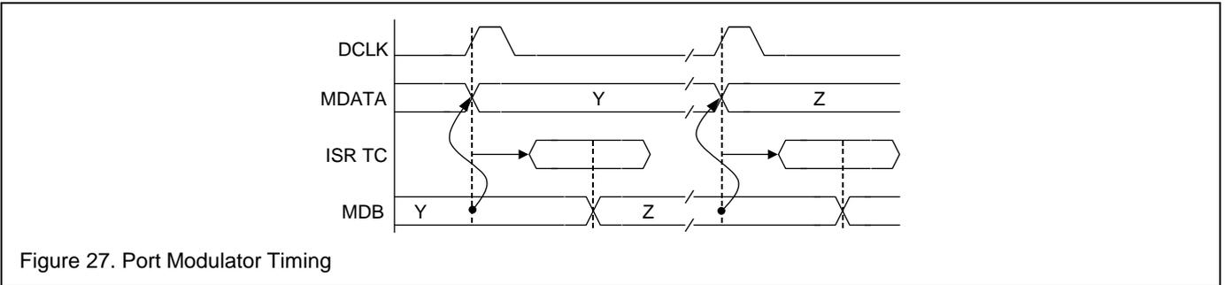
Figure 27. Port Modulator Timing
