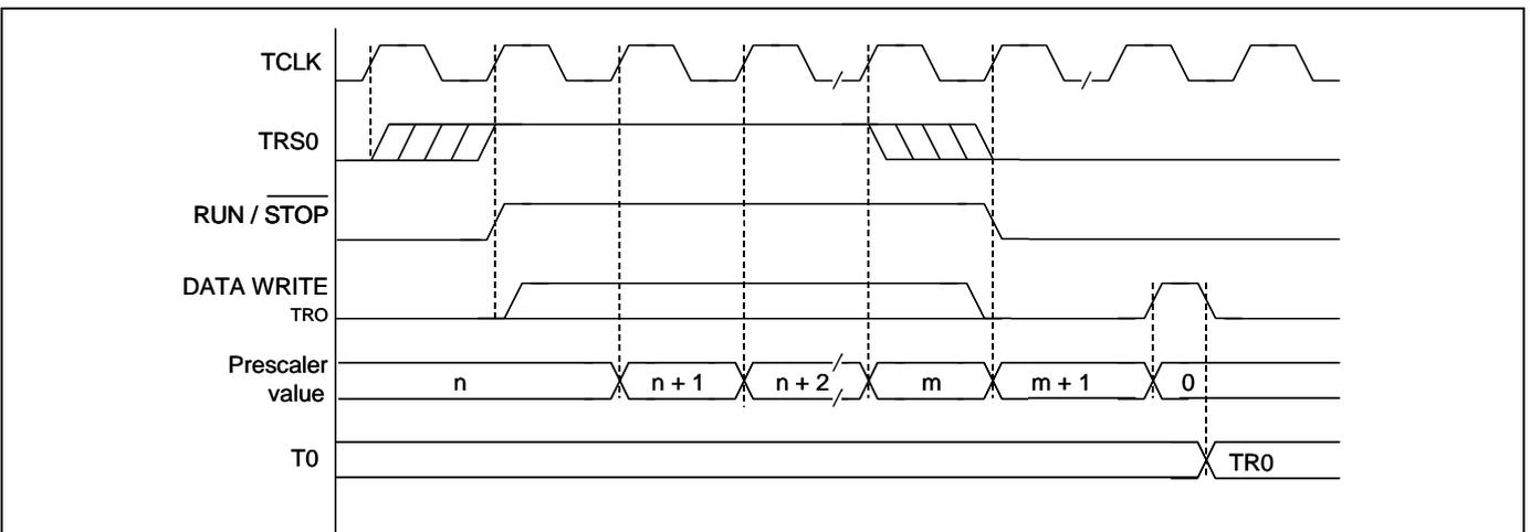
Figure 15. Timer/Counter 0 Timing
