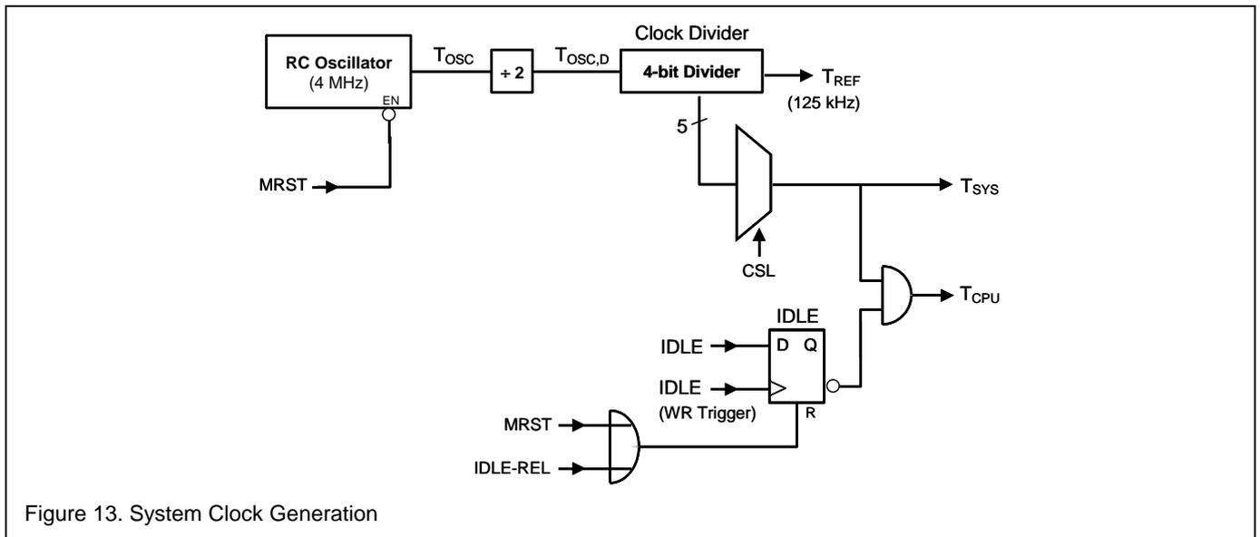
Figure 13. System Clock Generation
