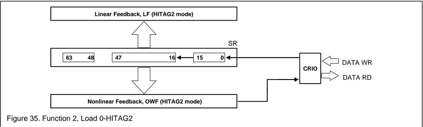
Figure 35. Function 2, Load 0-HITAG2
