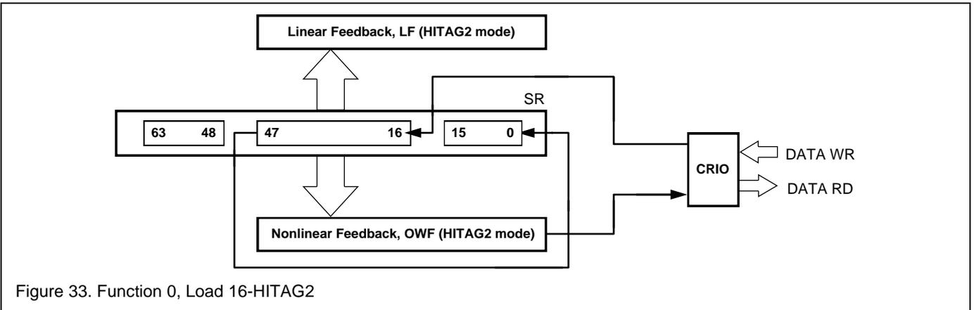
Figure 33. Function 0, Load 16-HITAG2
