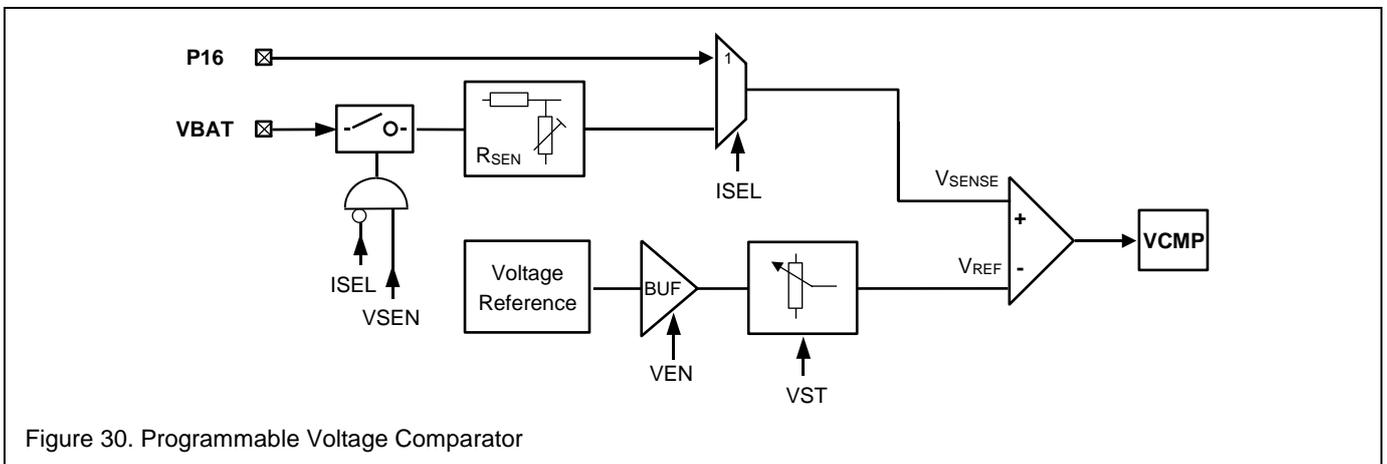
Figure 30. Programmable Voltage Comparator
