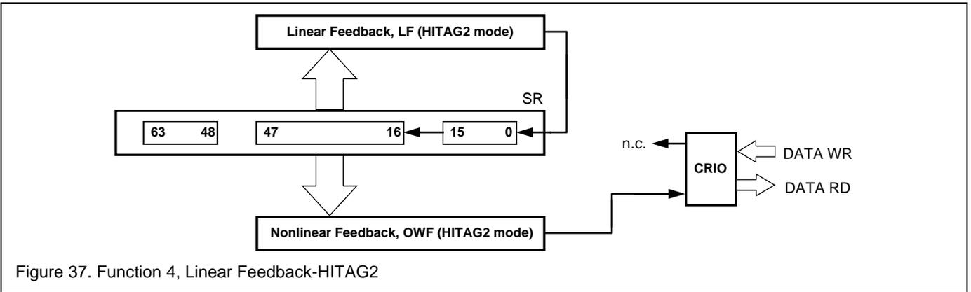
Figure 37. Function 4, Linear Feedback-HITAG2
