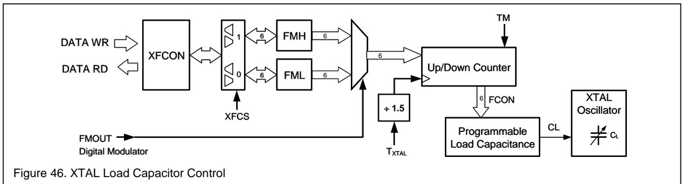
Figure 46. XTAL Load Capacitor Control
