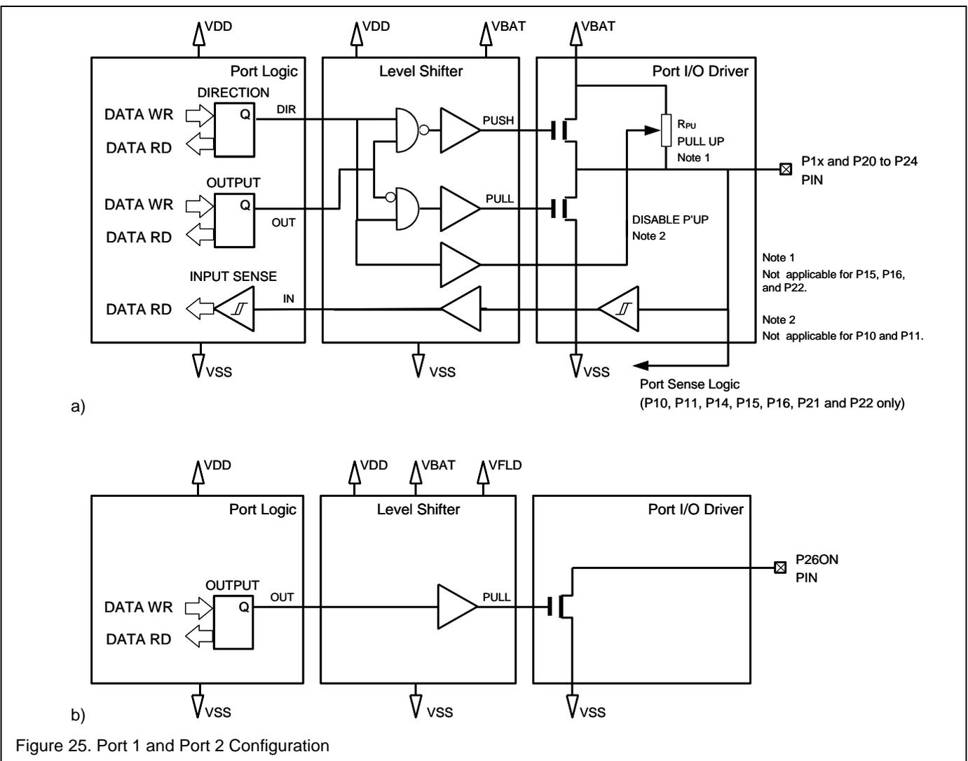
Figure 25. Port 1 and Port 2 Configuration
