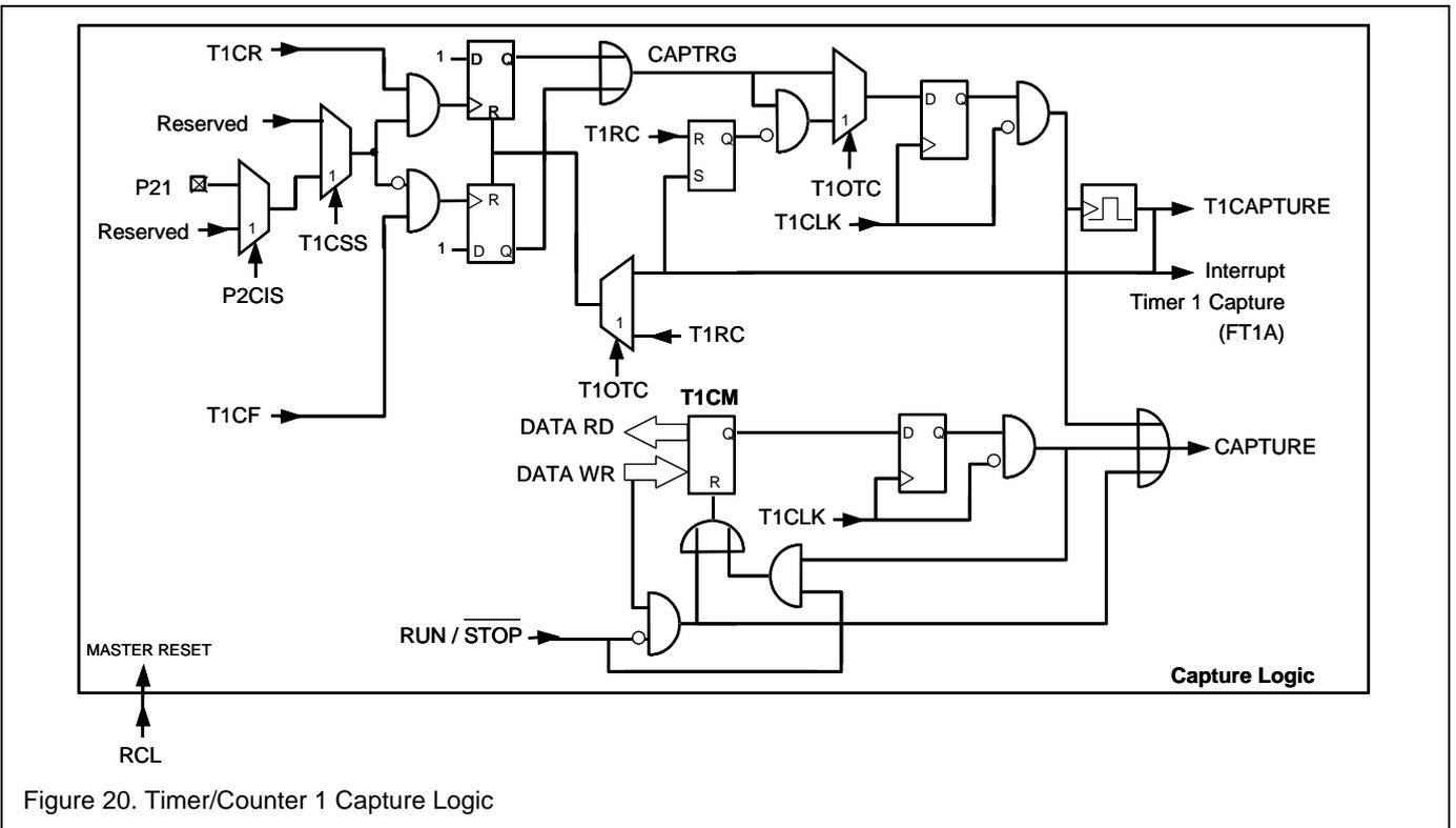
Figure 20. Timer/Counter 1 Capture Logic
