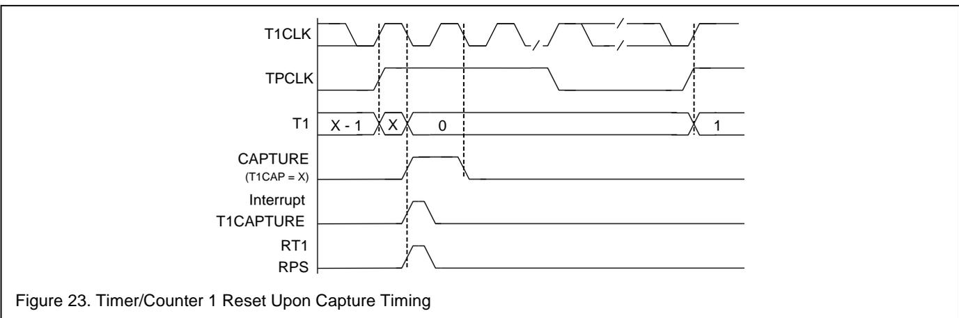
Figure 23. Timer/Counter 1 Reset Upon Capture Timing
