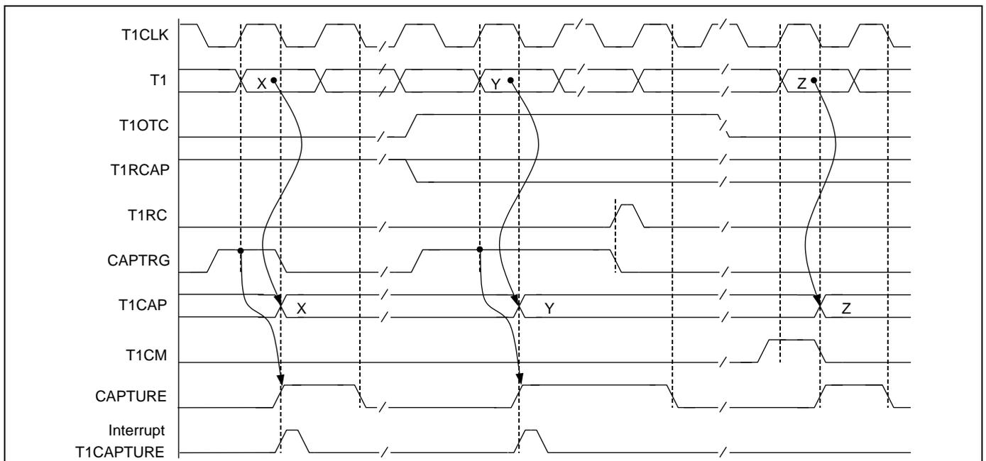
Figure 21. Timer/Counter 1 Capture Logic Timing
