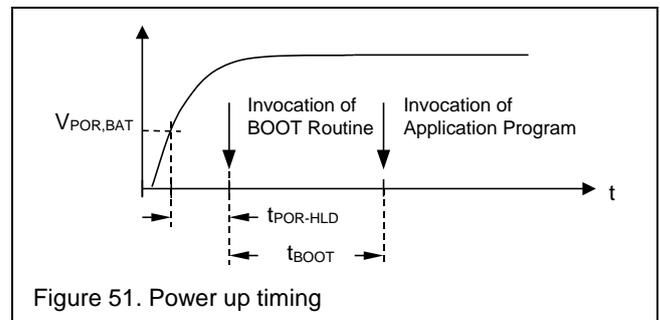
Figure 51. Power up timing
