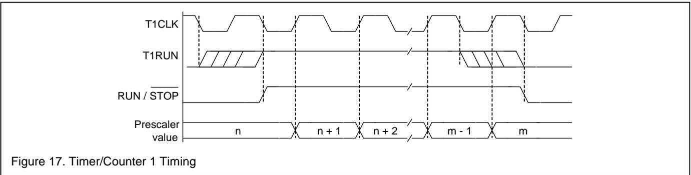
Figure 17. Timer/Counter 1 Timing
