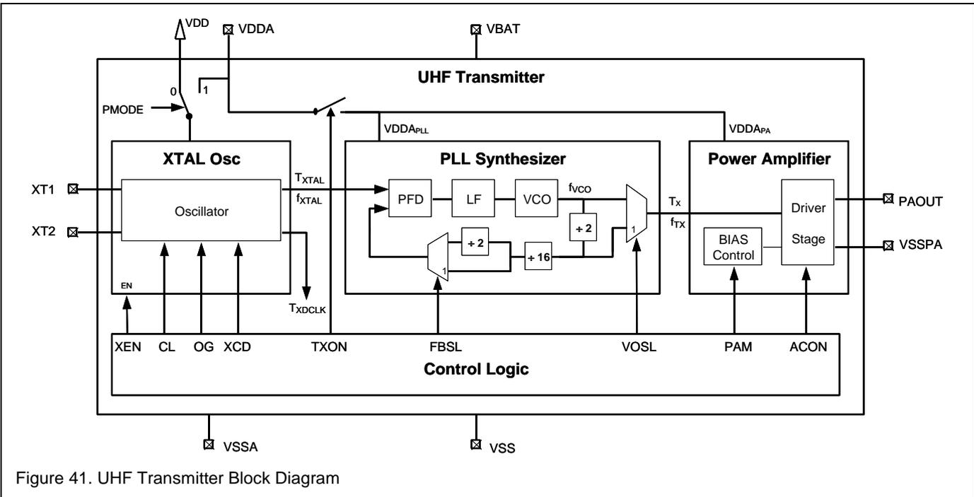
Figure 41. UHF Transmitter Block Diagram
