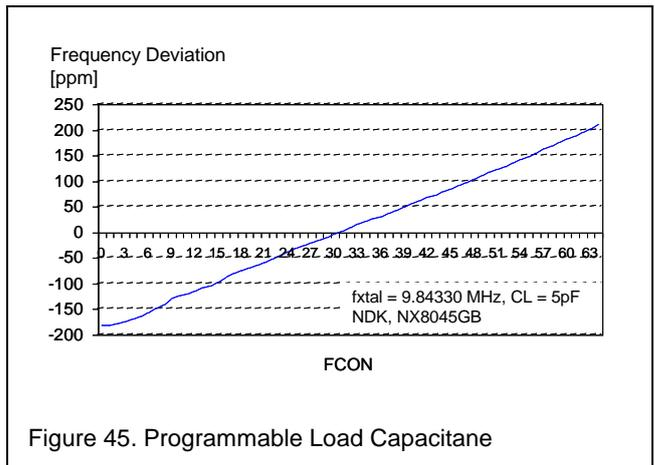
Figure 45. Programmable Load Capacitance
