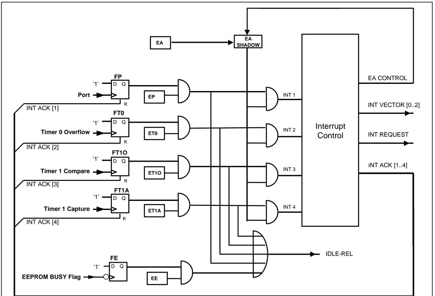
Figure 12. Interrupt and IDLE Control System
