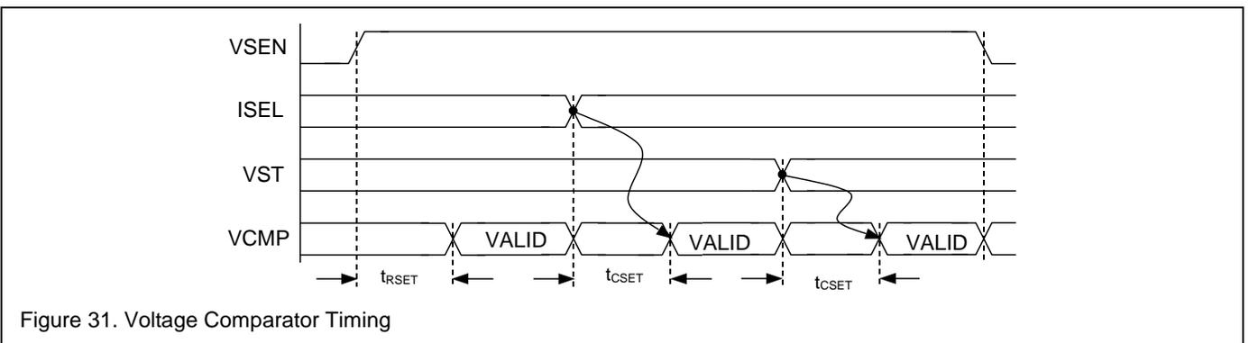
Figure 31. Voltage Comparator Timing
