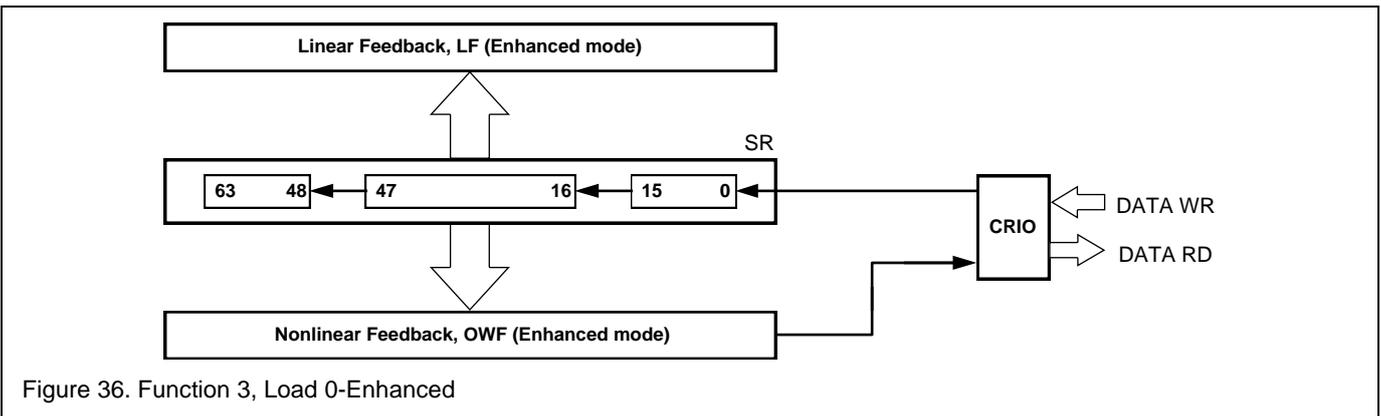
Figure 36. Function 3, Load 0-Enhanced
