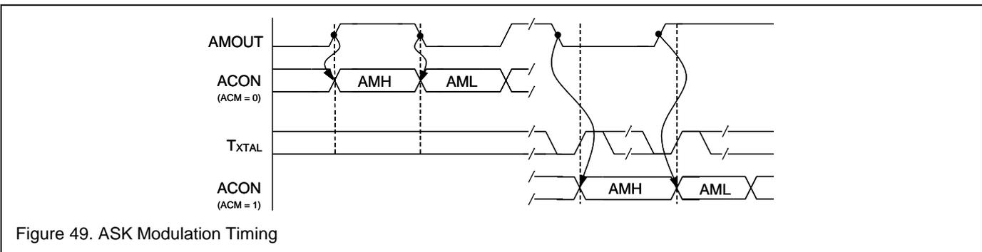
Figure 49. ASK Modulation Timing
