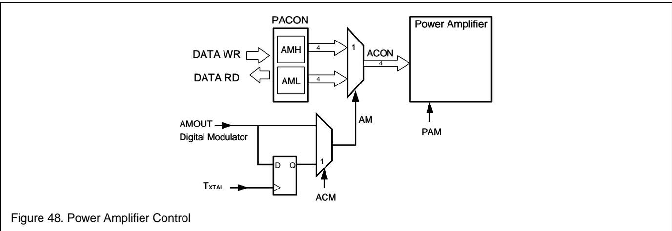
Figure 48. Power Amplifier Control
