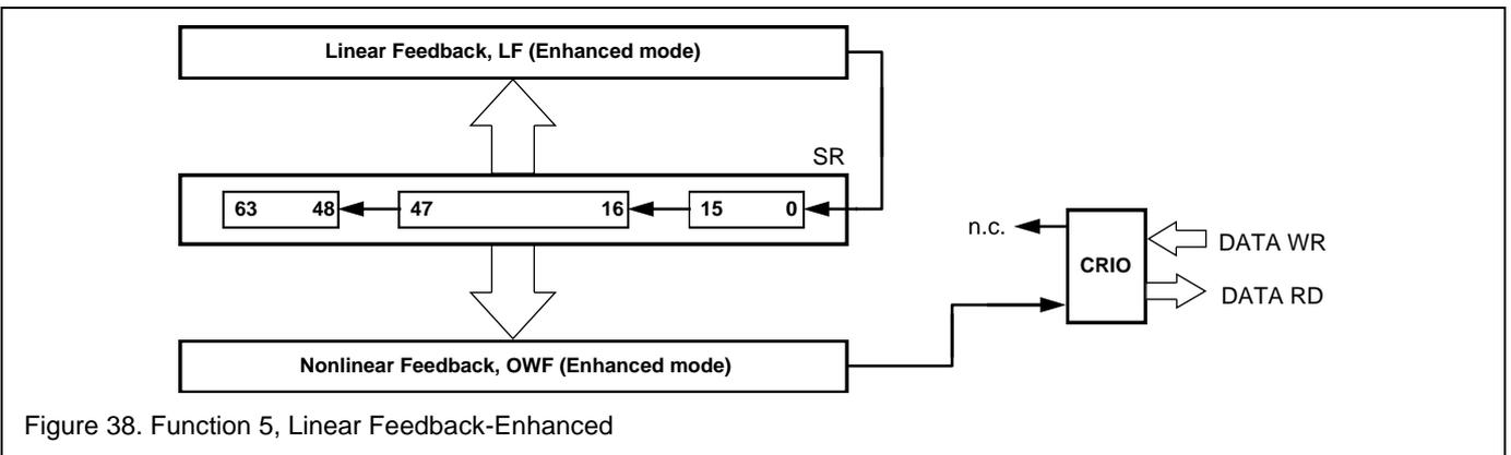
Figure 38. Function 5, Linear Feedback-Enhanced
