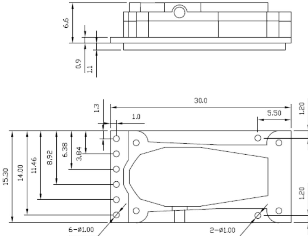
\* Module Total Dimension: 30.0mm (W) x 15.3mm (L) x 7.7mm (H)
