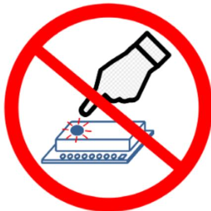
**Do not touch or remove the particle filter!**
