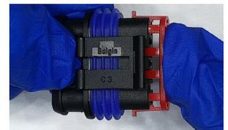
When contacts are in place, insert the appropriate wedgelock until a click is heard. Once male and female housings are prepared the parts can be mated
