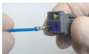
Line the contact up with the grommet.
