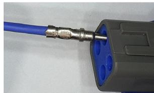
Line the contact up with the grommet.
