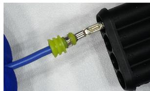
Line the contact up with the grommet.
