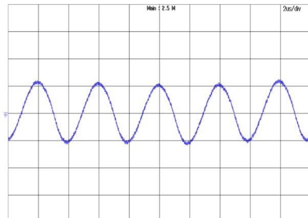
**Figure 30:** Output voltage ripple at  $V_{in}=72V$  and full load
