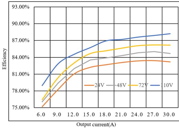
**Figure 1:** Efficiency vs. load current at 25°C.
