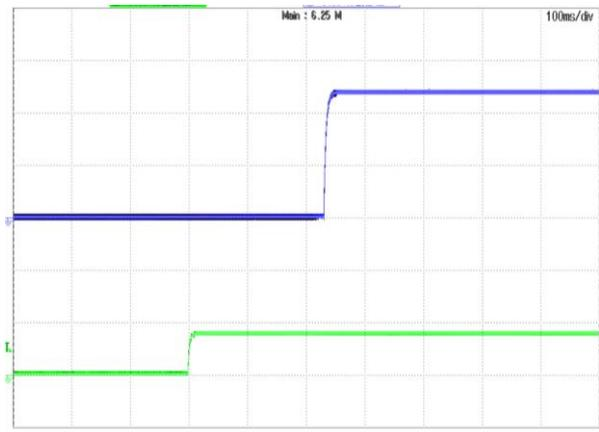
**Figure 10:** Turn-on transient at full load current (100ms/div).
