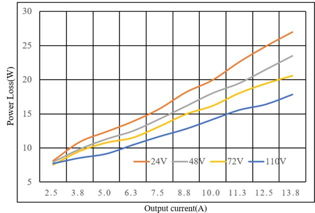
**Figure 8:** Power loss vs. load current at 25°C.
