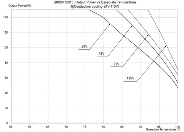
**Figure 35:** Output power vs. base plate temperature
