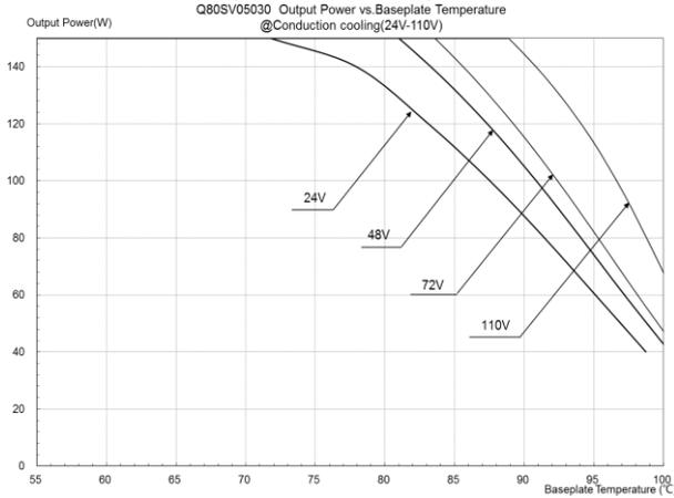
**Figure 34:** Output power vs. base plate temperature
