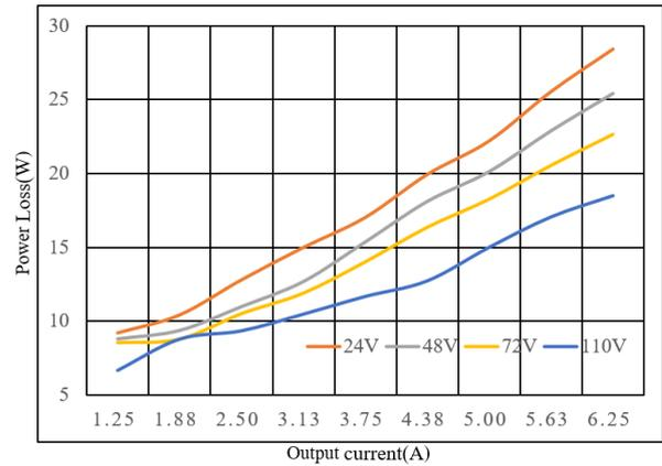
Figure 20: Power loss vs. load current at 25°C.
