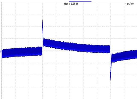
**Figure 11:** Output voltage response to step-change in load current (50%-75%-50% of full load;  $di/dt = 0.1A/\mu s$ ).
