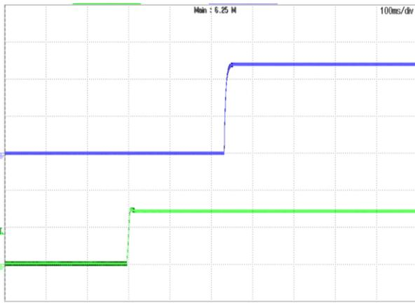
**Figure 9:** Turn-on transient at full load current (100ms/div).
