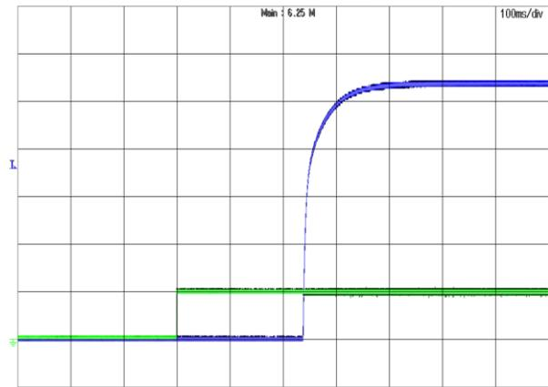
**Figure 28:** Turn-on transient at full load current (100ms/div).
