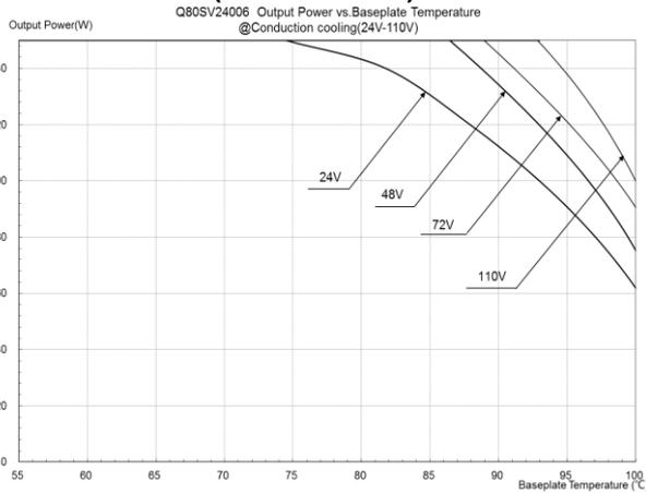
**Figure 36:** Output power vs. base plate temperature
