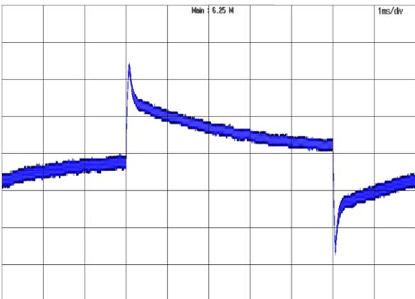
Figure 23: Output voltage response to step-change in load current (50%-75%-50% of full load;  $di/dt = 0.1A/\mu s$ ).
