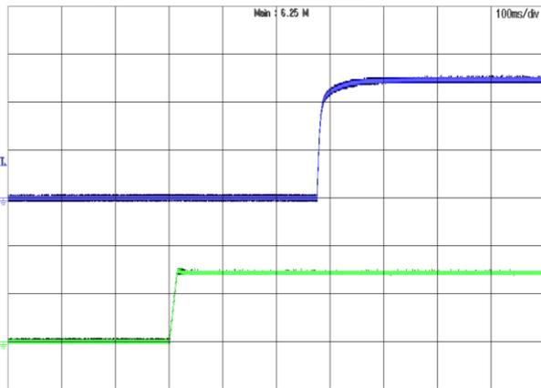
**Figure 3:** Turn-on transient at full load current (100ms/div).
