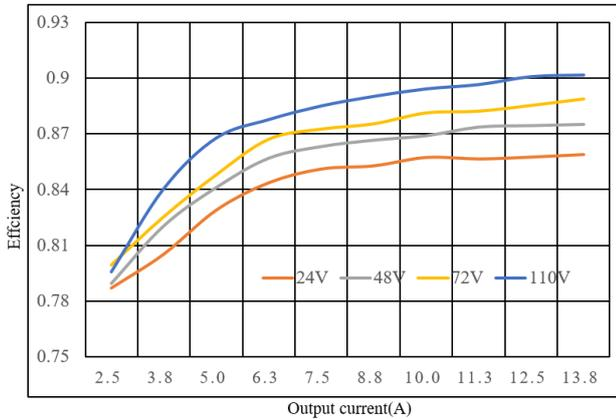
**Figure 7:** Efficiency vs. load current at 25°C.
