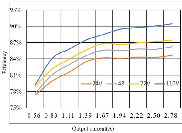
**Figure 25:** Efficiency vs. load current at 25°C.
