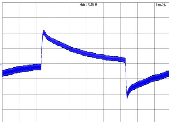
**Figure 29:** Output voltage response to step-change in load current (50%-75%-50% of full load;  $di/dt = 0.1A/\mu s$ ).
