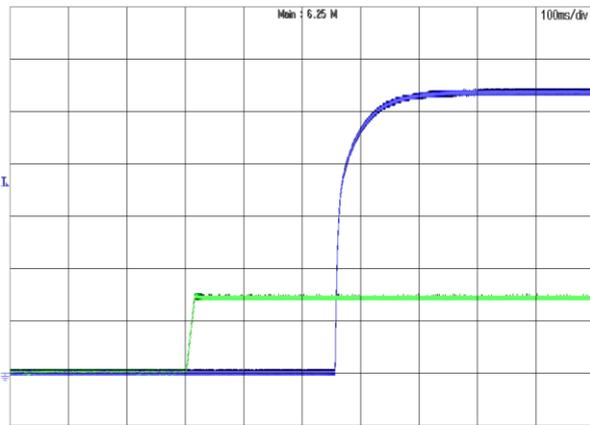
**Figure 27:** Turn-on transient at full load current (100ms/div).
