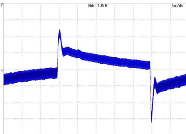
**Figure 17:** Output voltage response to step-change in load current (50%-75%-50% of full load;  $di/dt = 0.1A/\mu s$ ).
