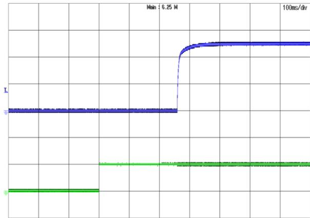
**Figure 4:** Turn-on transient at full load current (100ms/div).
