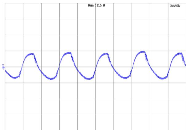
**Figure 6:** Output voltage ripple at  $V_{in}=72V$  and full load
