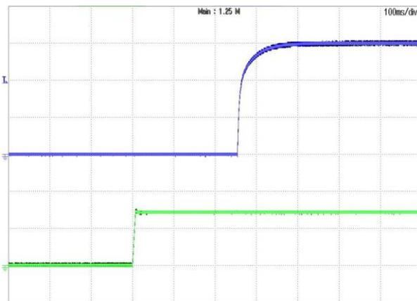
**Figure 15:** Turn-on transient at full load current (100ms/div).
