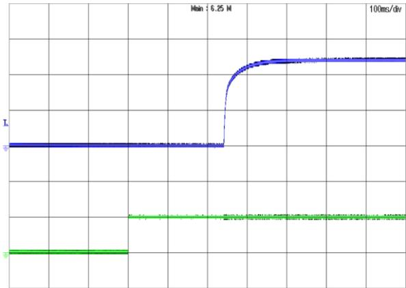
Figure 22: Turn-on transient at full load current (100ms/div).
