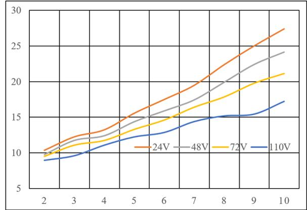
**Figure 14:** Power loss vs. load current at 25°C.
