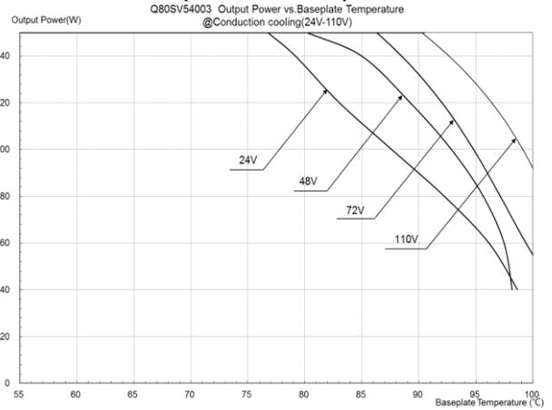
**Figure 37:** Output power vs. base plate temperature
