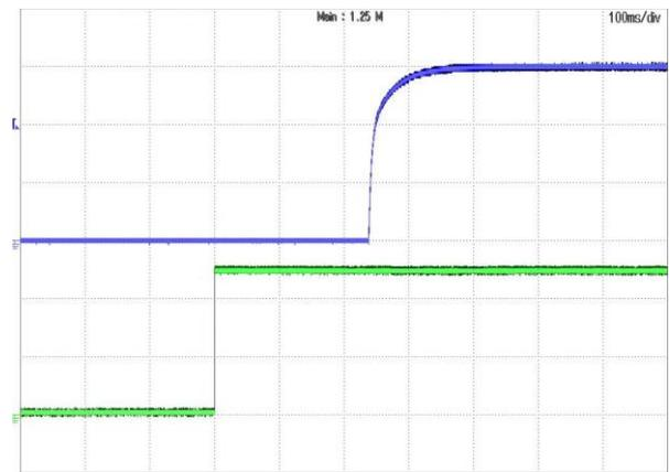
**Figure 16:** Turn-on transient at full load current (100ms/div).
