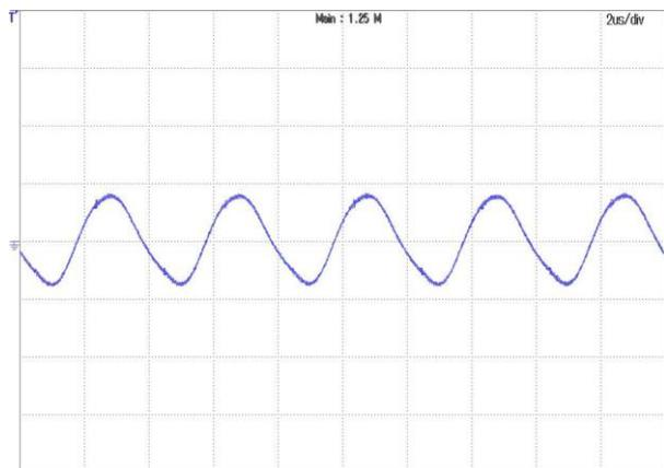
**Figure 18:** Output voltage ripple at  $V_{in}=72V$  and full load
