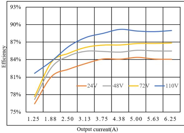
Figure 19: Efficiency vs. load current at 25°C.
