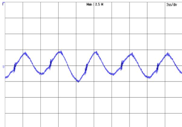
Figure 24: Output voltage ripple at  $V_{in}=72V$  and full load
