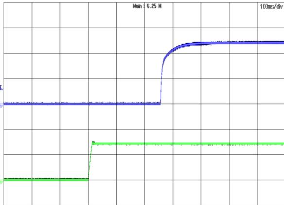
Figure 21: Turn-on transient at full load current (100ms/div).
