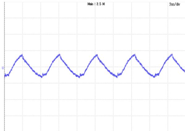
**Figure 12:** Output voltage ripple at  $V_{in}=72V$  and full load
