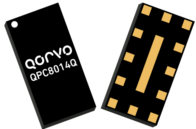
13 Pin 1.1 x 1.9 x 0.44 mm Module Package
