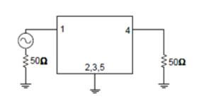
Notes: Blocking capacitors are required on any RF ports where a DC voltage may be present.
