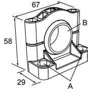
**Hole center spacing:** A=ø 50.8
