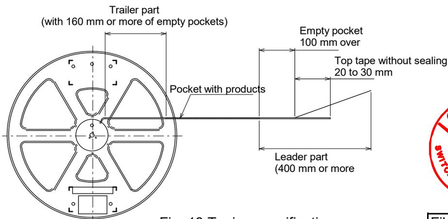
Fig. 13 Taping specification Δ4
