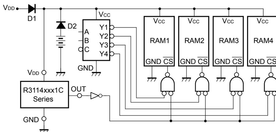
• **Voltage level Indicator Circuit (lighted when the power runs out)
