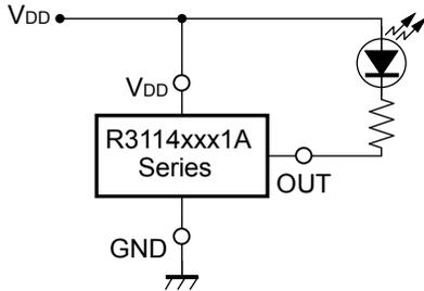
• **Detector Threshold Adjustable Circuit 1
