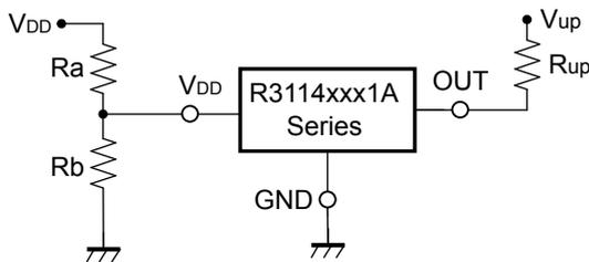
$$\text{Adjustable Detector Threshold} = (-V_{\text{DET}}) \times (R_a + R_b) / R_b$$
