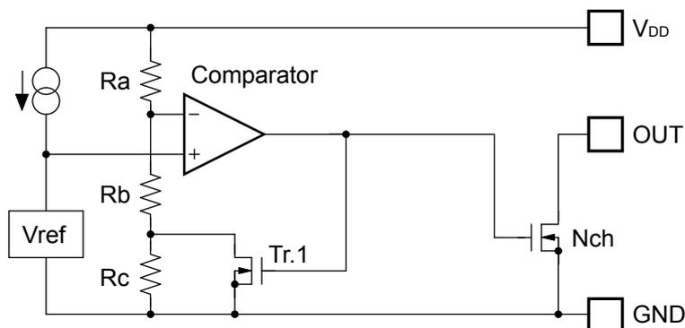
OUT pin should be pulled-up to  $V_{DD}$  or an external voltage level.
