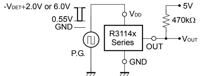
Output Delay Time Test Circuit
