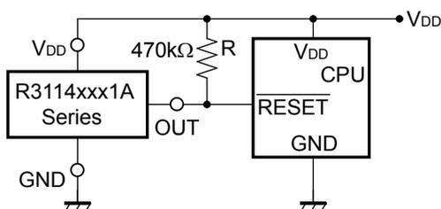
Case2. Input Voltage to R3114xxx1A is unequal to Input Voltage to CPU
