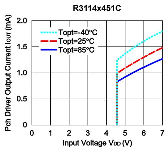
7) Pch Driver Output Current vs.  $V_{DS}$
