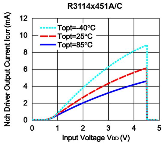
5) Nch Driver Output Current vs.  $V_{DS}$
