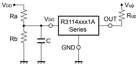
$$\text{Adjustable Detector Threshold} = (-V_{\text{DET}}) \times (R_a + R_b) / R_b$$
