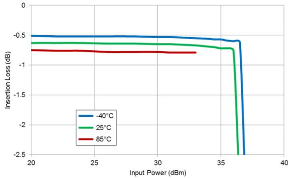
**Insertion Loss versus RF Power Over Temperature**
