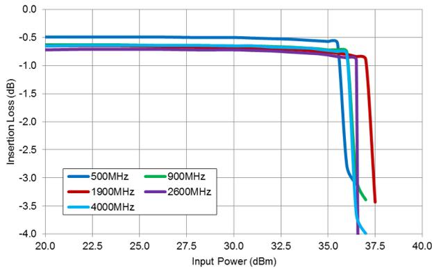
**Insertion Loss versus Input Power**
