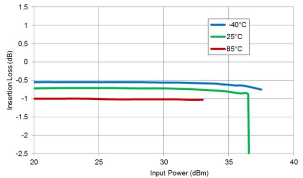
**Insertion Loss versus Input Power**
