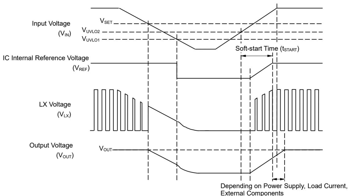
**Timing Chart with Variations in Input Voltage ( $V_{IN}$ )**
