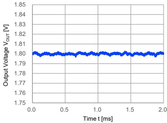
$V_{IN}=3.6V$ ,  $V_{OUT}=1.8V$ ,  $I_{OUT}=1mA$
