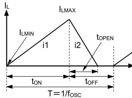
**Inductor Current ( $I_L$ ) flowing through Inductor (L)**
