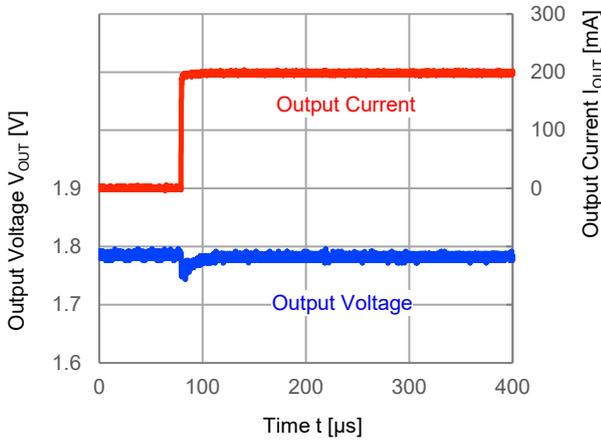
$V_{IN}=3.6V$ ,  $V_{OUT}=1.8V$ ,  $I_{OUT}=200mA \rightarrow 1mA$
