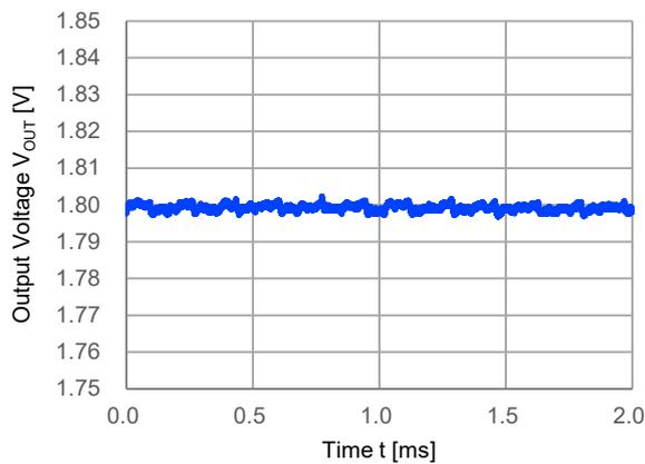
$V_{IN}=3.6V$ ,  $V_{OUT}=1.8V$ ,  $I_{OUT}=400mA$
