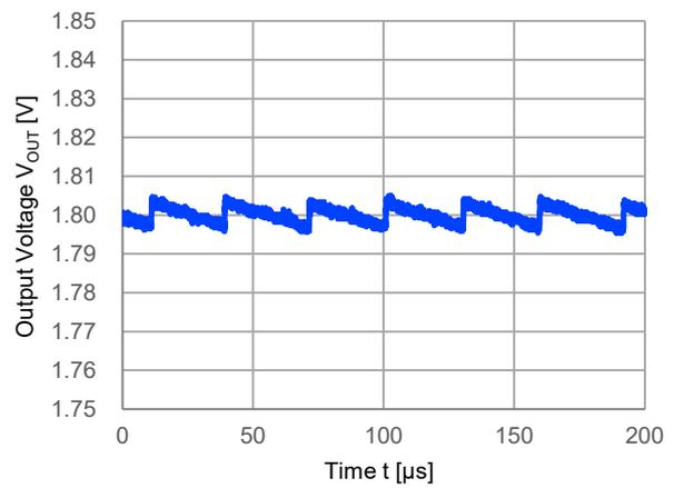
$V_{IN}=3.6V$ ,  $V_{OUT}=1.8V$ ,  $I_{OUT}=400mA$
