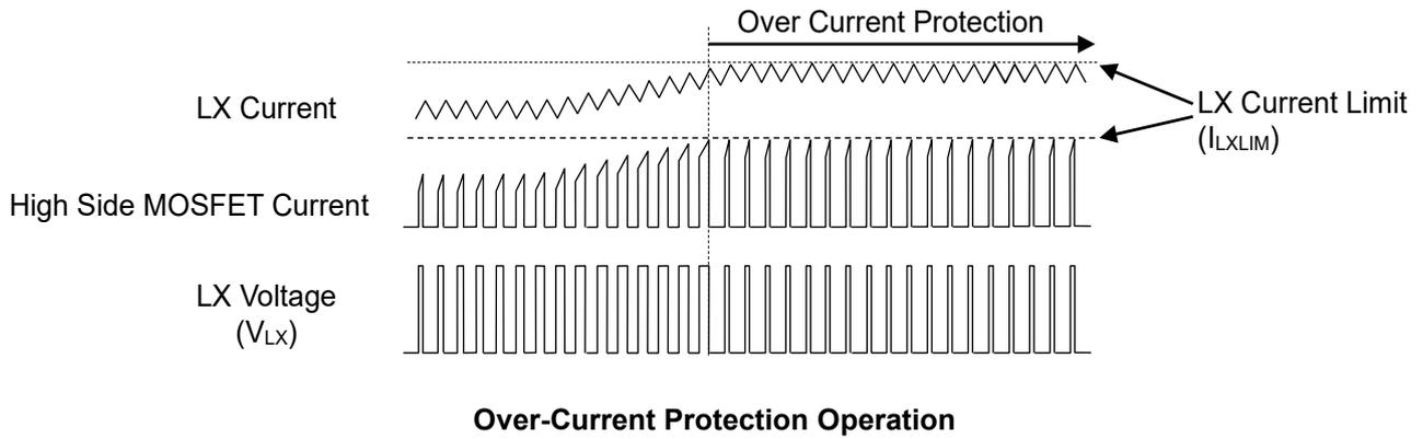
**Operation of Step-down DC/DC module and Output Current**
