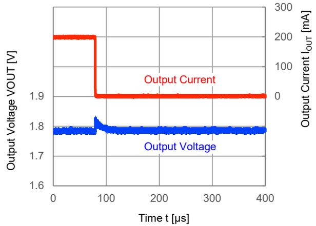
$V_{IN}=3.6V$ ,  $V_{OUT}=1.8V$ ,  $I_{OUT}=1mA \rightarrow 200mA$
