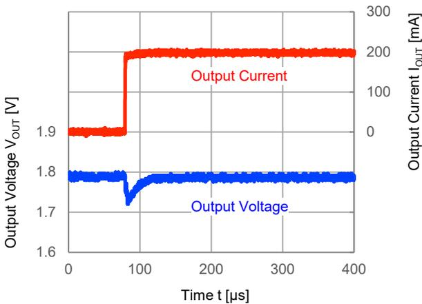
$V_{IN}=3.6V$ ,  $V_{OUT}=1.8V$ ,  $I_{OUT}=200mA \rightarrow 1mA$
