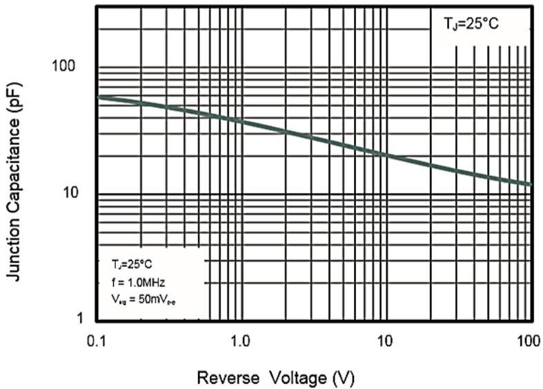
**SMD FAST RECOVERY RECTIFIER RS SERIES CASE SOD123FL**
