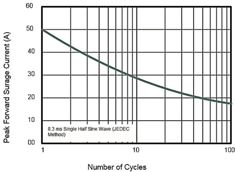
**SMD FAST RECOVERY RECTIFIER RS SERIES CASE SOD123FL**
