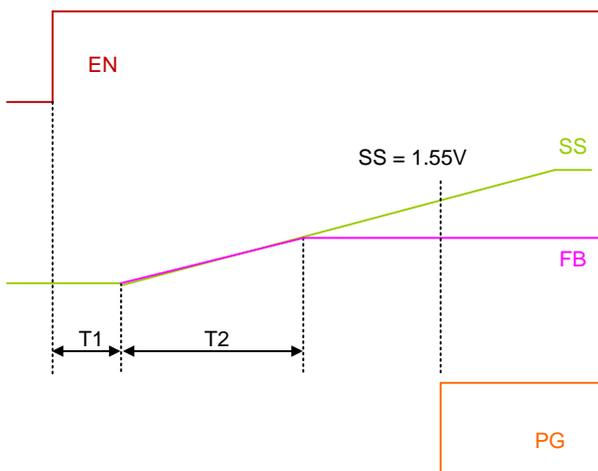
T1 : EN delay, from EN go high to SS start rising, T1 = 50μs;
