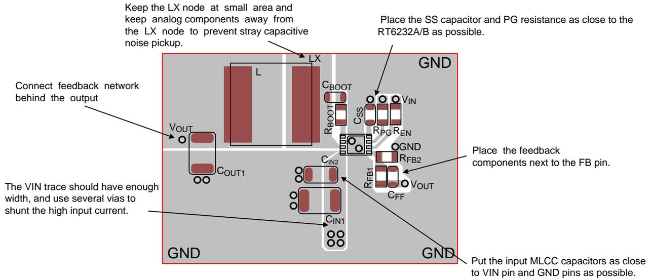
Figure 8. PCB Layout Guide
