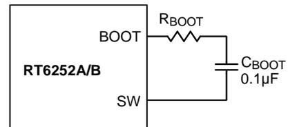
Figure 11. External Bootstrap Resistor at the BOOT Pin
