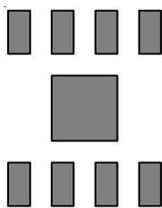
Figure 10 (a). Minimum Footprint,  $\theta_{JA} = 75^{\circ}\text{C}/\text{W}$
