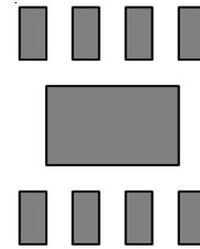
Figure 10 (b). Copper Area =  $10\text{mm}^2$ ,  $\theta_{JA} = 64^{\circ}\text{C}/\text{W}$
