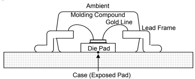
Figure 6. SOP-8 (Exposed Pad) Package Sectional Drawing
