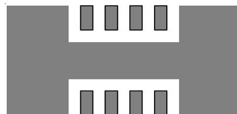
Figure 10 (e). Copper Area =  $70\text{mm}^2$ ,  $\theta_{JA} = 49^{\circ}\text{C}/\text{W}$
