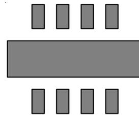
Figure 10 (c). Copper Area =  $30\text{mm}^2$ ,  $\theta_{JA} = 54^{\circ}\text{C}/\text{W}$
