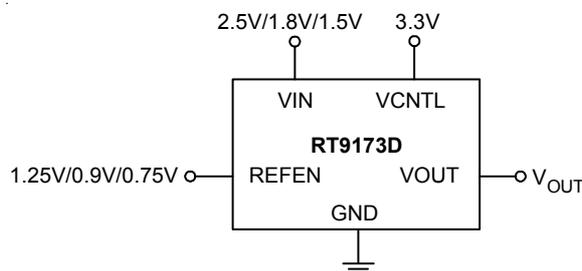
Figure 1. Test Circuit for Typical Operating Characteristics Curves
