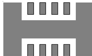
Figure 10 (d). Copper Area =  $50\text{mm}^2$ ,  $\theta_{JA} = 51^{\circ}\text{C}/\text{W}$
