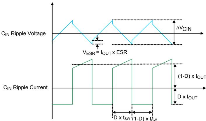
Figure 6.  $C_{IN}$  Ripple Voltage and Ripple Current
