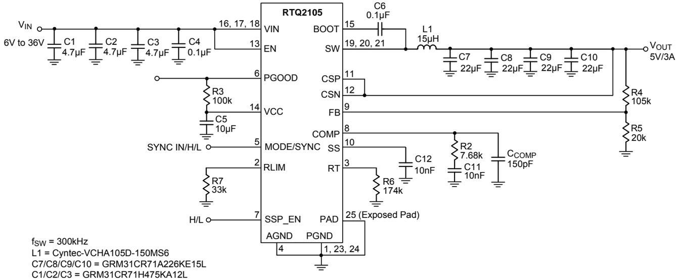
**Step-Down Circuit with Cable Drop Compensation and Average Current Limit ( for  $V_{OUT} = 5V$  only)**
