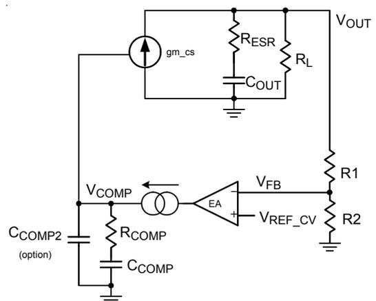
Figure 9. Simplified Equivalent Circuit of Buck with PCMC
