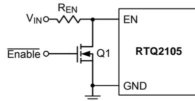
Figure 15. Logic Control for the EN Pin
