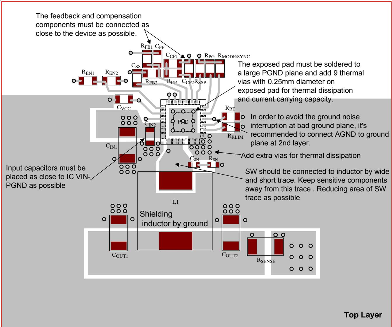
Figure 19. Layout Guide (Top Layer)
