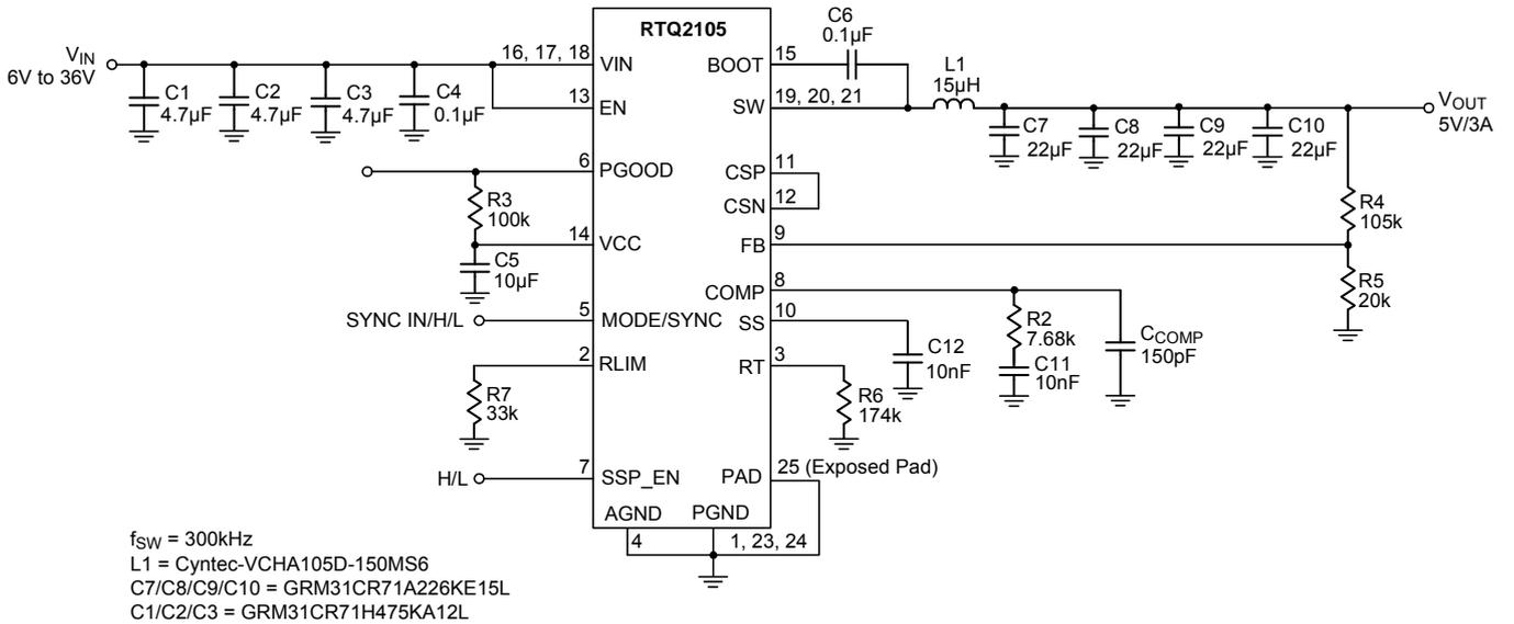
**300kHz, 3.3V, 3A Step-Down Converter**
