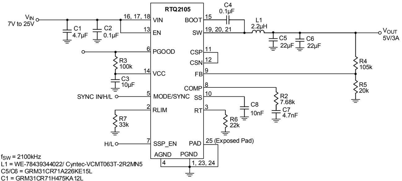
**Step-Down Circuit with Switch-Over Function (for  $V_{OUT}$  regulated within 4.8V to 6V only)**
