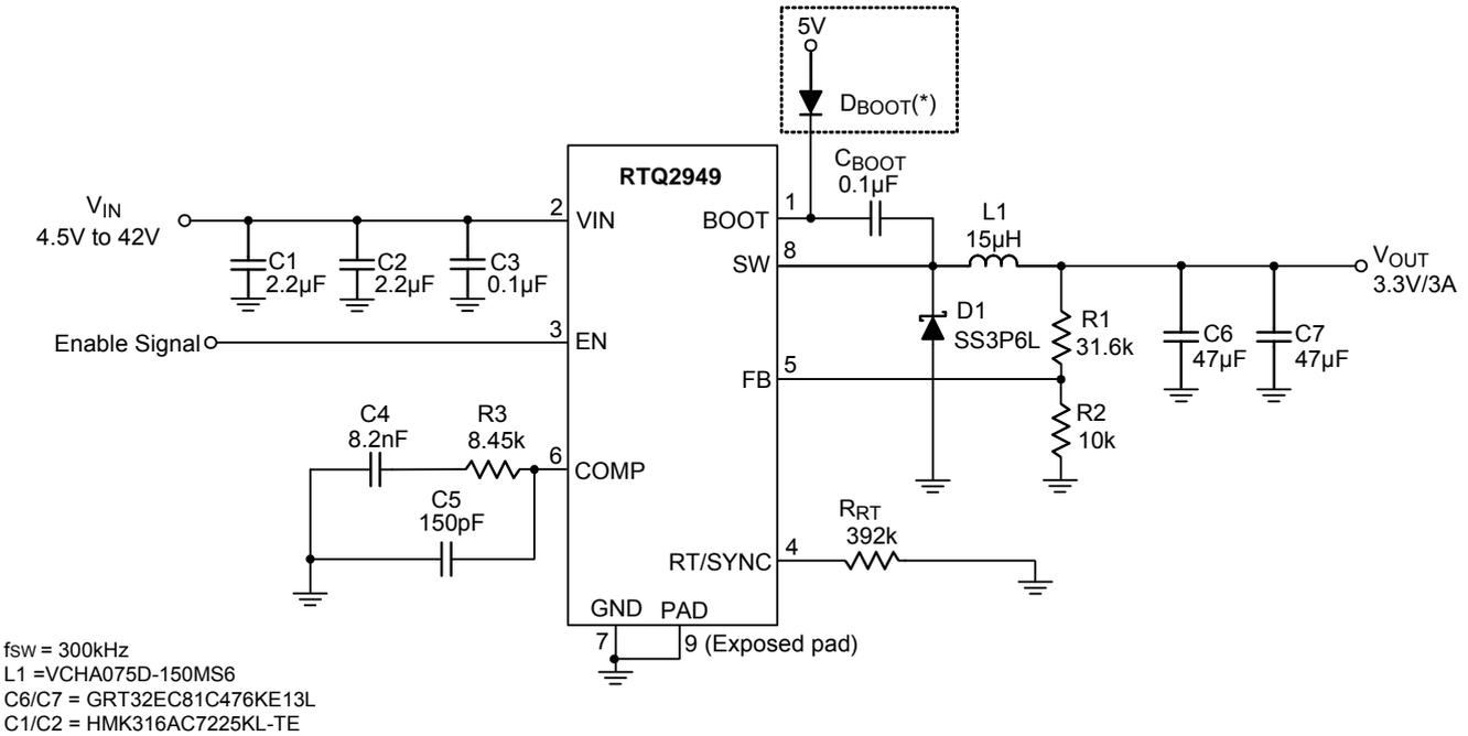
**500kHz, 5V, 3A Step-Down Converter**
