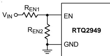
Figure 12. Resistive Divider for Under-Voltage Lockout Threshold Setting
