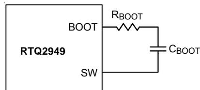
Figure 10. External Bootstrap Resistor at the BOOT Pin
