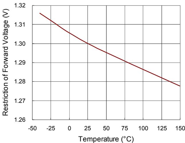
Figure 5. Restriction of Forward Voltage vs. Temperature
