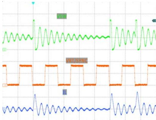
Figure 13. Synchronization Mode in PSM
