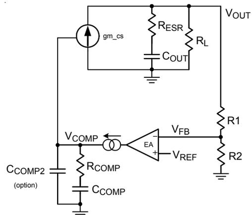
Figure 8. Simplified Equivalent Circuit of Buck with PCMC
