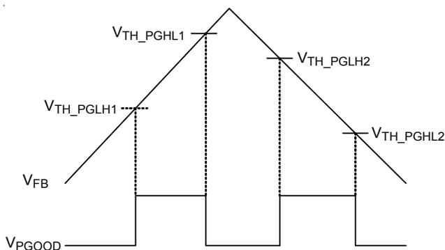
Figure 2. The Logic of PGOOD for RTQ2965GQW
