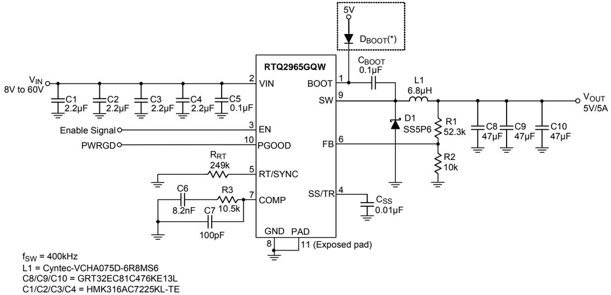
**400kHz, 12V, 5A Step-Down Converter**
