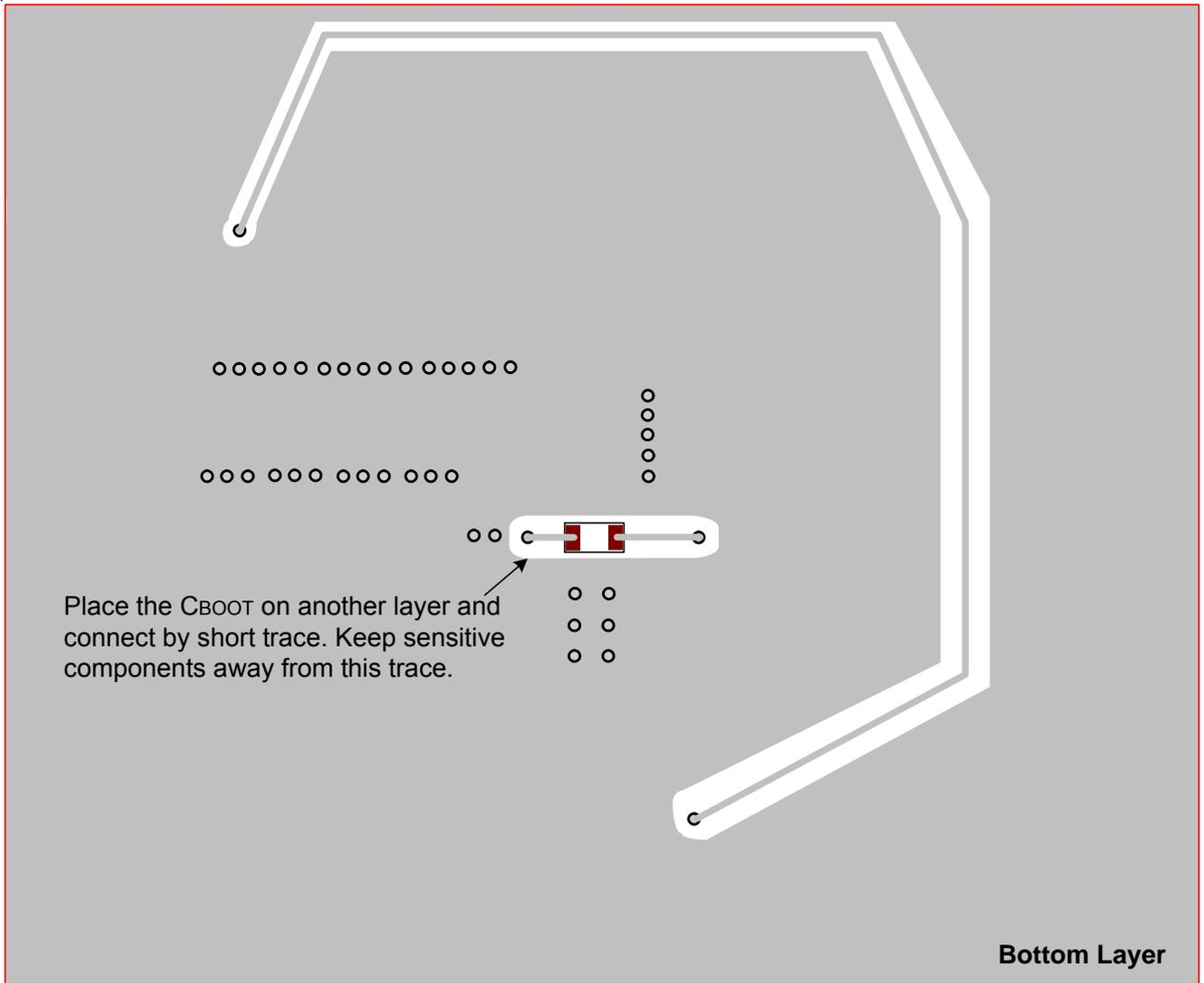
Figure 18. Layout Guide for RTQ2965GQW (Bottom Layer)
