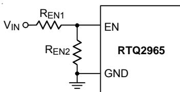
Figure 14. Resistive Divider for Under-Voltage Lockout Threshold Setting
