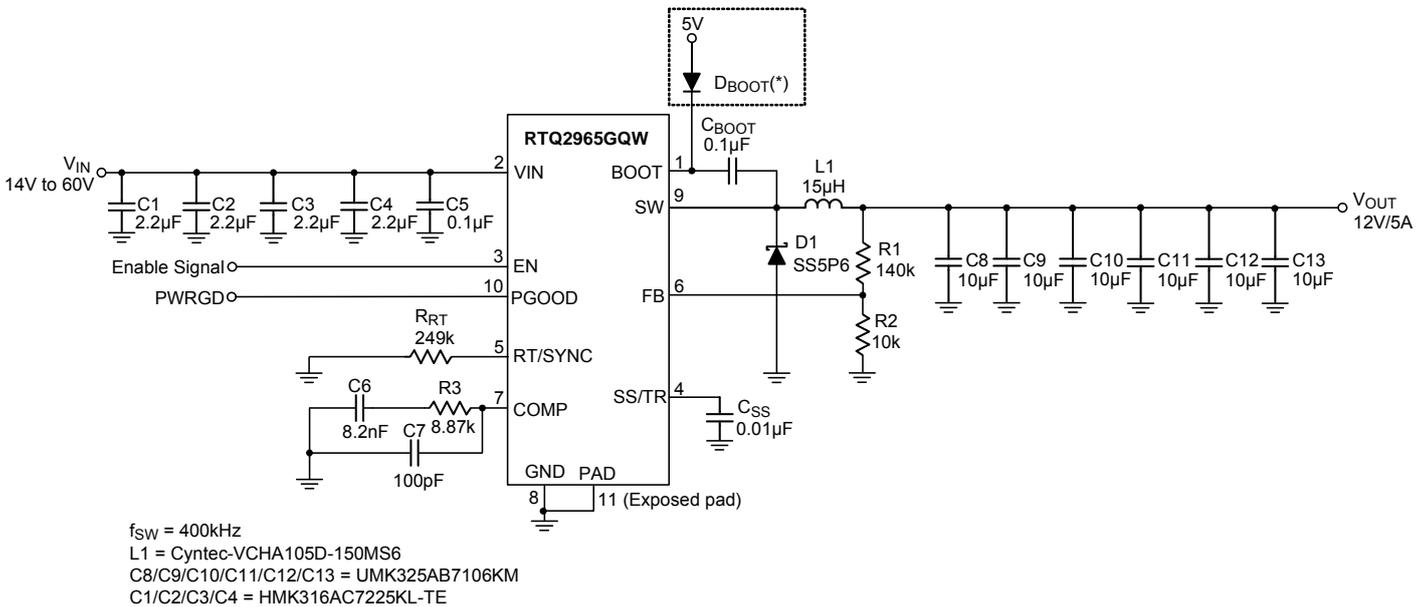
\* : While the input voltage is below 5.5V or duty ratio is higher than 65%, an external bootstrap diode must be added between an external 5V voltage supply and the BOOT pin to enhance the drive capability for the high-side MOSFET. Refer to the Application Information for more details on the external bootstrap diode design.
