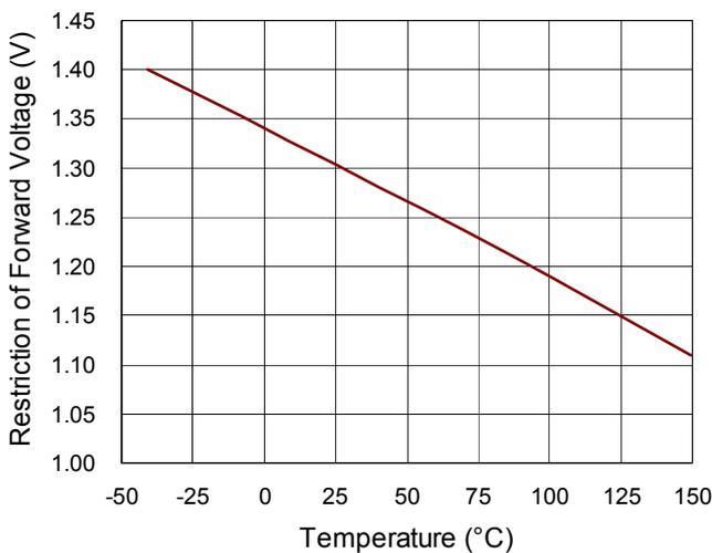
Figure 6. Restriction of Forward Voltage vs. Temperature
