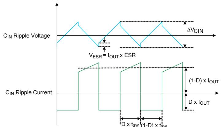
Figure 5.  $C_{IN}$  Ripple Voltage and Ripple Current
