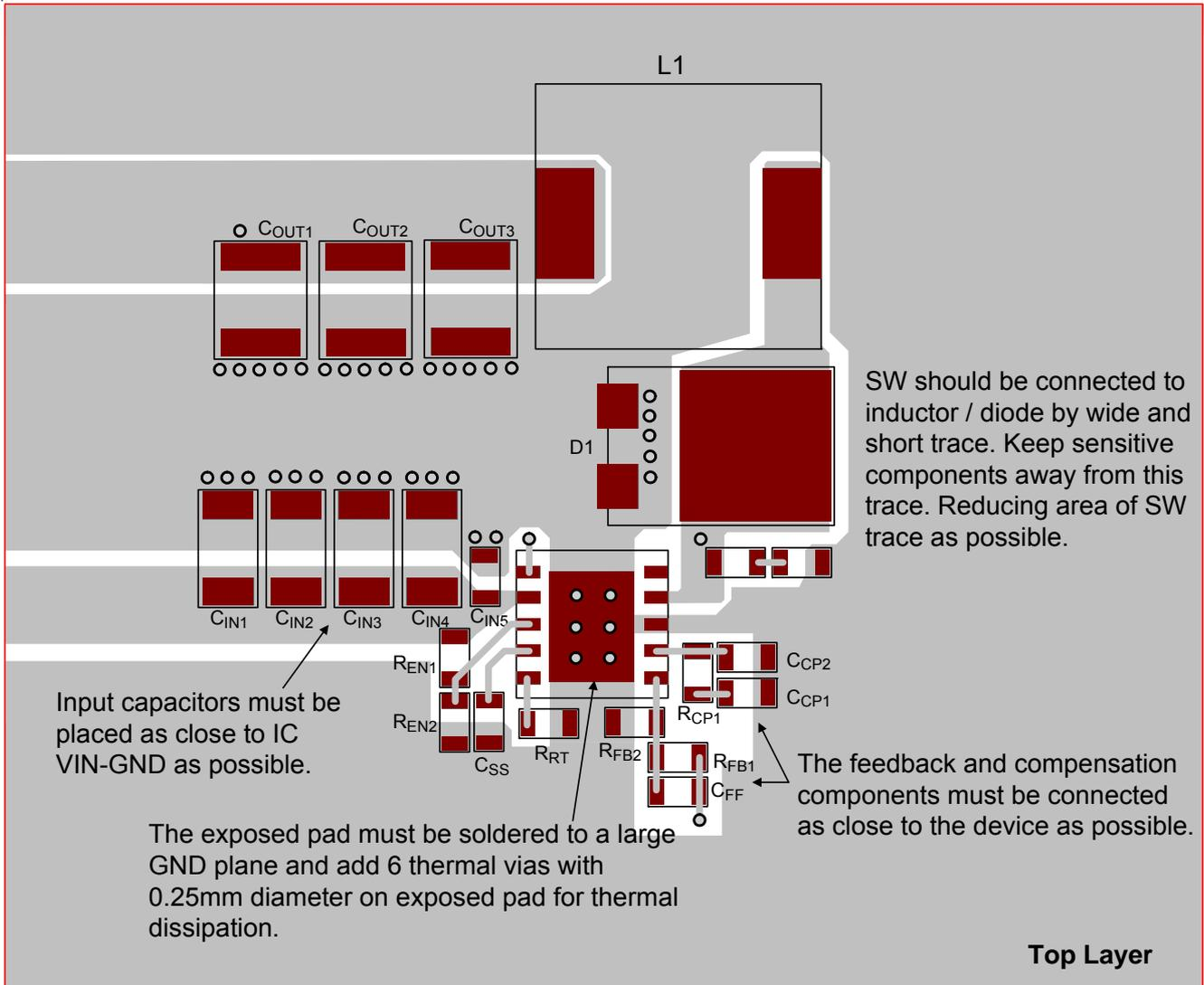
Figure 17. Layout Guide for RTQ2965GQW (Top Layer)
