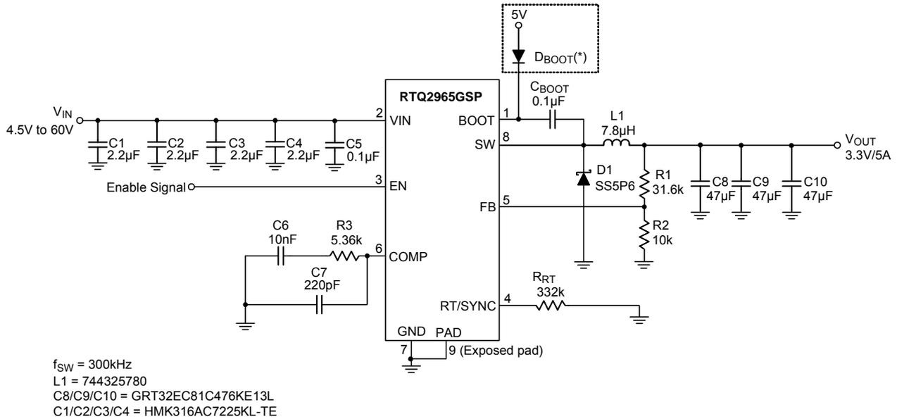
**400kHz, 5V, 5A Step-Down Converter**
