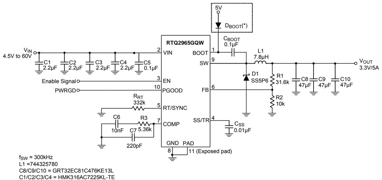
**400kHz, 5V, 5A Step-Down Converter**
