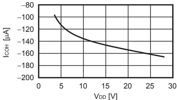
**4.2  $I_{COH}$  vs.  $V_{DD}$  (S-8223B/D Series)**
