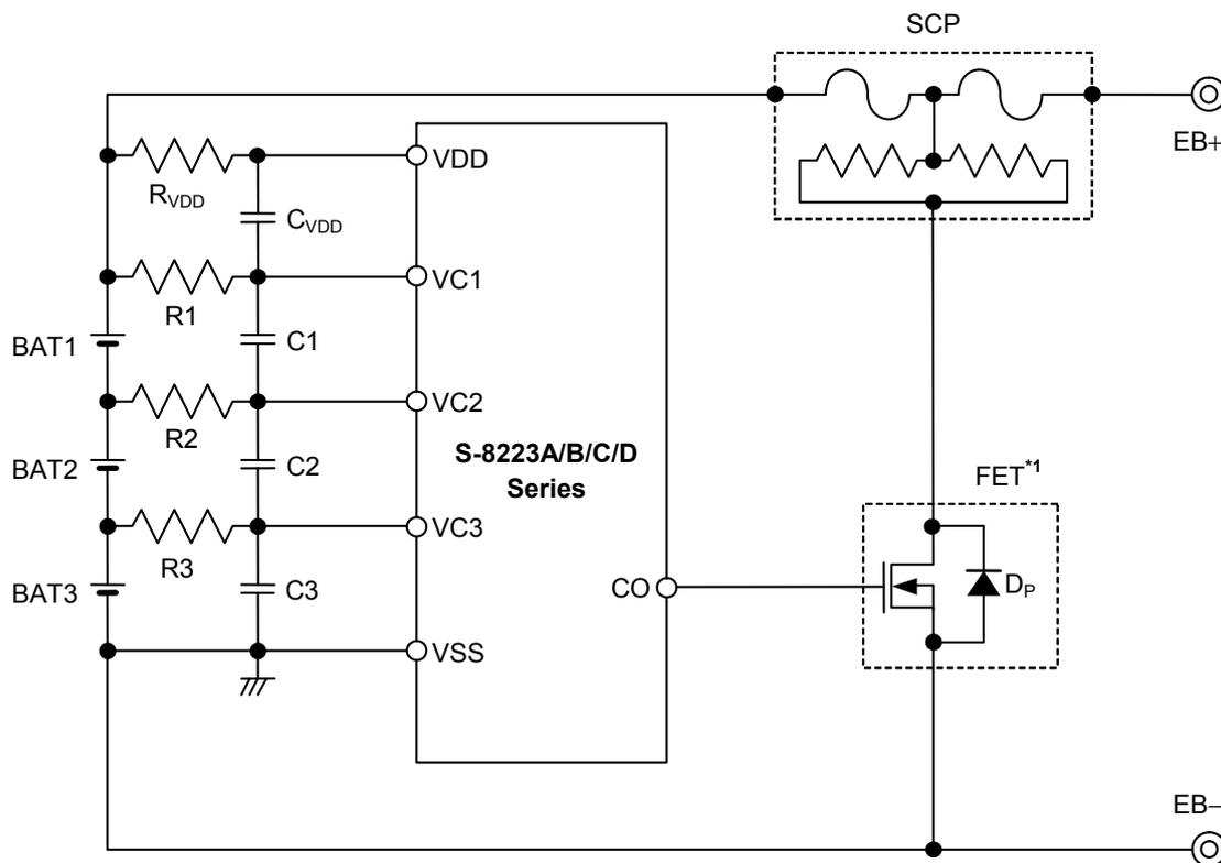
\*1. The S-8223B/D Series limits its CO pin output voltage to 11.5 V max., so a FET with the gate withstand voltage of 12 V can be used.
