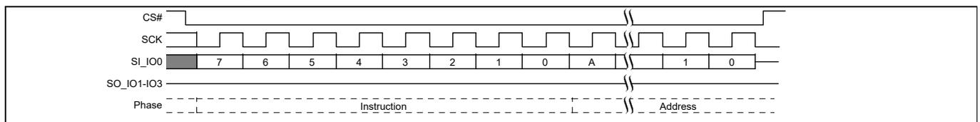
**Figure 89** Sector Erase (SE D8h or 4SE DCh) command sequence<sup>[56]</sup>
