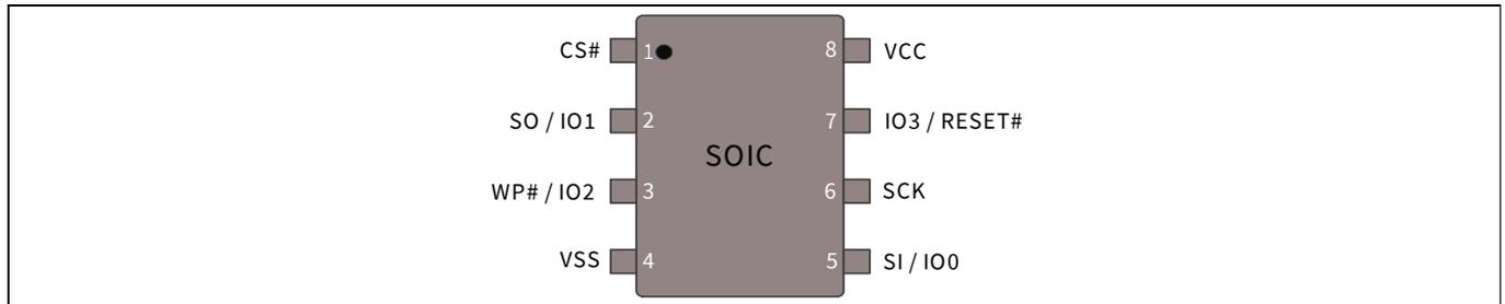
**Figure 1** 8-pin plastic small outline package (SOIC8)
