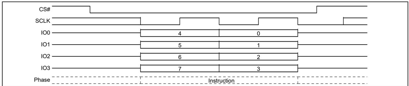
**Figure 56 Write Enable (WREN) command sequence QPI mode**
