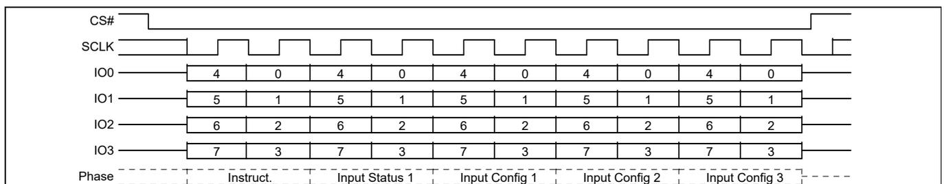
Figure 54 Write Register (WRR) command sequence QPI
