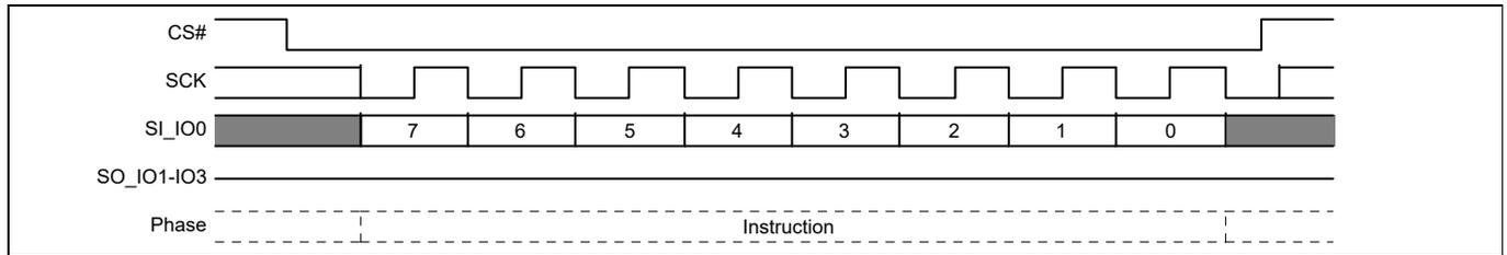
**Figure 59 Clear Status Register (CLSR) command sequence**
