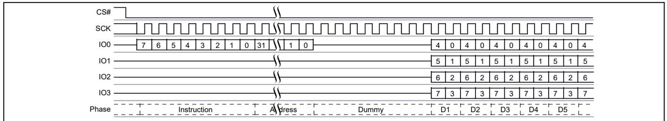
Figure 15 Quad Output Read command
