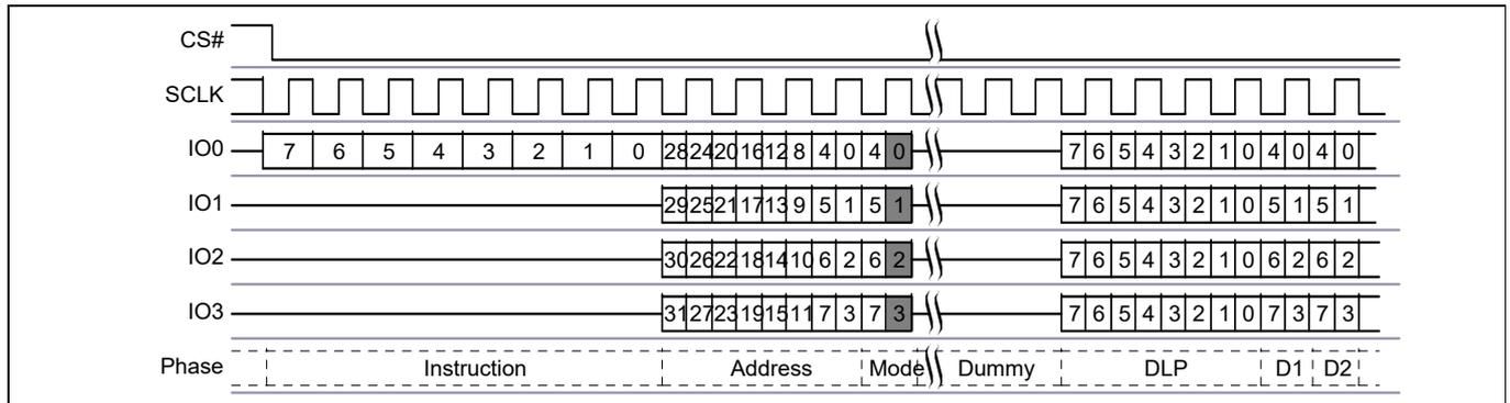
**Figure 19** DDR Quad I/O Read command<sup>[7]</sup>
