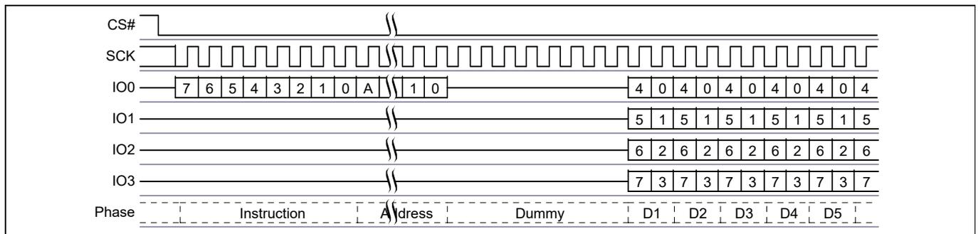
**Figure 75** Quad Output Read command sequence<sup>[45]</sup>
