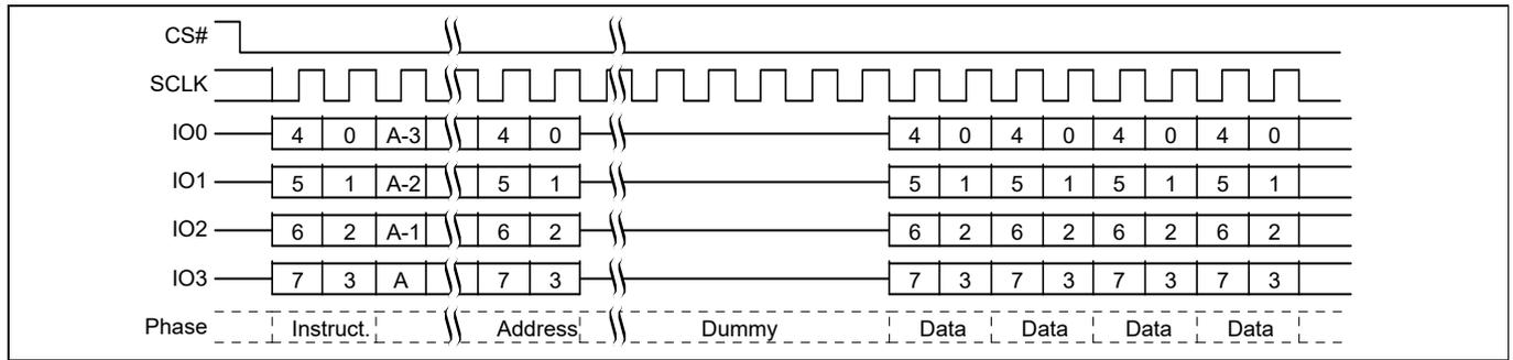
Figure 62 ECC Status Register Read QPI mode, command sequence [39, 40]
