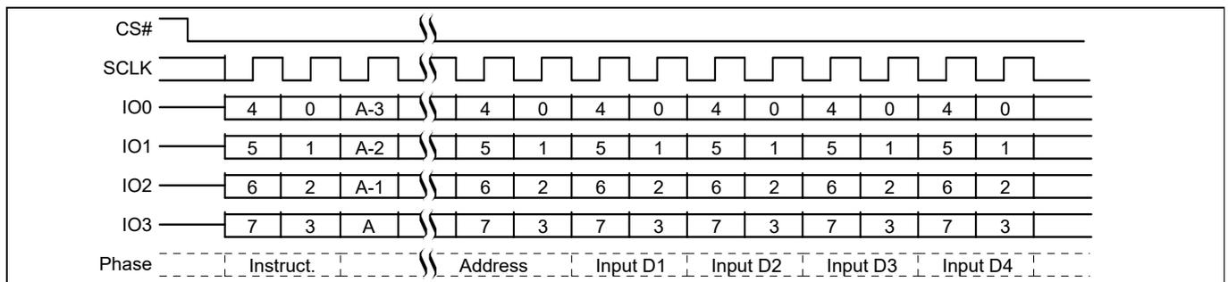
**Figure 105** DYB Write QPI mode command sequence<sup>[61, 62]</sup>
