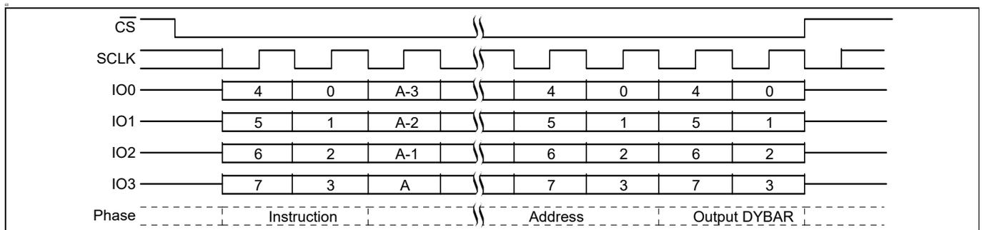
Figure 103 DYBRD QPI mode command sequence<sup>[58, 60]</sup>
