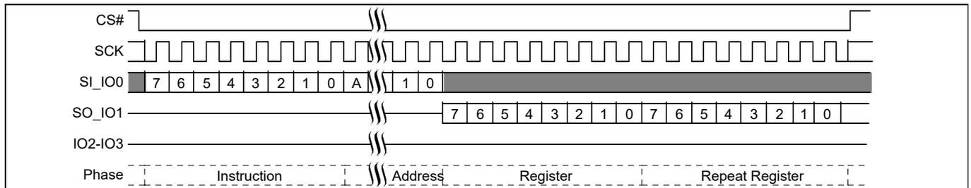
Figure 102 DYBRD command sequence<sup>[58, 59]</sup>
