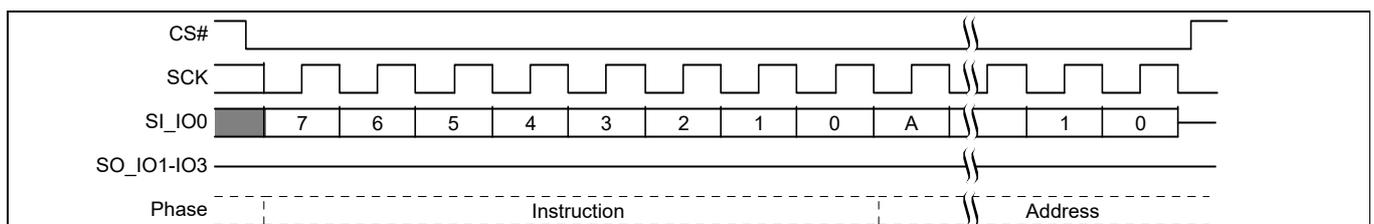
**Figure 87** Parameter Sector Erase (P4E 20h or 4P4E 21h) command sequence<sup>[55]</sup>
