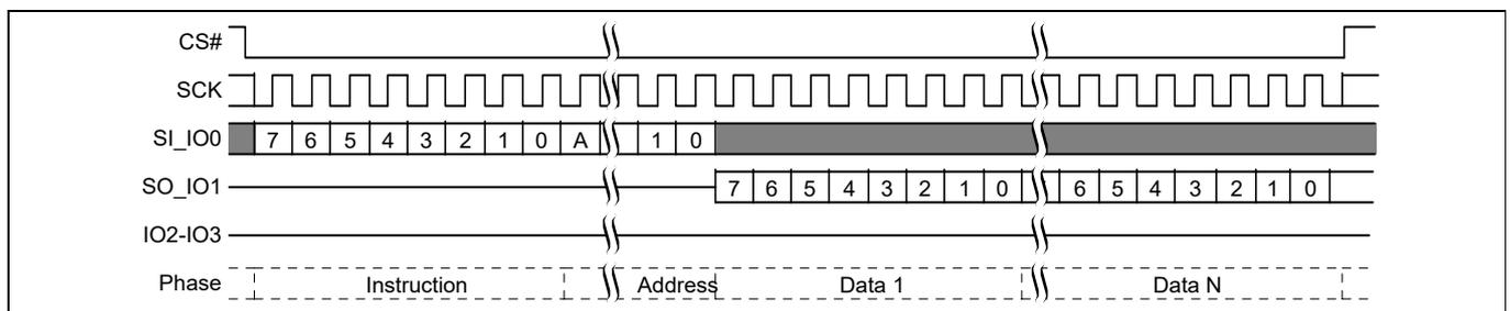
**Figure 72** Read command sequence<sup>[42]</sup>
