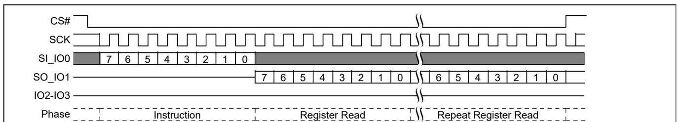
**Figure 52 Read Configuration Register (RDCR) command sequence**
