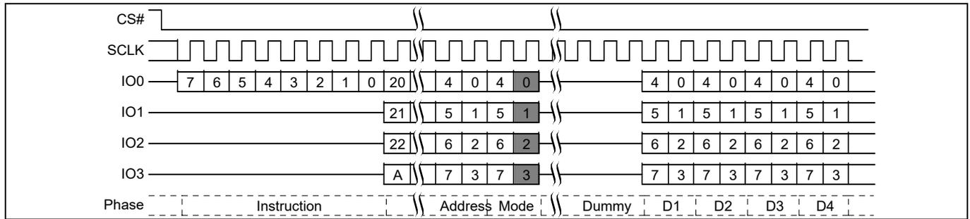
Figure 78 Quad I/O Read Initial Access command sequence<sup>[48]</sup>
