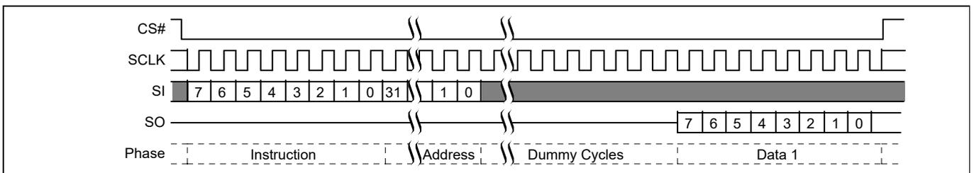
Figure 13 Single Bit Wide I/O command with latency
