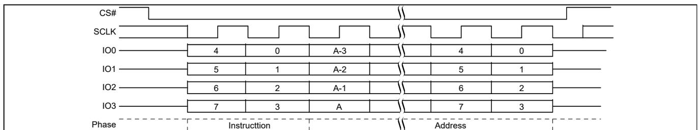
**Figure 88** Parameter Sector Erase (P4E 20h or 4P4E 21h) QPI mode command sequence<sup>[55]</sup>
