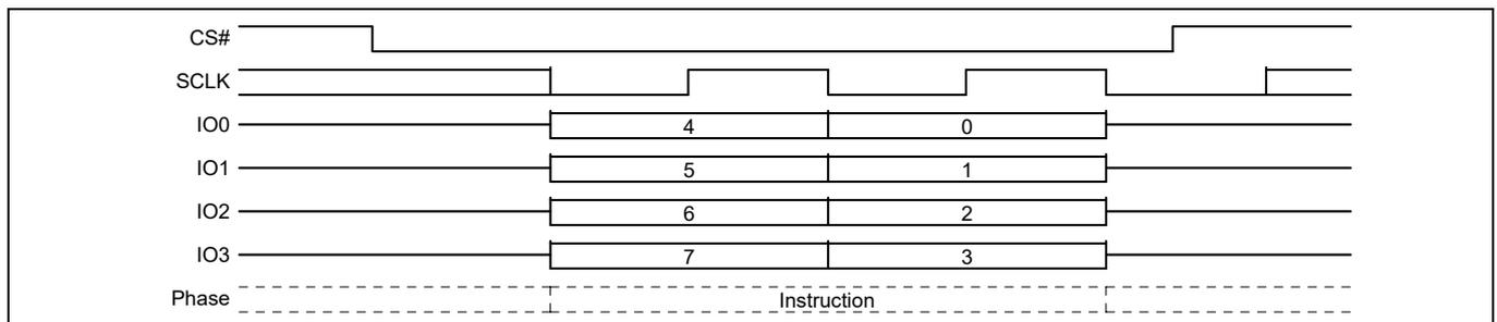
**Figure 119 Release from Deep Power Down (RES) command sequence – QPI mode**
