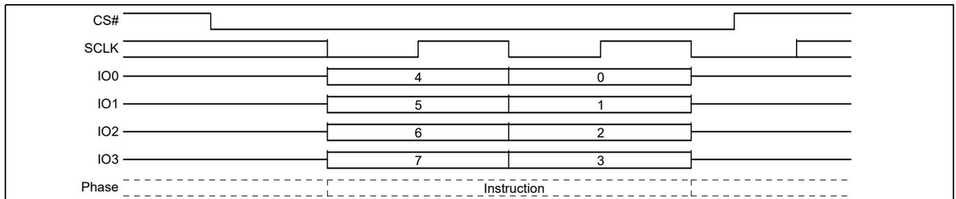
**Figure 92 Bulk Erase Command sequence QPI mode**
