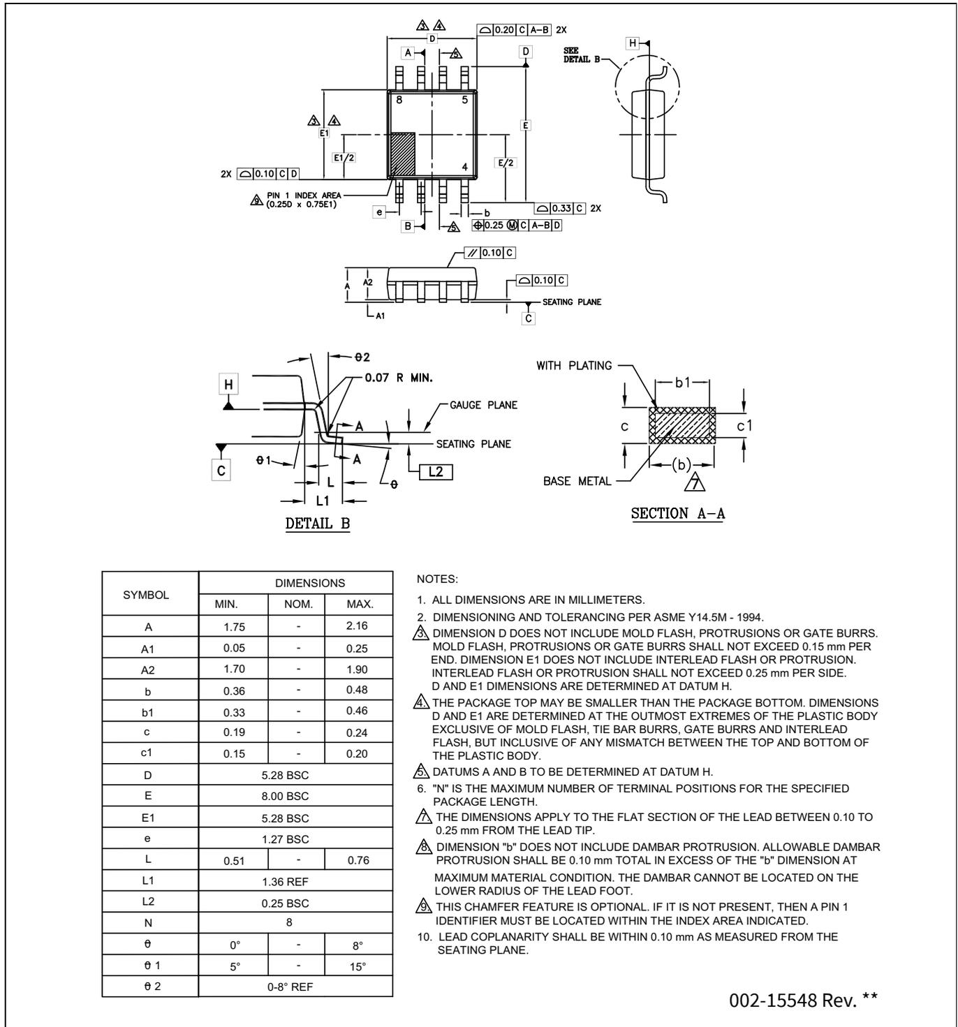
Figure 124 8-lead SOIC (5.28 × 5.28 × 2.16 mm) SOC008 package outline, 002-15548
