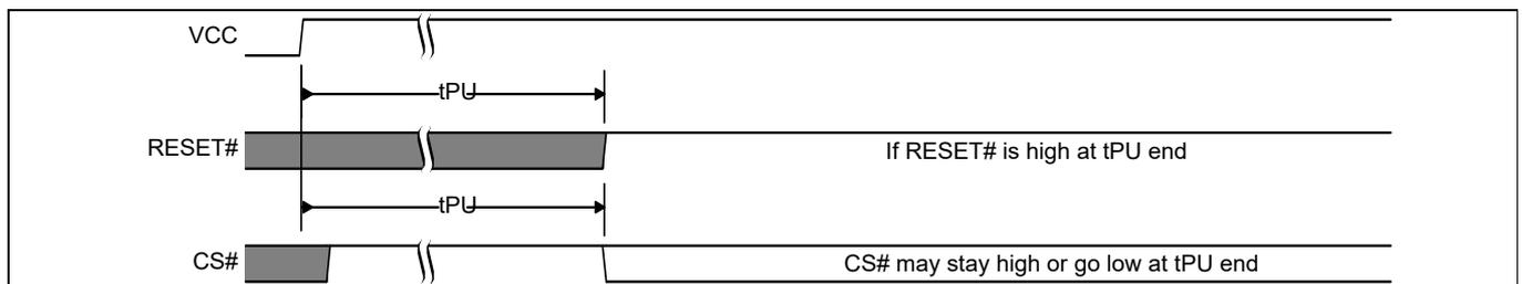
**Figure 25** Reset high at the end of POR
