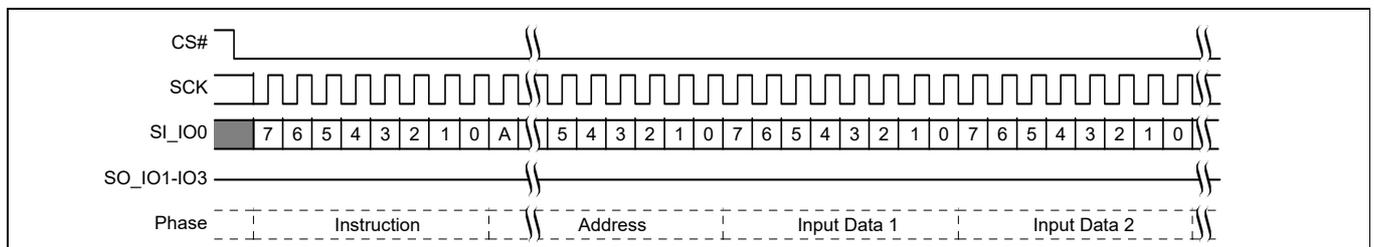
**Figure 104** DYB Write command sequence<sup>[61, 62]</sup>
