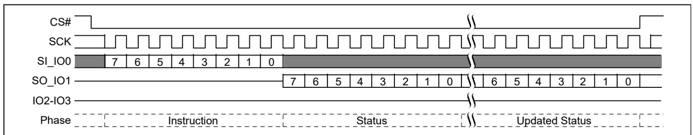
**Figure 49 Read Status Register-1 (RDSR1) command sequence**
