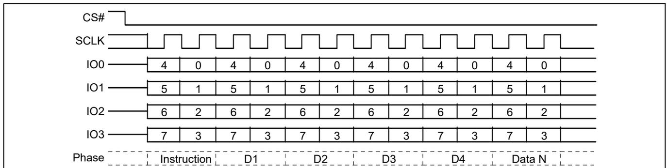
**Figure 42** Read Identification (RDID) QPI mode command
