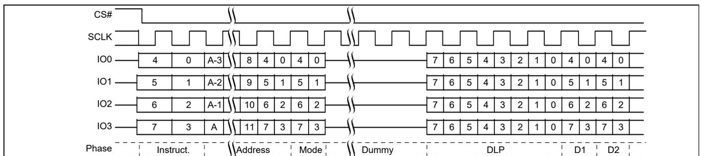
**Figure 82** DDR Quad I/O Read initial access QPI mode<sup>[50, 51]</sup>
