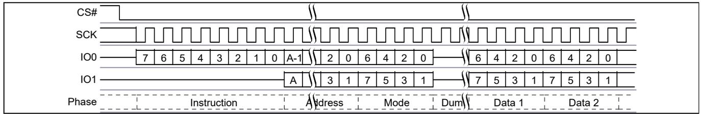
Figure 76 Dual I/O Read command sequence<sup>[46, 47]</sup>
