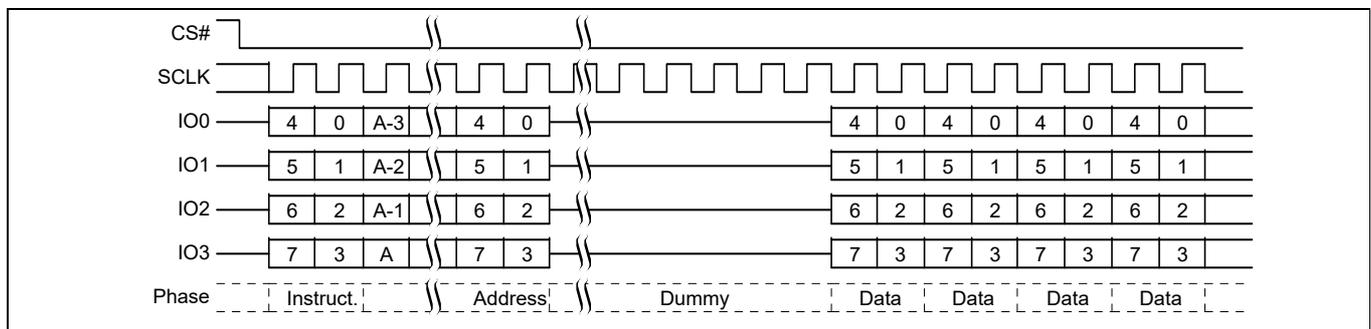
**Figure 69 Read Any Register, QPI mode, command sequence**<sup>[41]</sup>
