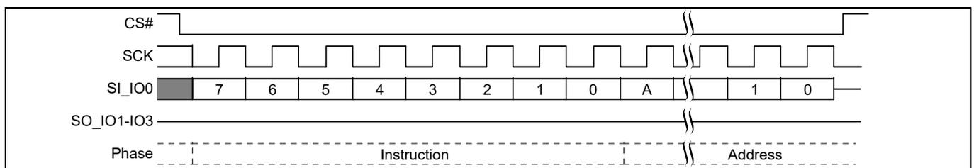
Figure 107 PPB command sequence<sup>[65, 66]</sup>
