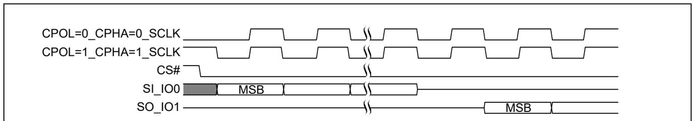
**Figure 8 SPI SDR modes supported**
