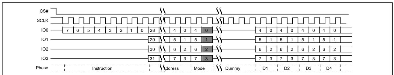
Figure 17 Quad I/O command<sup>[6]</sup>
