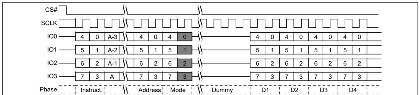
Figure 79 Quad I/O Read Initial Access command sequence QPI mode<sup>[48]</sup>
