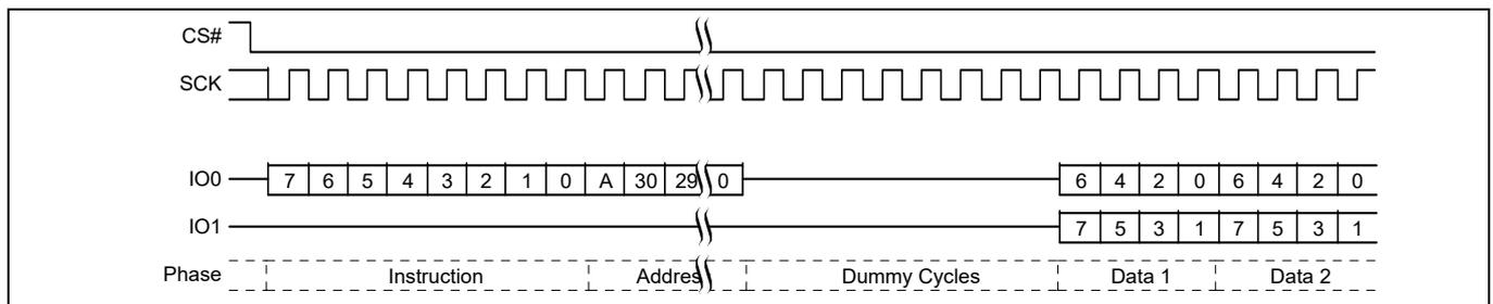
**Figure 74** Dual Output Read command sequence<sup>[44]</sup>
