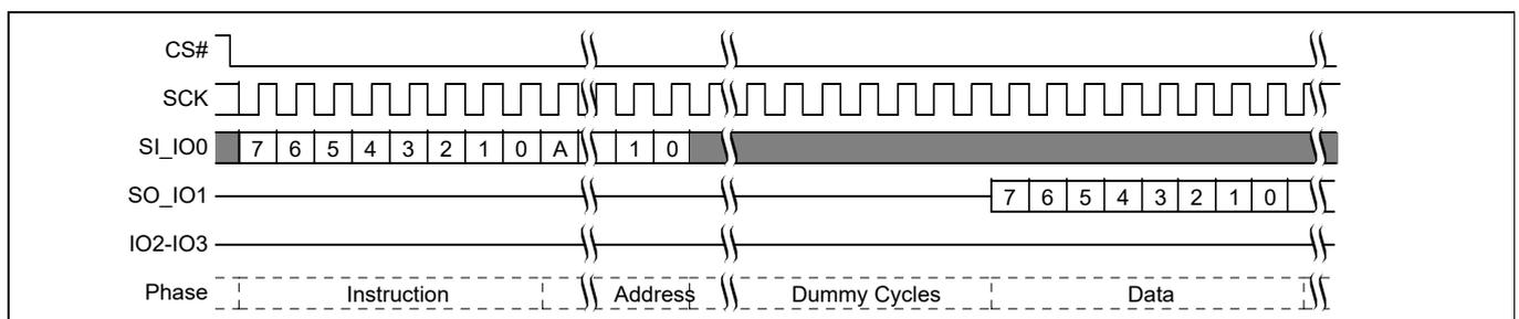
**Figure 61 ECC Status Register Read command sequence** <sup>[37, 38]</sup>
