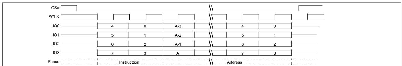
**Figure 90** Sector Erase (SE D8h or 4SE DCh) QPI mode command sequence<sup>[56]</sup>
