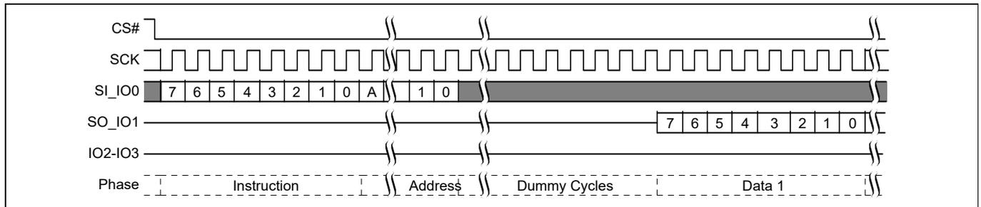
**Figure 73** Fast Read (FAST\_READ) command sequence<sup>[43]</sup>
