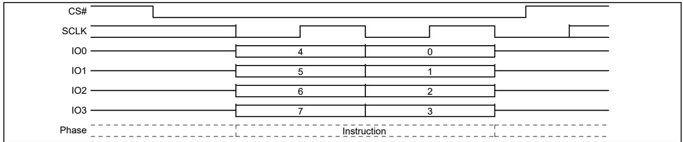
**Figure 67 Enter 4 Byte Address QPI mode**
