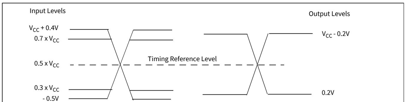
Figure 23 Input, output, and timing reference levels
