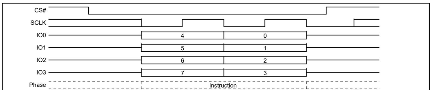
**Figure 115 Software reset/mode bit command sequence – QPI mode**
