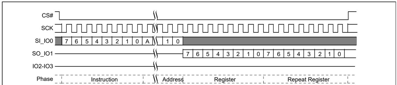
Figure 106 PPB Read command sequence<sup>[63, 64]</sup>
