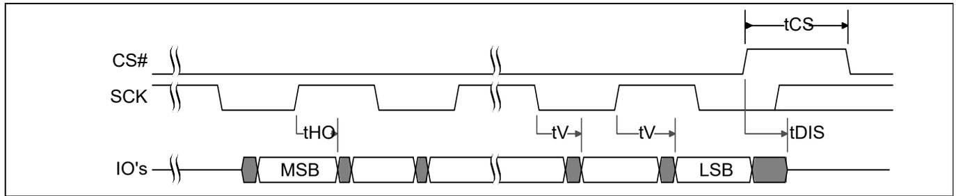
Figure 36 SPI DDR output timing
