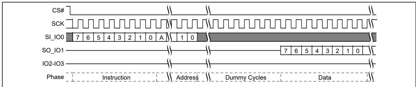
**Figure 68 Read Any Register Read command sequence**<sup>[41]</sup>
