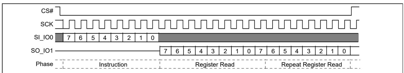
**Figure 109 PPB Lock Register command sequence**
