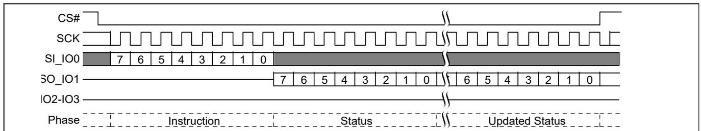
**Figure 51 Read Status Register-2 (RDSR2) command**
