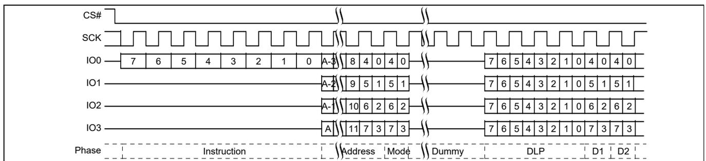
**Figure 81** DDR Quad I/O Read initial access<sup>[50, 51]</sup>
