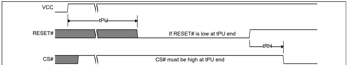
**Figure 24** Reset low at the end of POR
