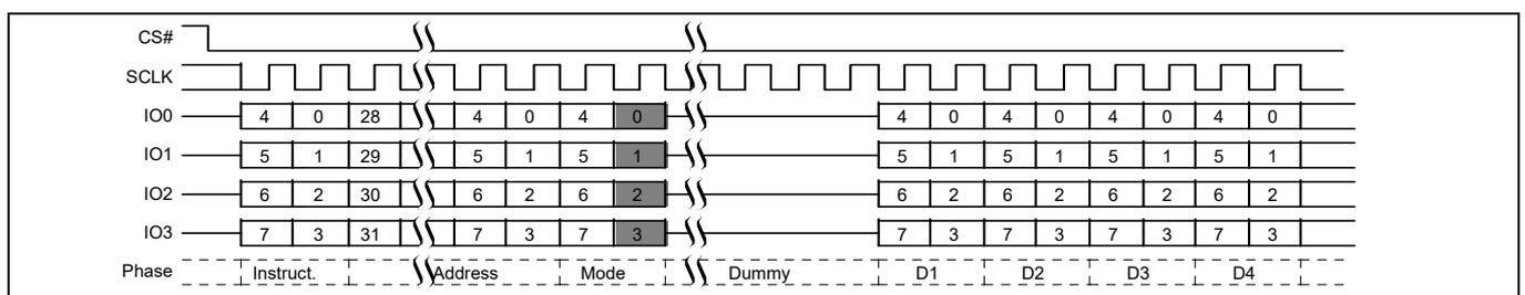
Figure 18 Quad I/O Read command in QPI mode<sup>[6]</sup>
