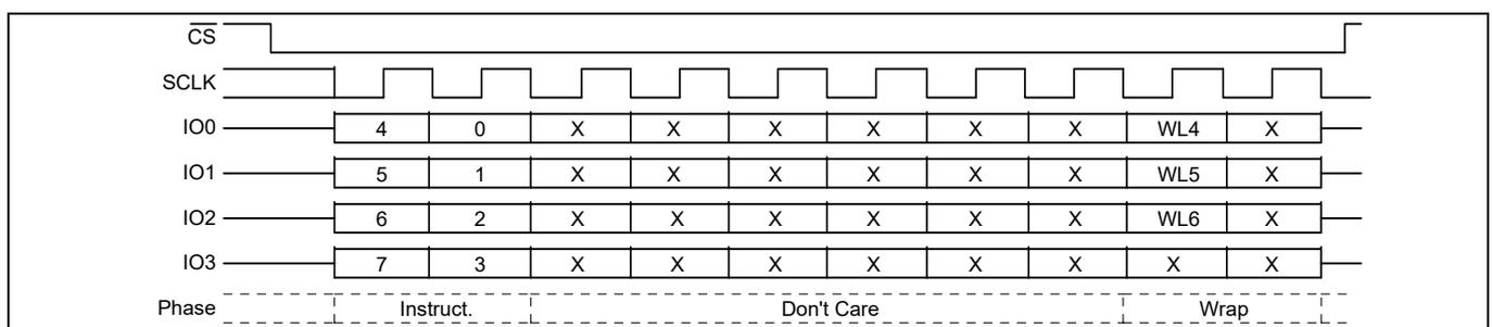
**Figure 71 Set Burst Length command sequence QPI mode**
