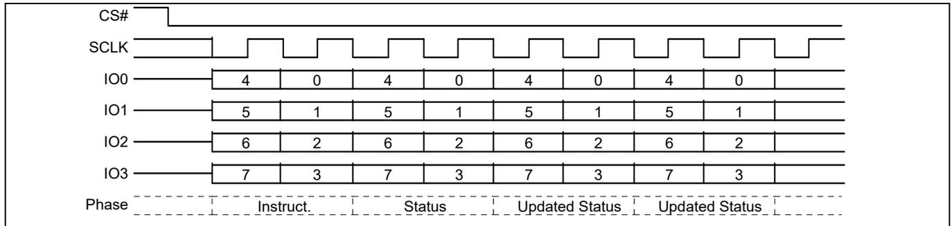
**Figure 50 Read Status Register-1 (RDSR1) QPI mode command**
