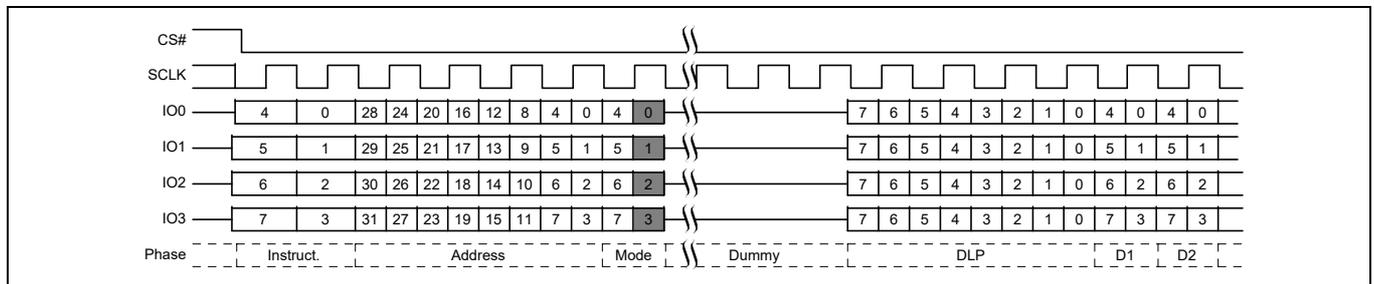
**Figure 20** DDR Quad I/O Read command QPI mode<sup>[7]</sup>
