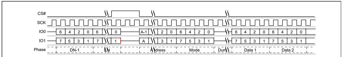
Figure 77 Dual I/O Continuous Read command sequence<sup>[46, 47]</sup>
