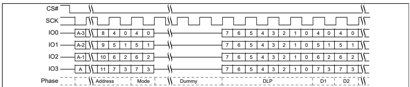
**Figure 83** Continuous DDR Quad I/O Read subsequent access<sup>[50, 51, 52]</sup>
