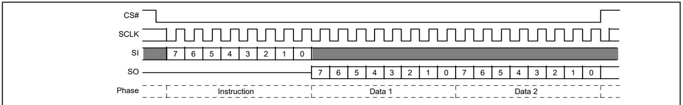
Figure 12 Single Bit Wide Output command without latency
