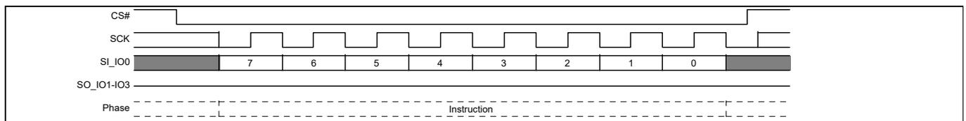
Figure 116 Deep Power Down (DPD) command sequence
