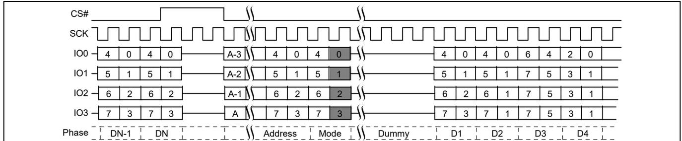
Figure 80 Continuous Quad I/O Read command sequence<sup>[48, 49]</sup>
