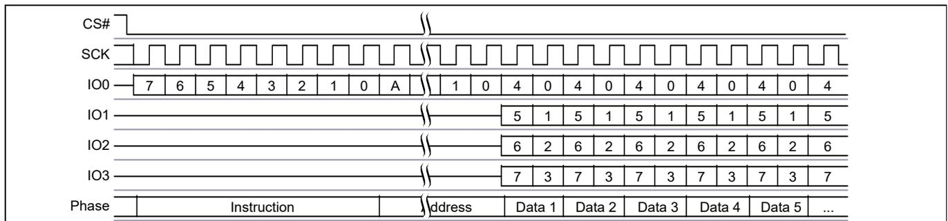
**Figure 86** Quad Page Program command sequence<sup>[54]</sup>
