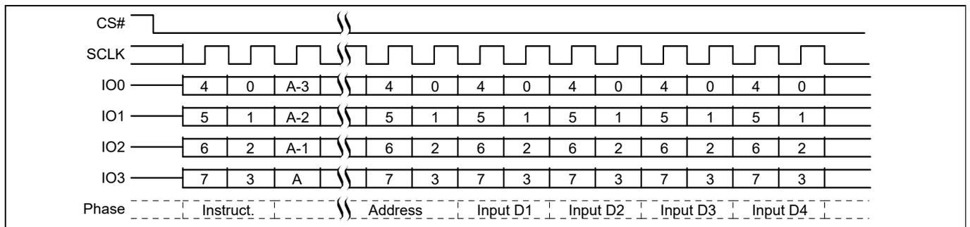
**Figure 85 Page Program (PP 02h or 4PP 12h) QPI mode command sequence<sup>[53]</sup>**
