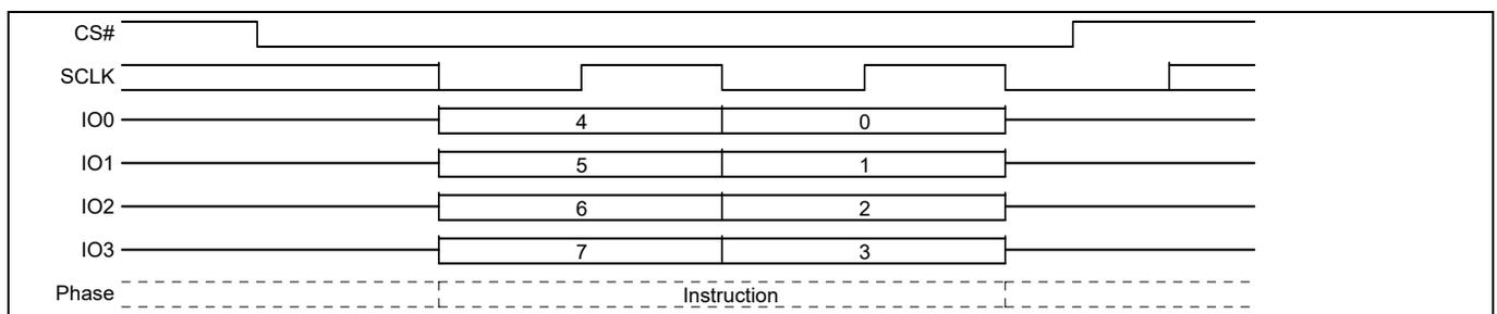
**Figure 58 Write Disable (WRDI) command sequence QPI mode**
