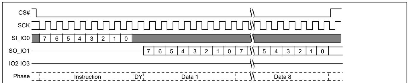
**Figure 111 Password Read (PASSRD) command sequence**
