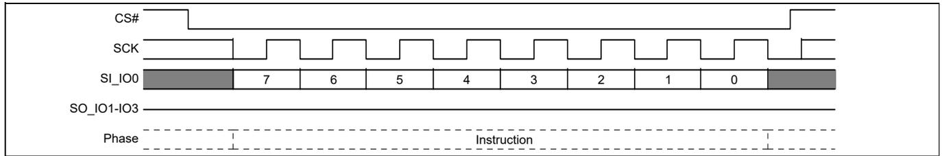
**Figure 95 Program or Erase Suspend command sequence**
