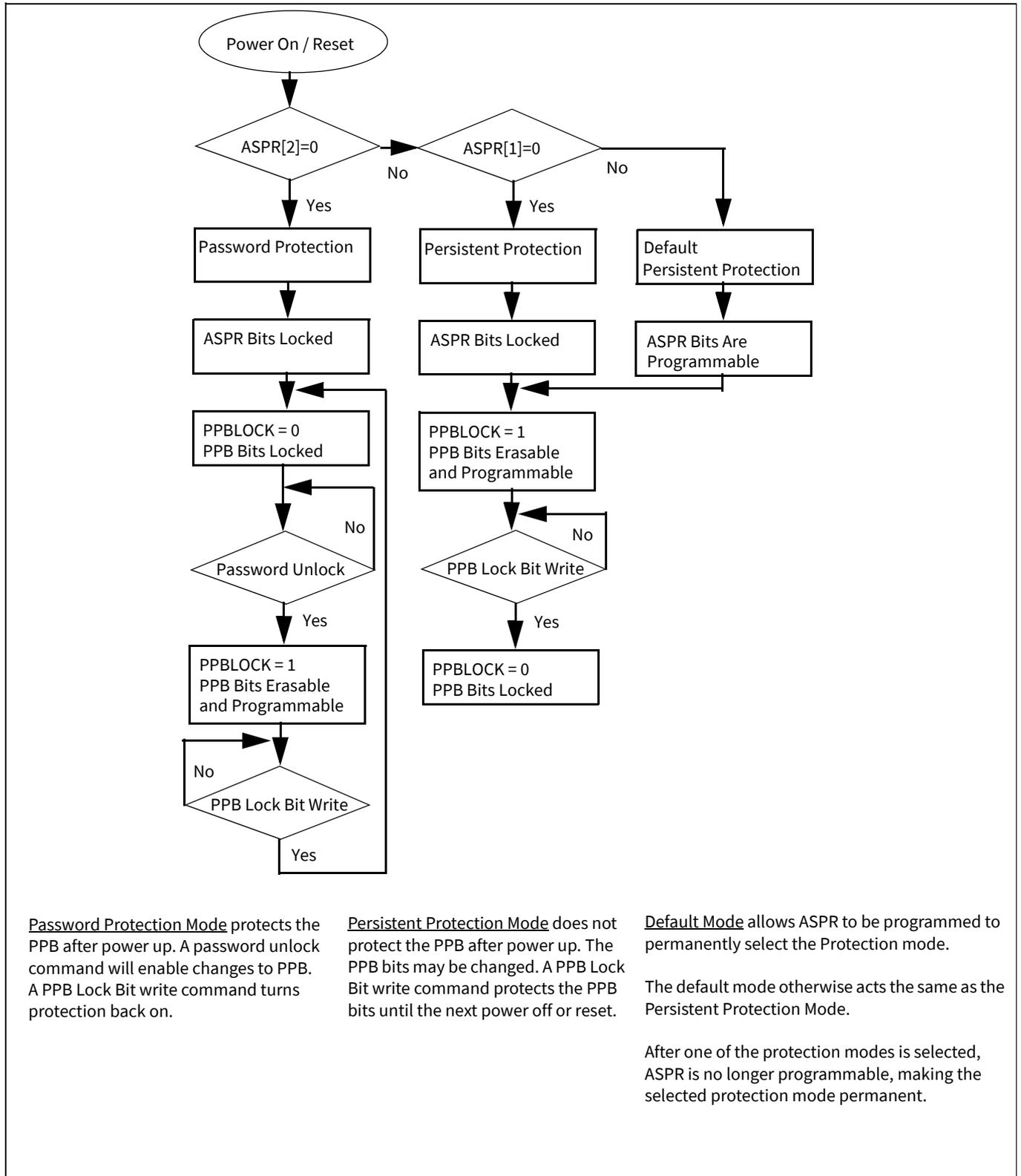
Password Protection Mode protects the PPB after power up. A password unlock command will enable changes to PPB. A PPB Lock Bit write command turns protection back on.
