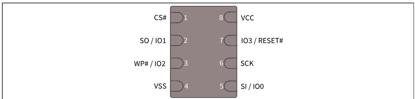
**Figure 2** 8-pad LGA 5 × 6 (W9A008), top view<sup>[4]</sup>
