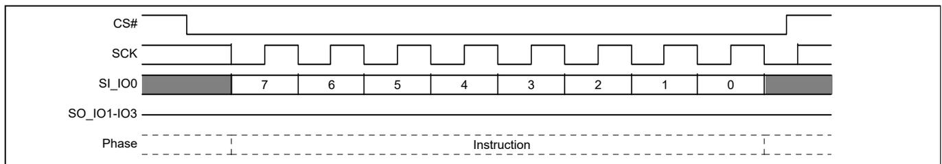
**Figure 114 Software/mode bit reset command sequence**
