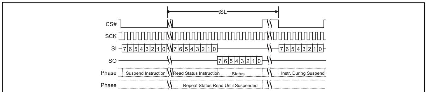
**Figure 88** Program or Erase Suspend command sequence
