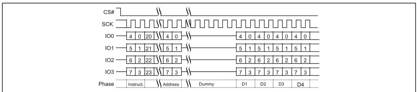
**Figure 44 RSFDP QPI mode command sequence**
