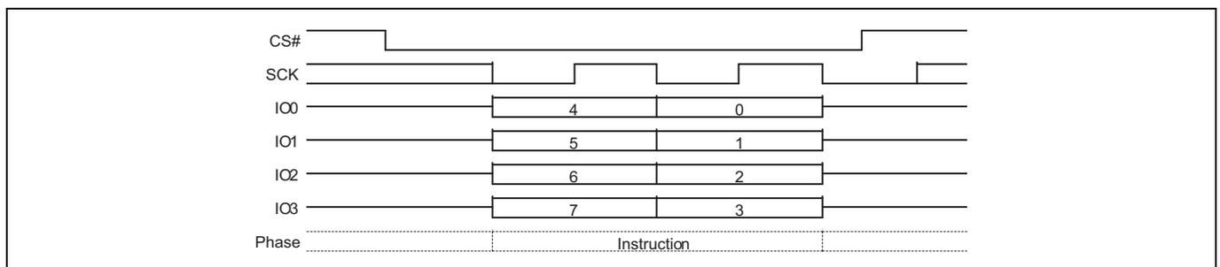
**Figure 55 Write Disable (WRDI) command sequence QPI mode**
