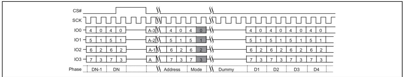
Figure 74 Continuous Quad I/O Read command sequence (EBh or ECh)<sup>[60, 61]</sup>
