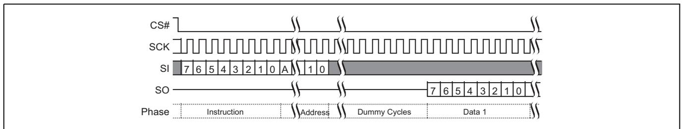
**Figure 69** Fast Read (FAST\_READ) command sequence (3-byte address, 0Bh [CR2V[7] = 0])<sup>[52]</sup>
