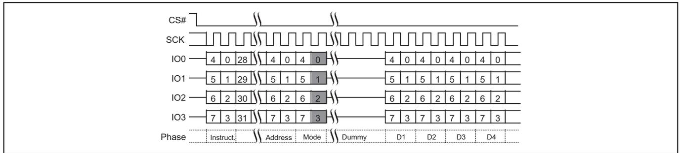
Figure 16 Quad I/O Read command in QPI mode
