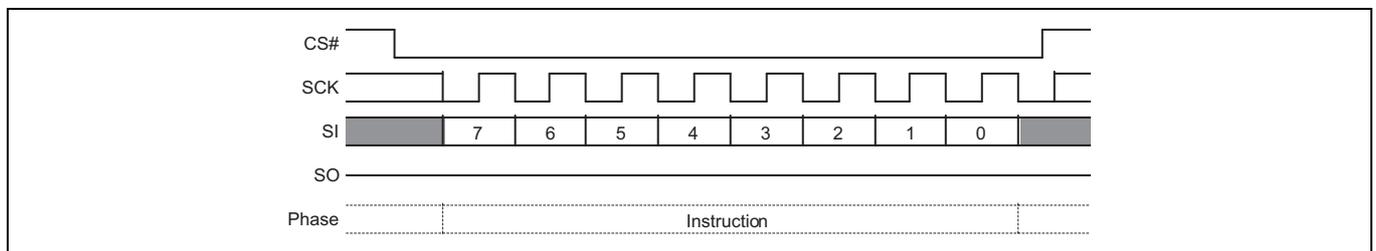
**Figure 84 Bulk Erase command sequence**
