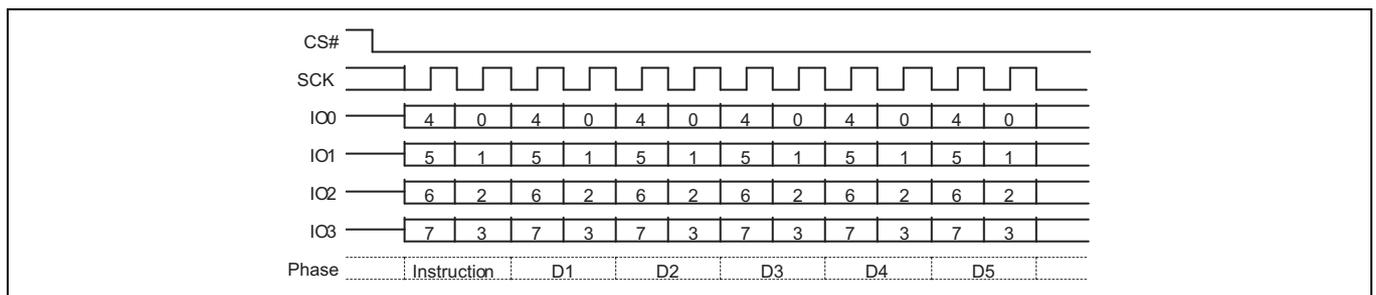
**Figure 42 Read Quad Identification (RDQID) command sequence**
