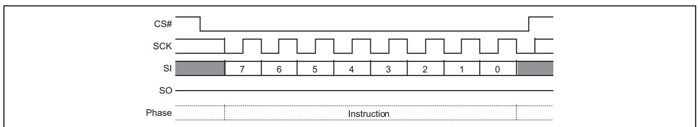
**Figure 89** Erase or Program Suspend command sequence
