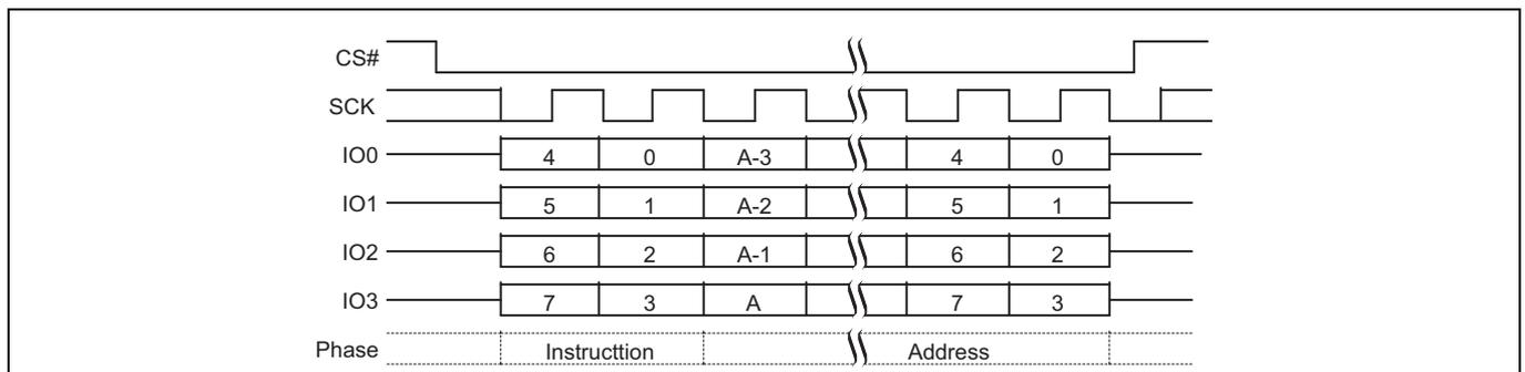
**Figure 81** Parameter Sector Erase (P4E 20h or 4P4E 21h) QPI mode command sequence<sup>[65]</sup>
