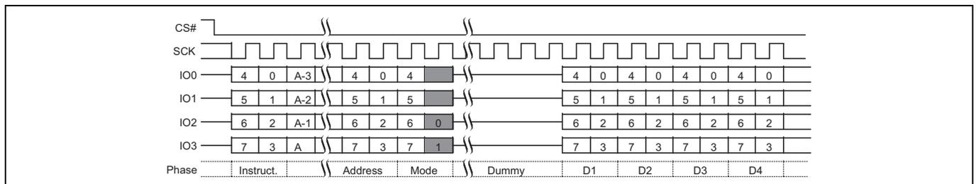
**Figure 73** Quad I/O Read command sequence (EBh or ECh), QPI Mode<sup>[58, 59]</sup>
