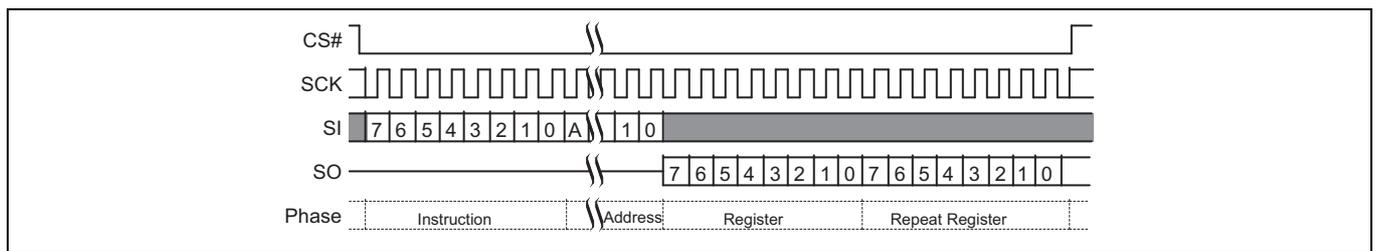
Figure 99 PPBRD command sequence<sup>[72, 73]</sup>
