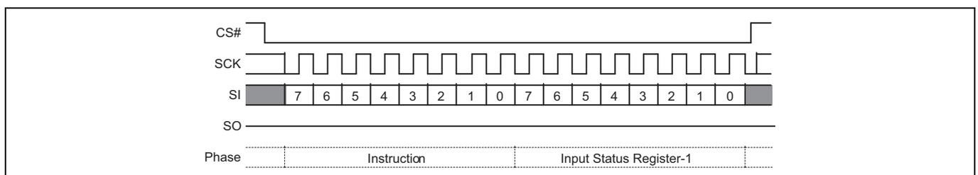
**Figure 49 Write Registers (WRR) command sequence – 8 data bits**
