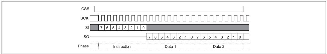
Figure 11 Single Bit Wide Output command
