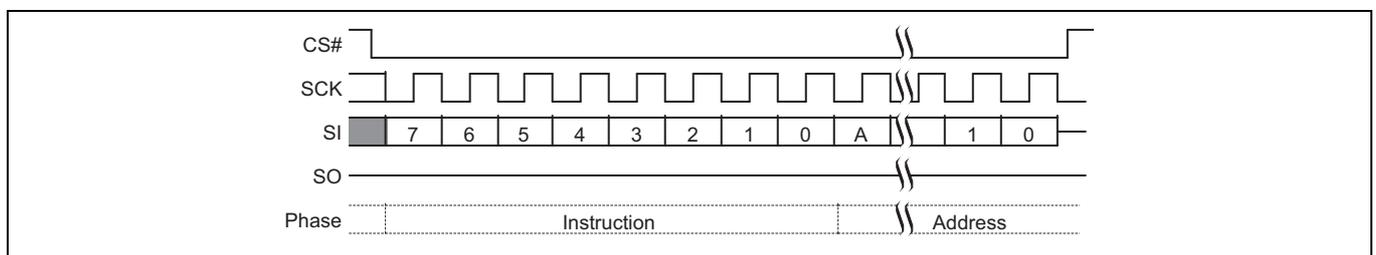
Figure 100 PPBP command sequence<sup>[74, 75]</sup>
