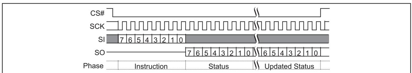
Figure 47 Read Status Register 2 (RDSR2) command
