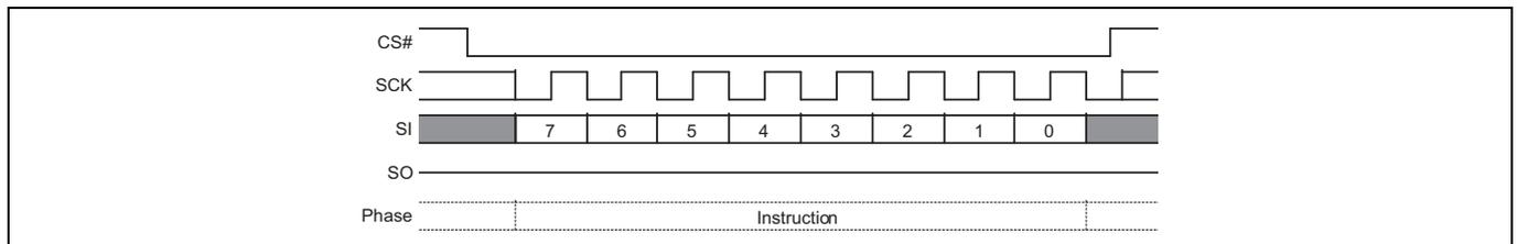
**Figure 109 Mode Bit Reset command sequence**
