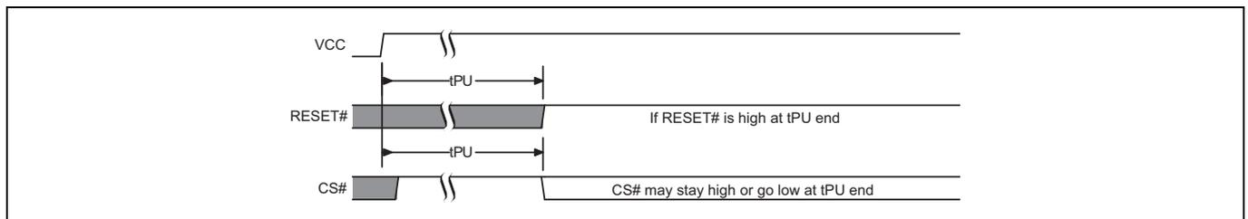
Figure 27 Reset HIGH at the end of POR
