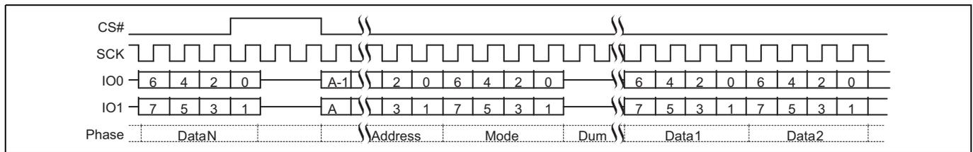
Figure 71 Dual I/O Continuous Read command sequence (BBh)<sup>[56, 57]</sup>
