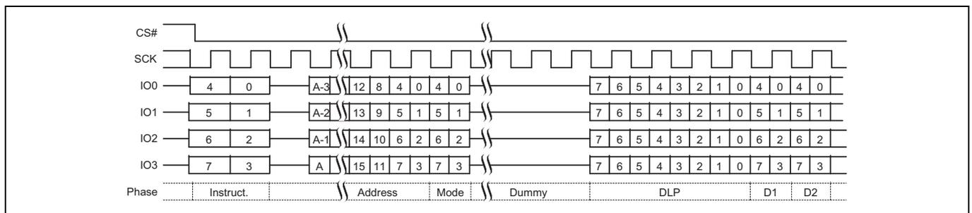
Figure 77 DDR Quad I/O Read Initial Access (EDh or EEh), QPI mode<sup>[62, 63]</sup>
