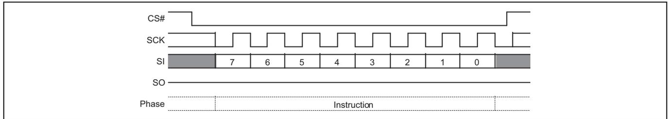
**Figure 56** Clear Status Register (CLSR) command sequence
