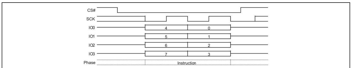
**Figure 110 Mode Bit Reset command sequence QPI mode**
