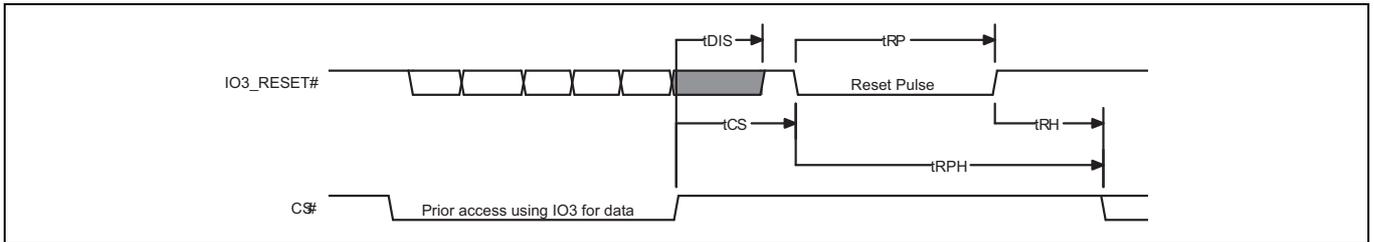
**Figure 30** Hardware reset when Quad mode and IO3 / reset# are enabled
