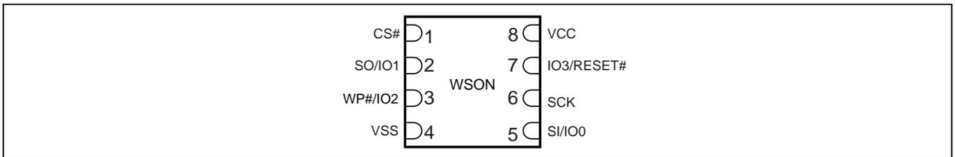
**Figure 2** 8-connector package (WSON 6 x 8), top view<sup>[9, 10]</sup>
