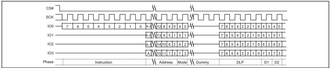
Figure 75 DDR Quad I/O Read Initial Access (EDh or EEh)<sup>[62, 63]</sup>
