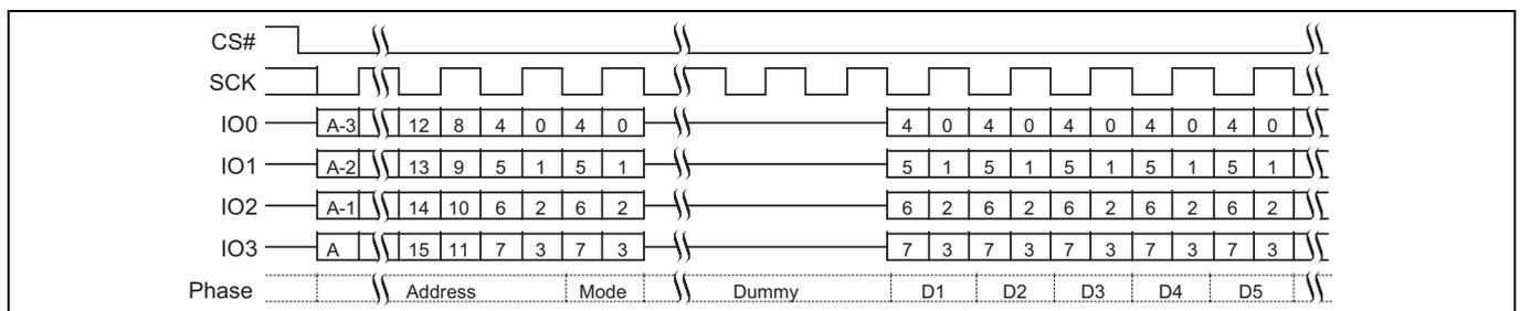
Figure 76 Continuous DDR Quad I/O Read Subsequent Access (EDh or EEh)<sup>[62, 63]</sup>
