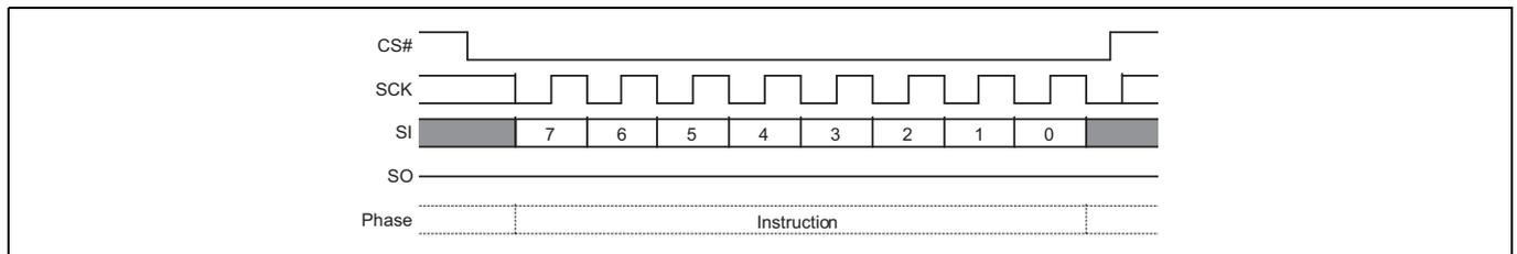
Figure 103 PPB Lock Bit Write command sequence
