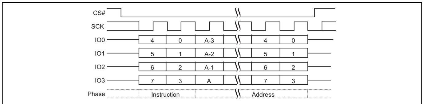
**Figure 83 Sector Erase (SE D8h or 4SE DCh) QPI mode command sequence<sup>[66]</sup>**
