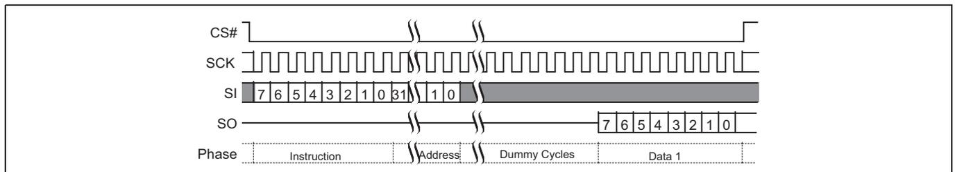
Figure 13 Single Bit Wide I/O command with latency
