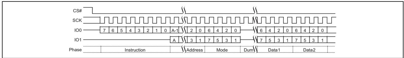
Figure 70 Dual I/O Read command sequence (BBh)<sup>[53-55]</sup>
