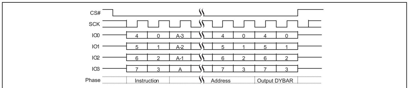
Figure 96 DYBRD QPI mode command sequence<sup>[68, 69]</sup>
