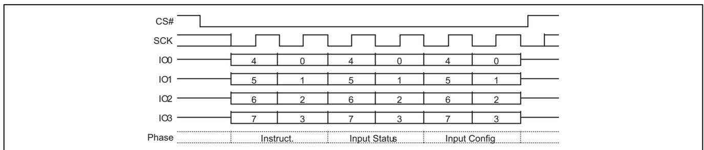
**Figure 51 Write Registers (WRR) command sequence – 16 data bits QPI mode**
