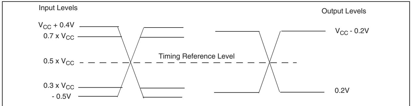
**Figure 25** Input, output, and timing reference levels
