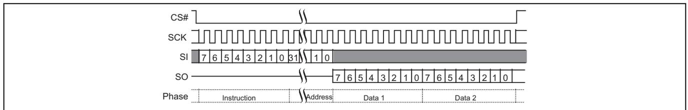
Figure 12 Single Bit Wide I/O command without latency
