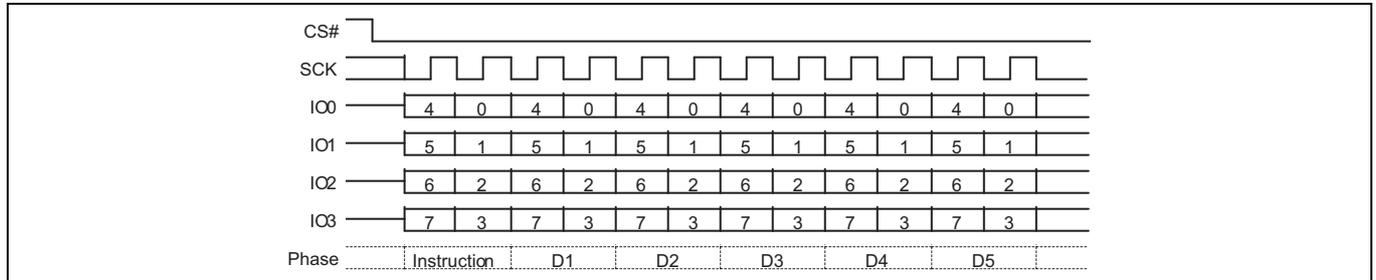
**Figure 41 Read Identification (RDID) QPI mode command**
