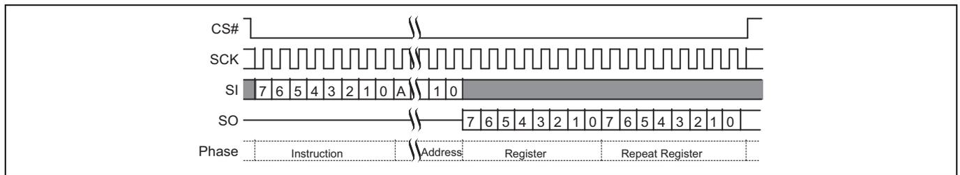
Figure 95 DYBRD command sequence<sup>[68, 69]</sup>
