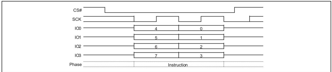
**Figure 53 Write Enable (WREN) command sequence QPI mode**
