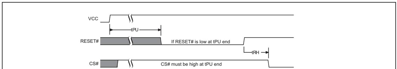
Figure 26 Reset LOW at the end of POR
