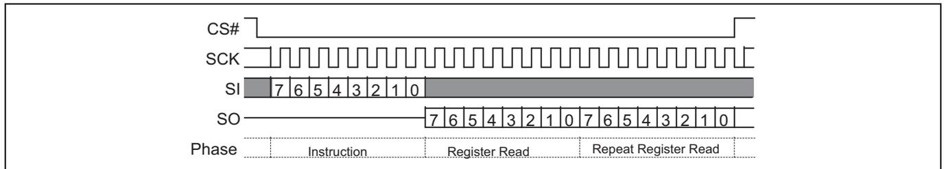
**Figure 48 Read Configuration Register (RDCR) command sequence**
