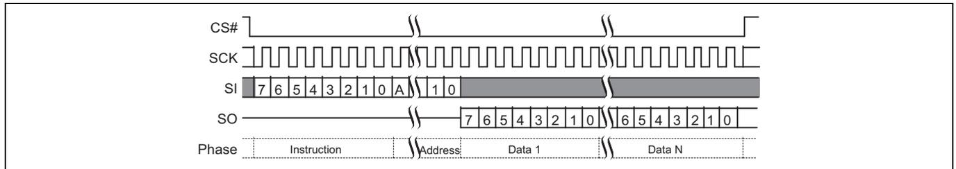
**Figure 68** Read command sequence (3-byte address, 03h or 13h)
