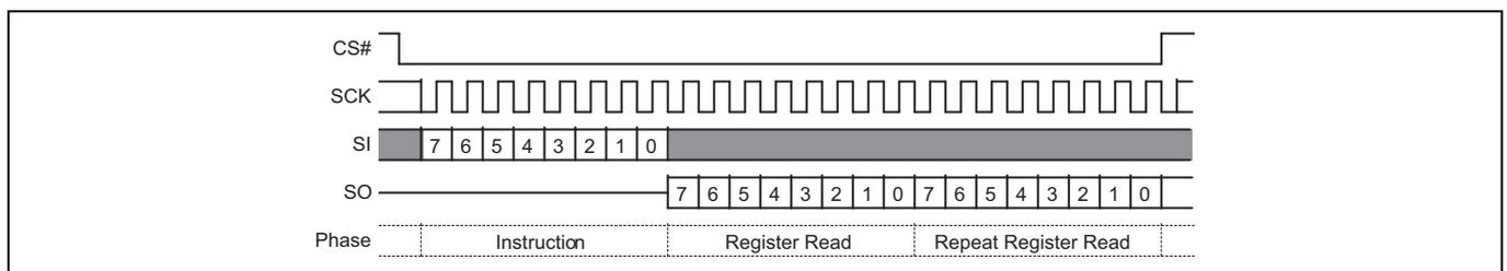
**Figure 102 PPB Lock Register Read command sequence**
