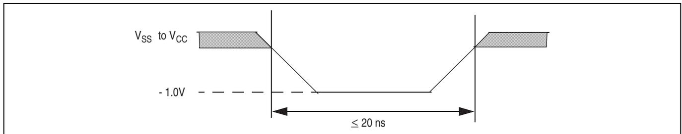
**Figure 19** Maximum negative overshoot waveform
