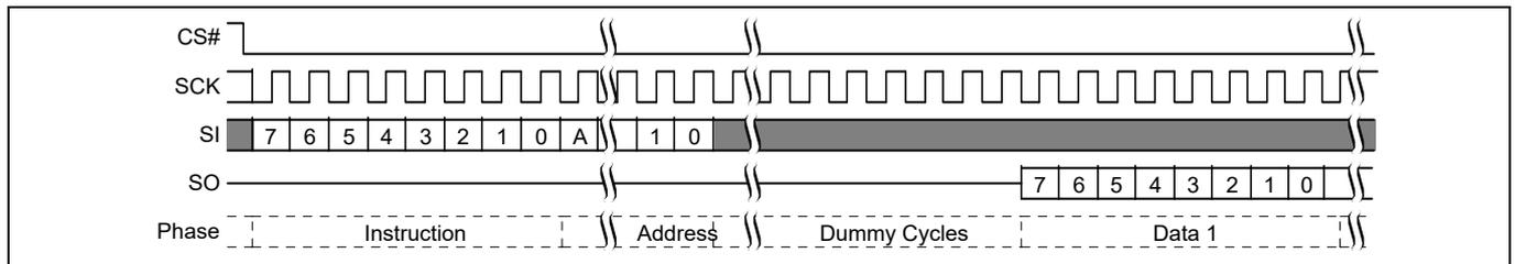
Figure 58 ECC Status Register Read command sequence<sup>[48, 49]</sup>
