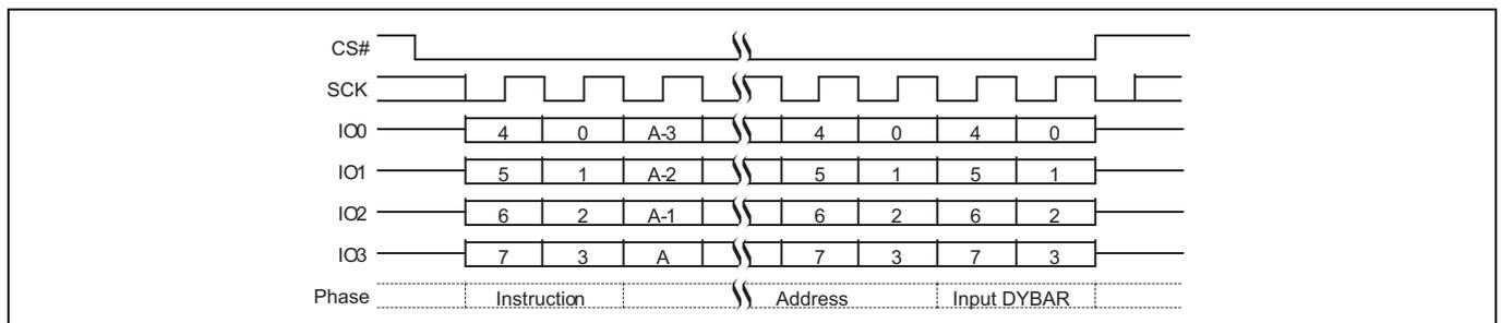
**Figure 98** DYBWR QPI mode command sequence<sup>[70, 71]</sup>
