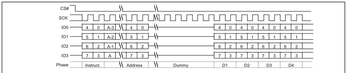
**Figure 66** Read Any Register, QPI Mode, command sequence<sup>[50]</sup>
