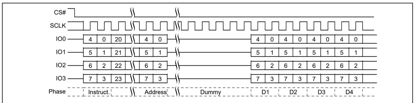
Figure 59 ECCRD (19h), QPI mode, CR2[7] = 0, command sequence
