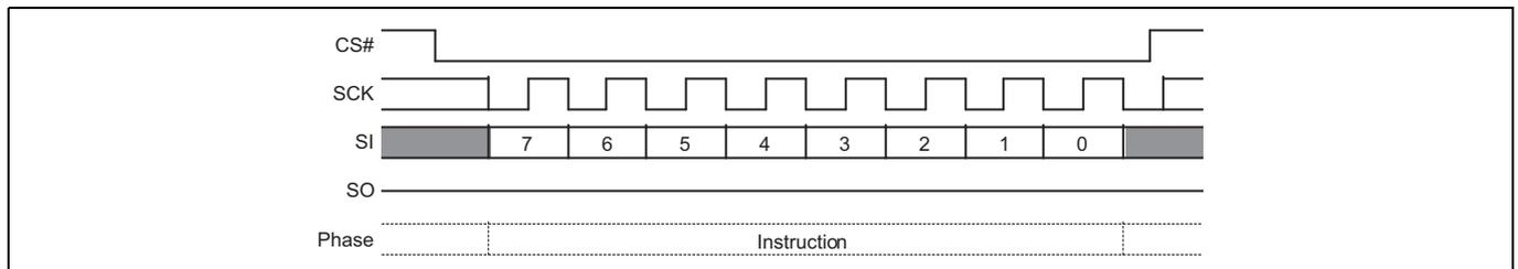
**Figure 64 Enter 4-Byte Address mode (4BAM B7h) command sequence**
