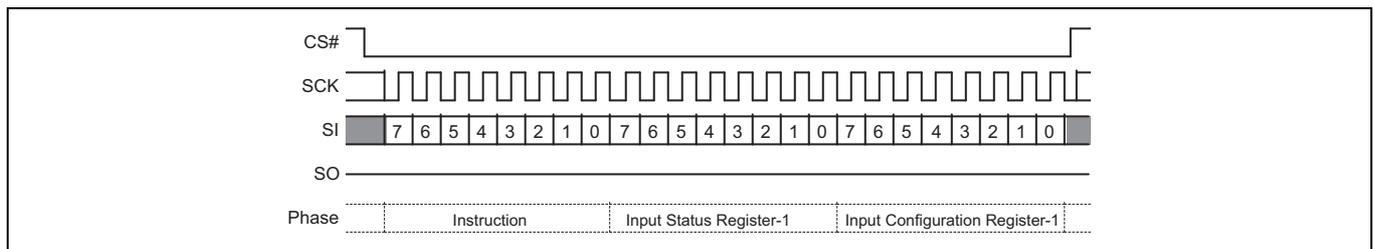
**Figure 50 Write Registers (WRR) command sequence – 16 data bits**
