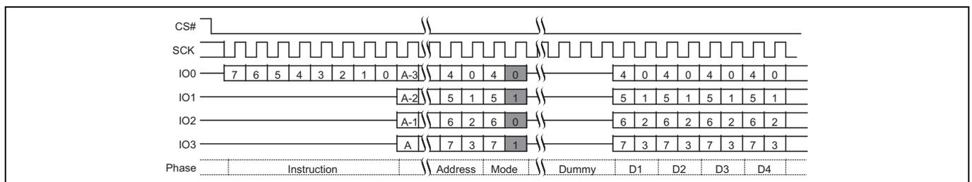
**Figure 72** Quad I/O Read command sequence (EBh or ECh)<sup>[58, 59]</sup>
