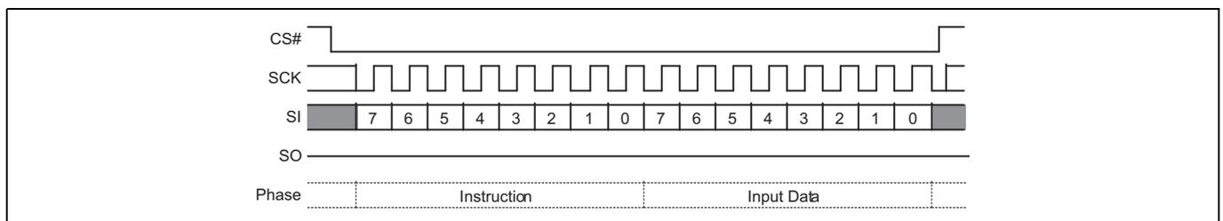
**Figure 61 Program NVDLR (PNVDLR) command sequence**
