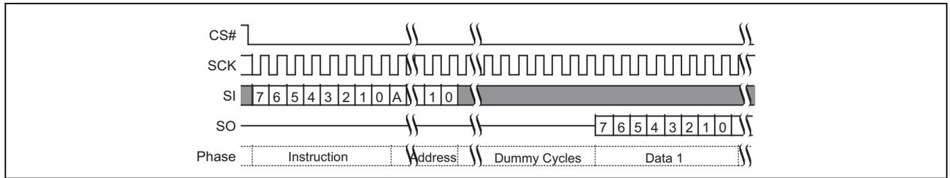
**Figure 65** Read Any Register Read command sequence<sup>[50]</sup>
