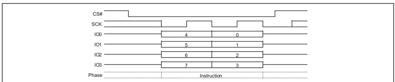
**Figure 108 Software Reset command sequence QPI mode**
