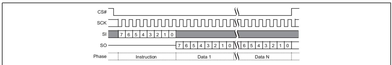
Figure 104 Password Read command sequence
