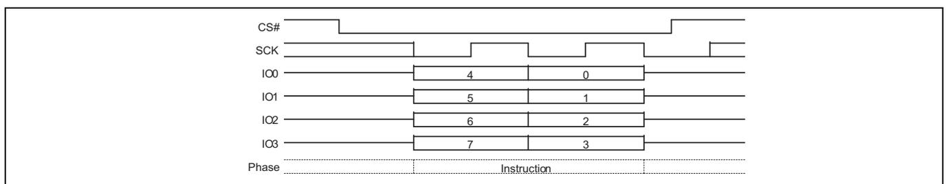
**Figure 85 Bulk Erase command sequence QPI mode**
