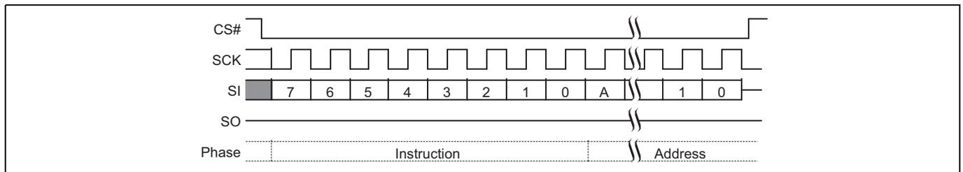
**Figure 82 Sector Erase (SE D8h or 4SE DCh) command sequence<sup>[66]</sup>**
