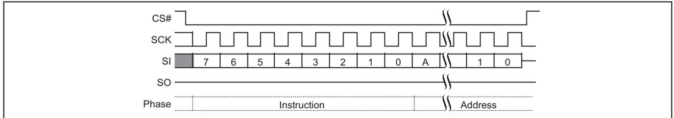
**Figure 80** Parameter Sector Erase (P4E 20h or 4P4E 21h) command sequence<sup>[65]</sup>
