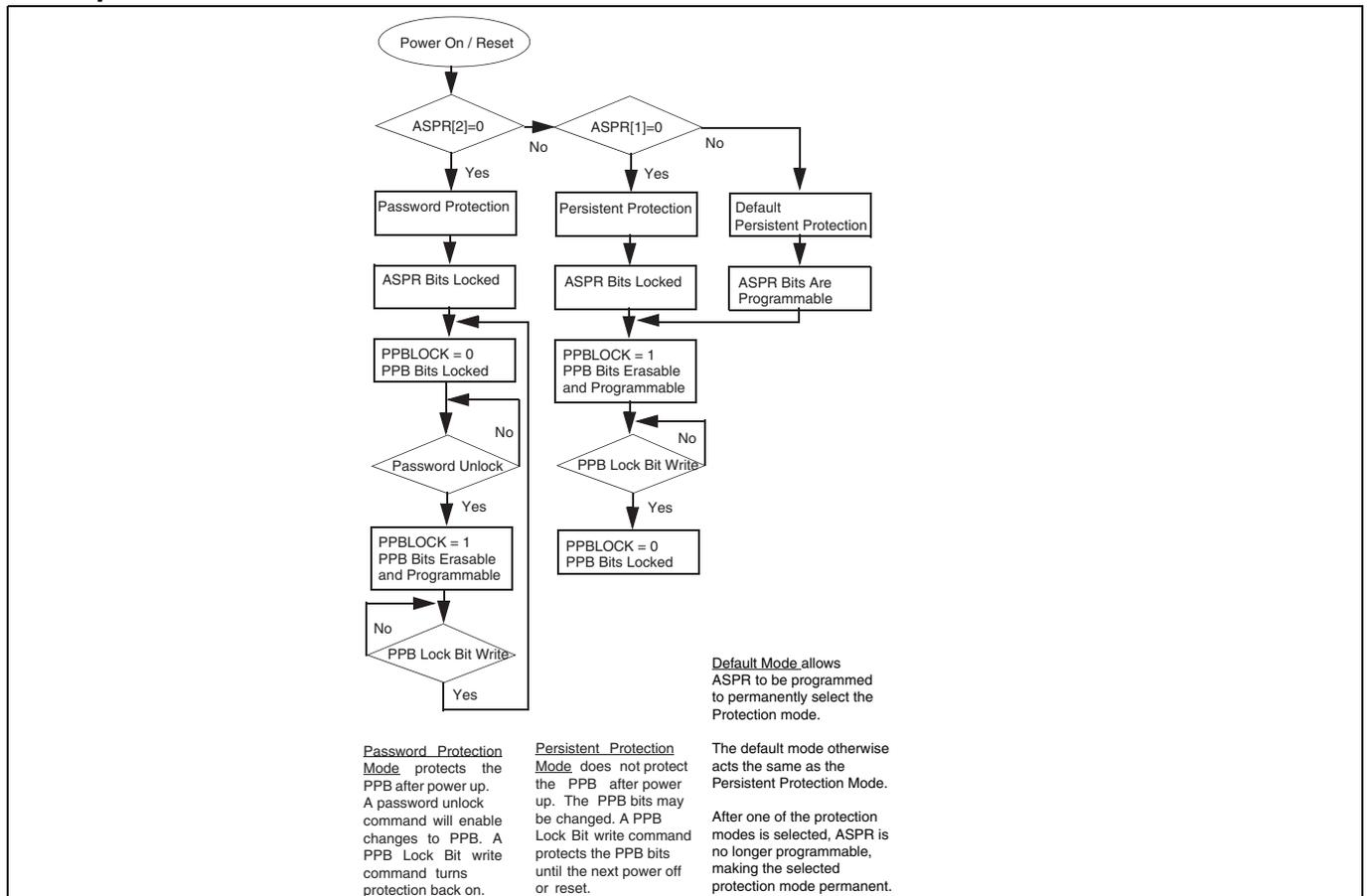
**Advanced sector protection overview** The Persistent Protection method sets the PPB Lock bit to 1 during POR, or Hardware Reset so that the PPB bits are unprotected by a device reset. There is a command to clear the PPB Lock bit to 0 to protect the PPB. There is no command in the Persistent Protection method to set the PPB Lock bit to 1, therefore the PPB Lock bit will remain at 0 until the next power-off or hardware reset. The Persistent
