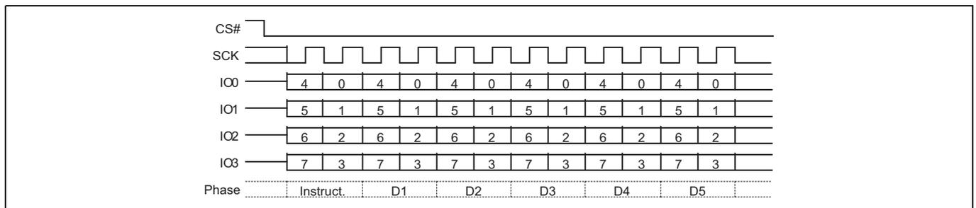
Figure 46 Read Status Register 1 (RDSR1) QPI Mode command
