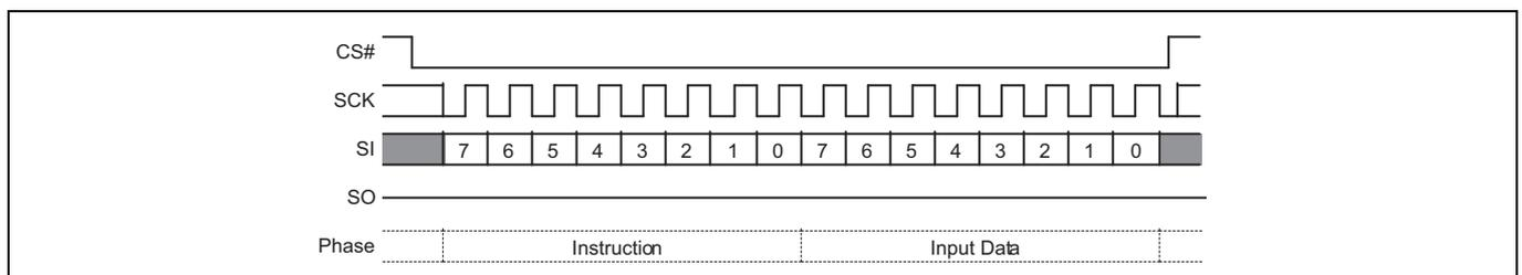
**Figure 62 Write VDLR (WVDLR) command sequence**
