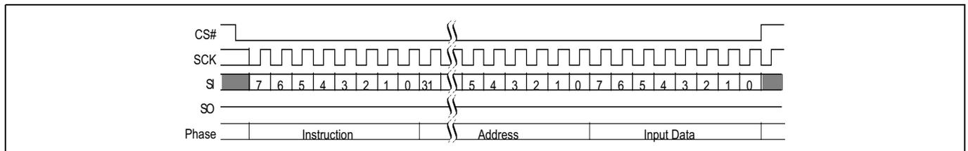
**Figure 97** DYBWR command sequence<sup>[70, 71]</sup>
