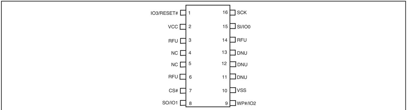
**Figure 1** 16-lead SOIC package, Top view<sup>[9]</sup>
