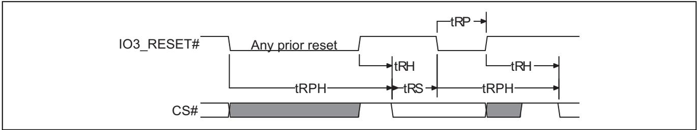
**Figure 29** Hardware reset when Quad mode is not enabled and IO3 / reset# is enabled
