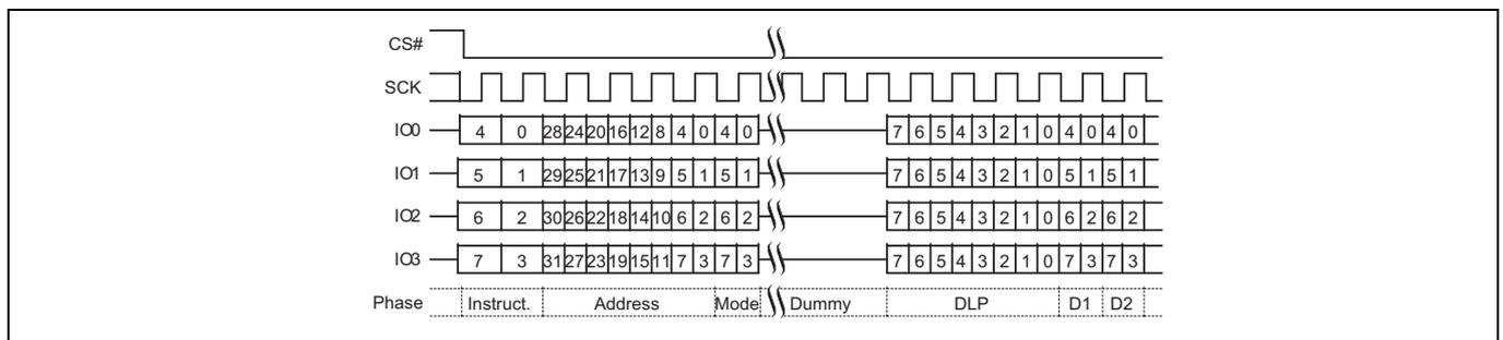
Figure 18 DDR Quad I/O Read in QPI mode
