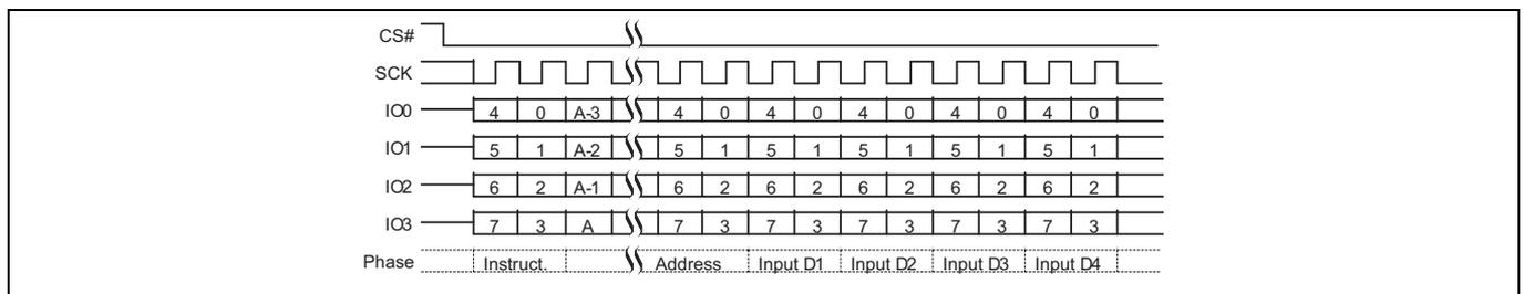
**Figure 79** Page Program (PP 02h or 4PP 12h) QPI mode command sequence<sup>[64]</sup>
