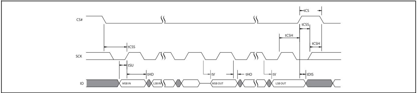
Figure 34 SPI SDR MIO timing
