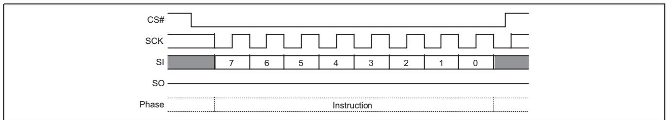
**Figure 113 Release from Deep Power-Down command sequence**
