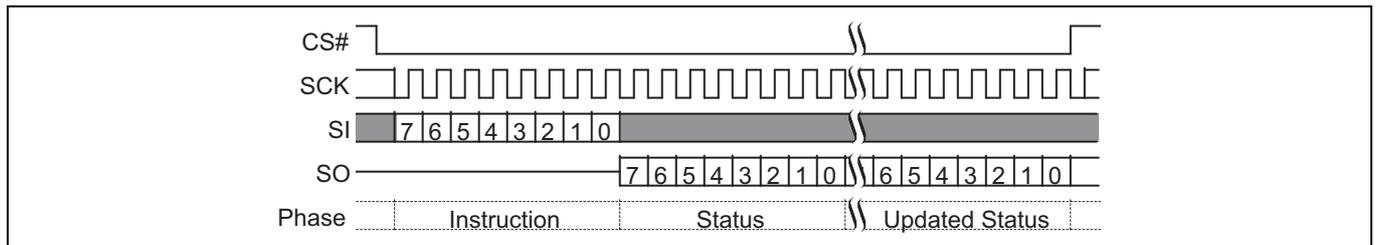
Figure 45 Read Status Register 1 (RDSR1) command sequence
