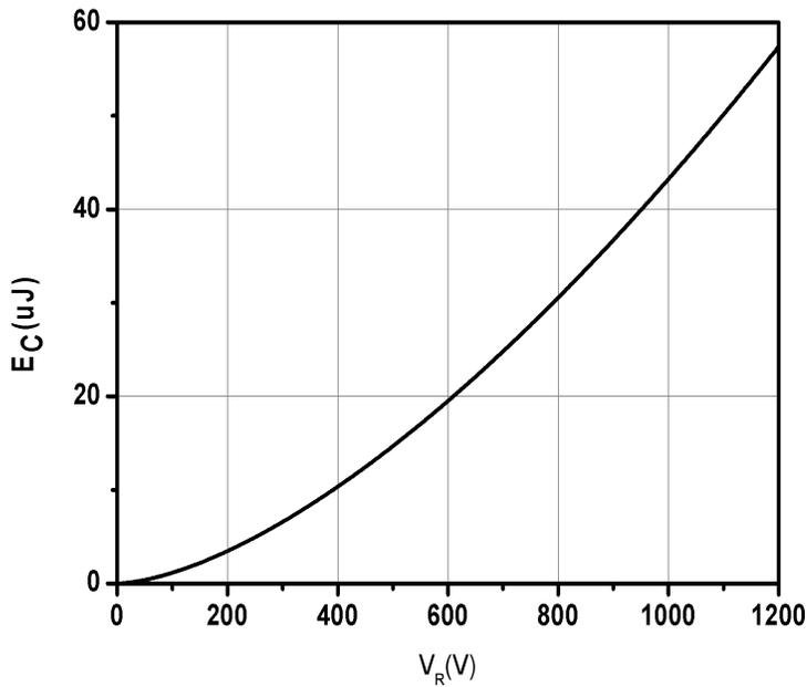
Fig.7-Capacitance Stored Energy
