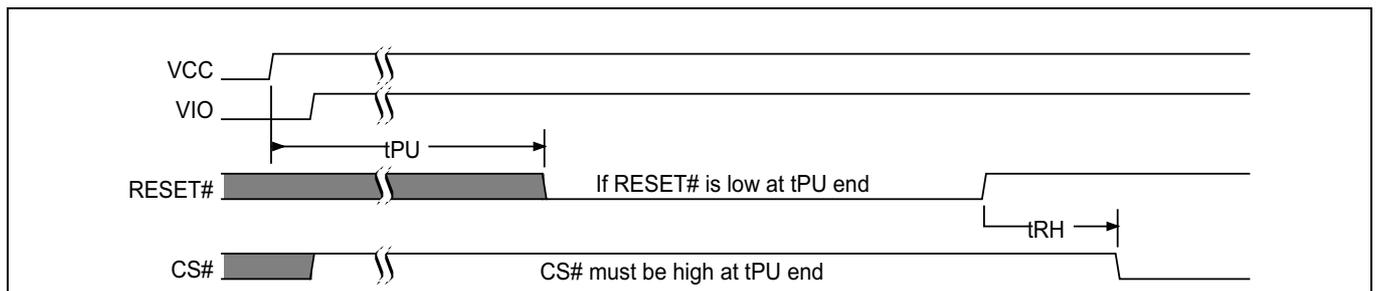
Figure 18 Reset LOW at the end of POR
