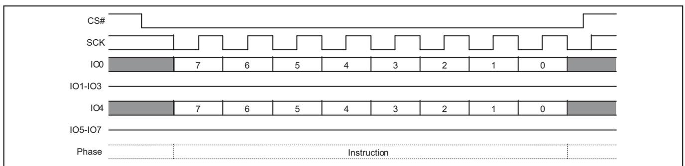
Figure 75 PPB Erase (PPBE E4h) command sequence
