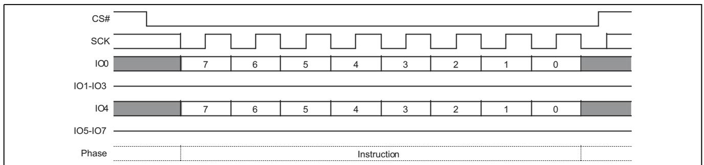
Figure 43 Dual-Quad Write Enable (WREN 06h) command sequence
