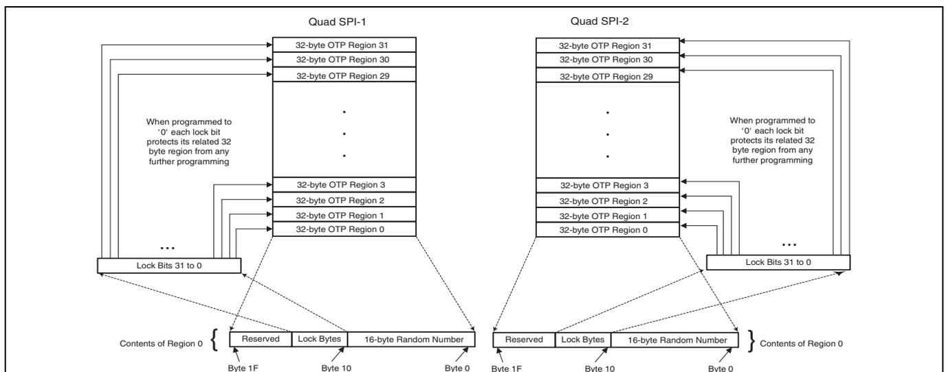
**Figure 29** OTP address space — Quad SPI-1 and Quad SPI-2
