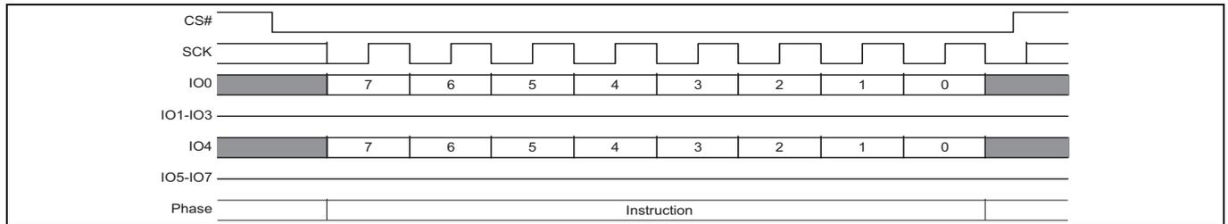
Figure 67 Dual-Quad Erase Resume command sequence
