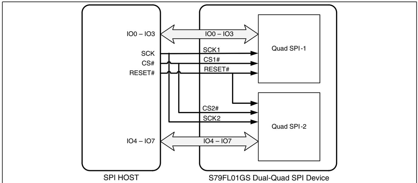
**Figure 1** SPI host and S79FL01GS dual-quad SPI device with dual CS# and SCK balls in the 24-ball BGA package (5x5 ball configuration)
