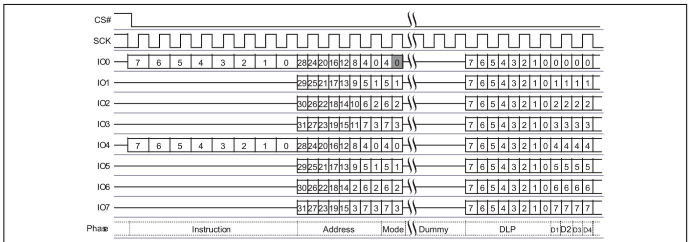
Figure 10 Dual-Quad DDR Quad I/O Read command
