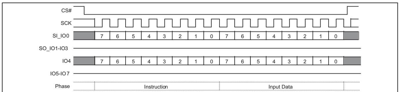
**Figure 51 Write VDLR (WVDLR 4Ah) command sequence**
