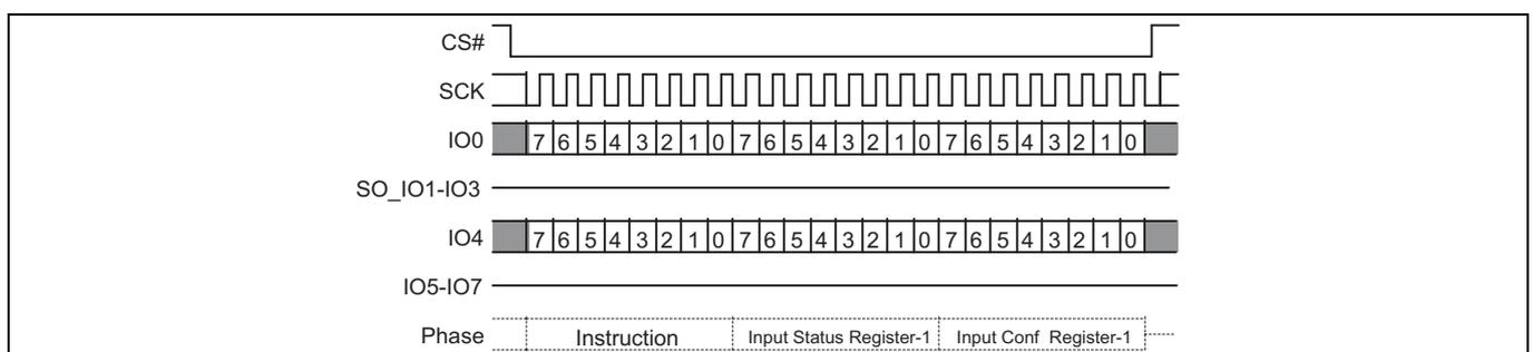
Figure 42 Dual-Quad Write Registers (WRR 01h) command sequence
