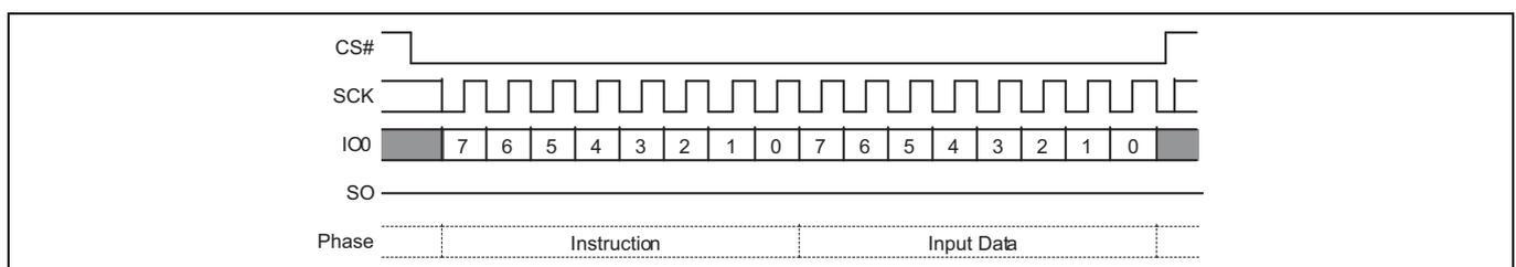
**Figure 5 Dual-Quad Single bit Wide Input command**
