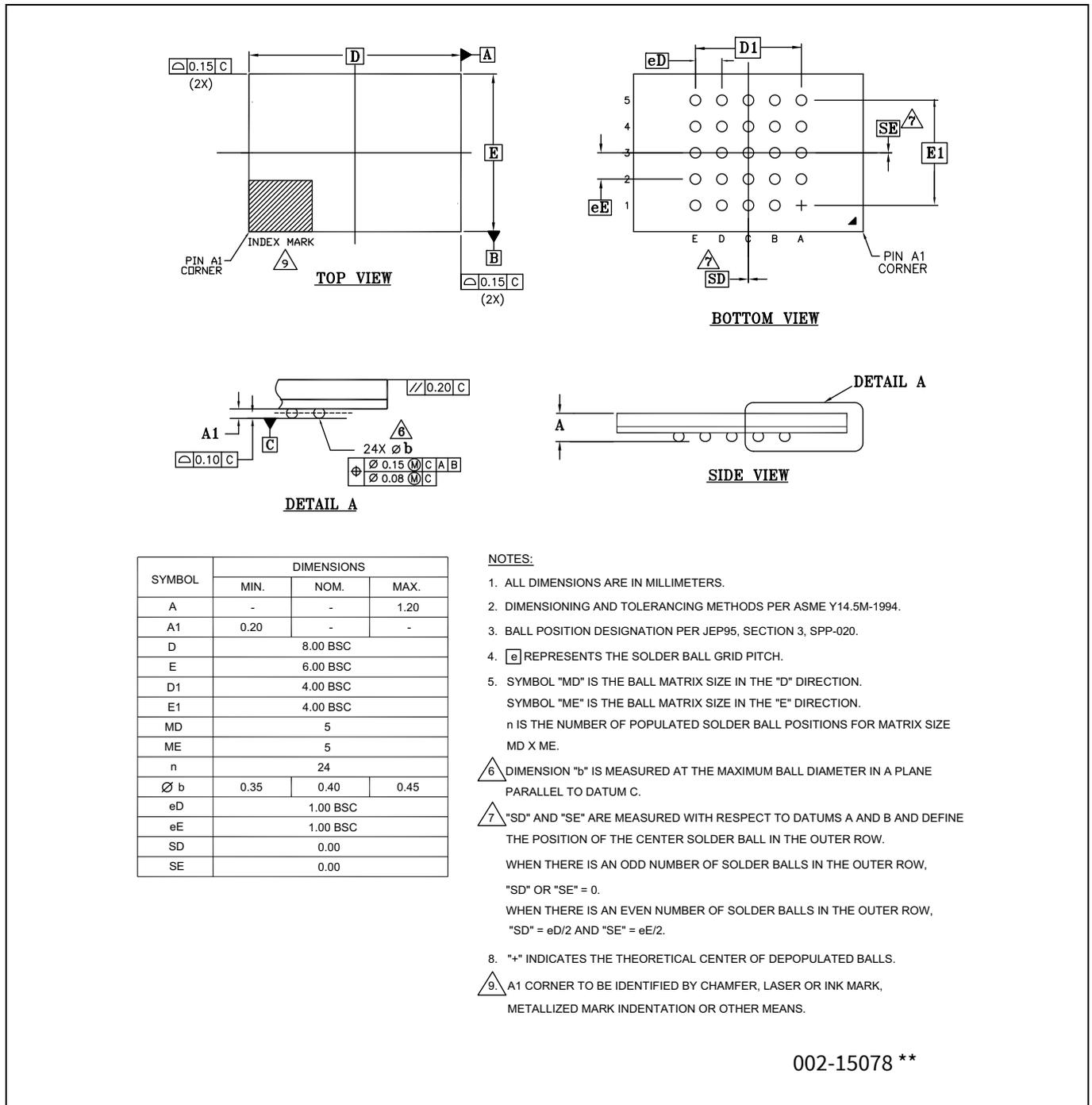
Figure 28 24-ball FBGA (8.0 × 6.0 × 1.2 mm) package outline (PG-TFBGA-24), 002-15078
