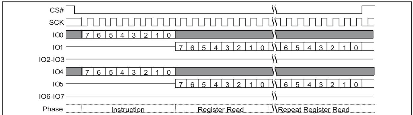
**Figure 37 Dual-Quad Read Configuration Register (RDCR 35h) command sequence**
