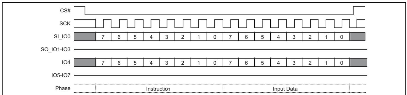
**Figure 50 Program NVDLR (PNVDLR 43h) command sequence**
