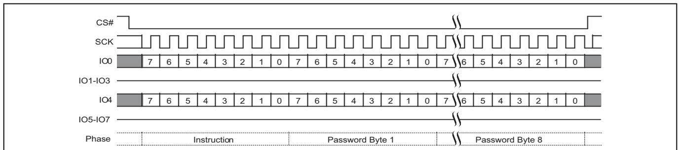
**Figure 79 Password Program (PASSP E8h) command sequence**
