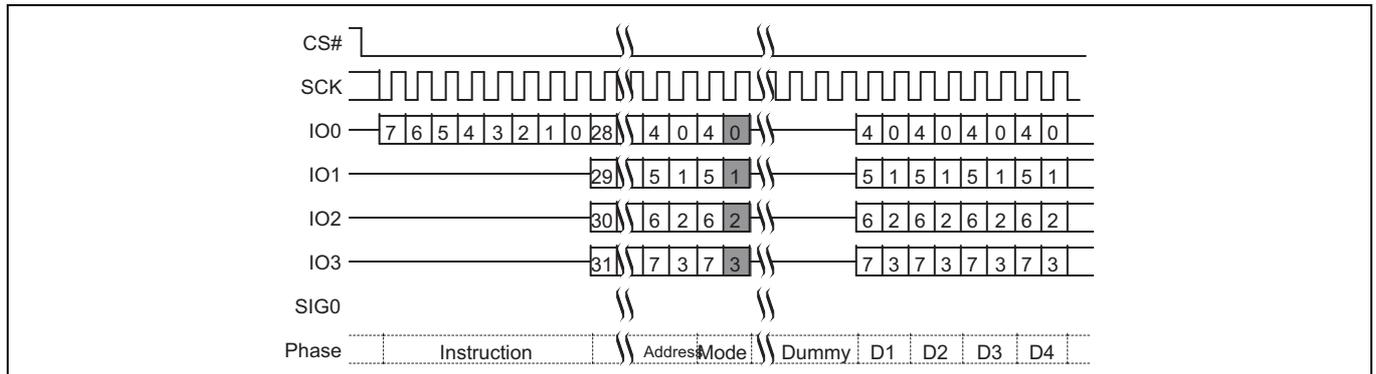
Figure 9 Dual-Quad, Quad I/O command
