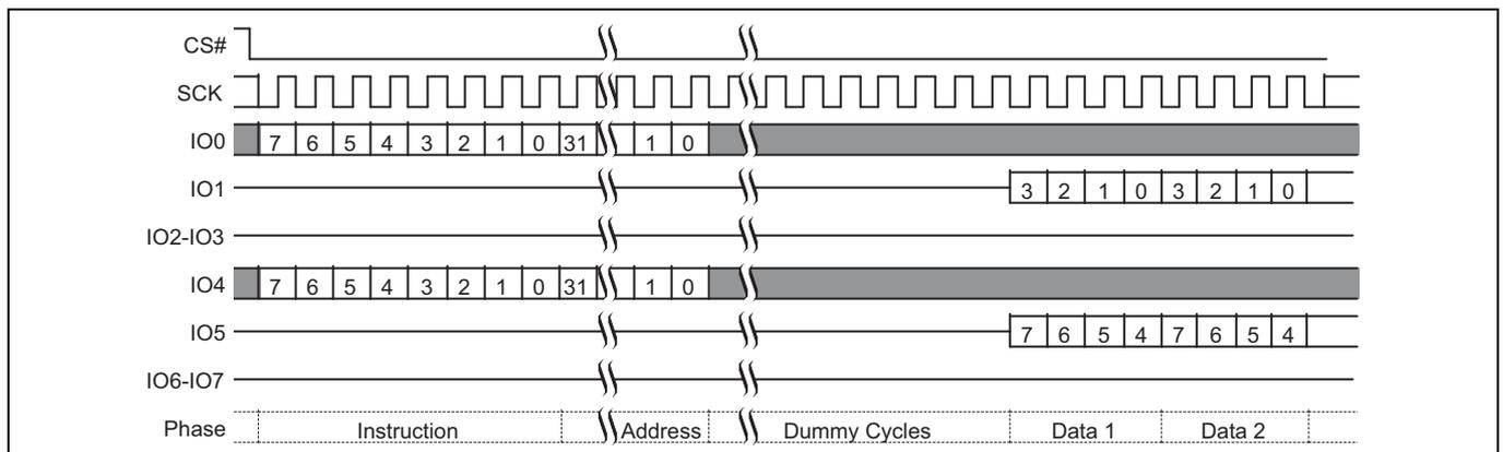
**Figure 54 Dual-Quad SPI Fast Read (FAST\_READ) command sequence**
