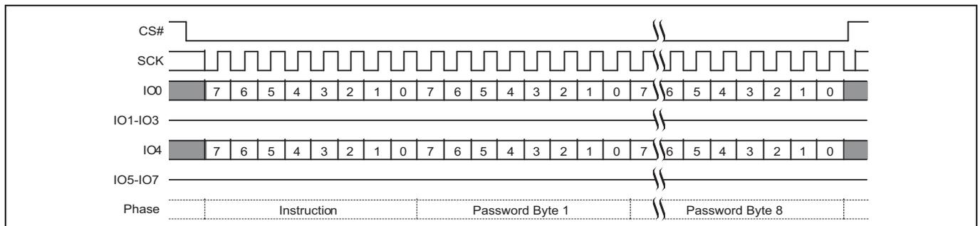
**Figure 80 Password Unlock (PASSU E9h) command sequence**
