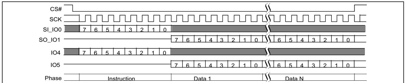
Figure 48 AutoBoot Register Read (ABRD 14h) command
