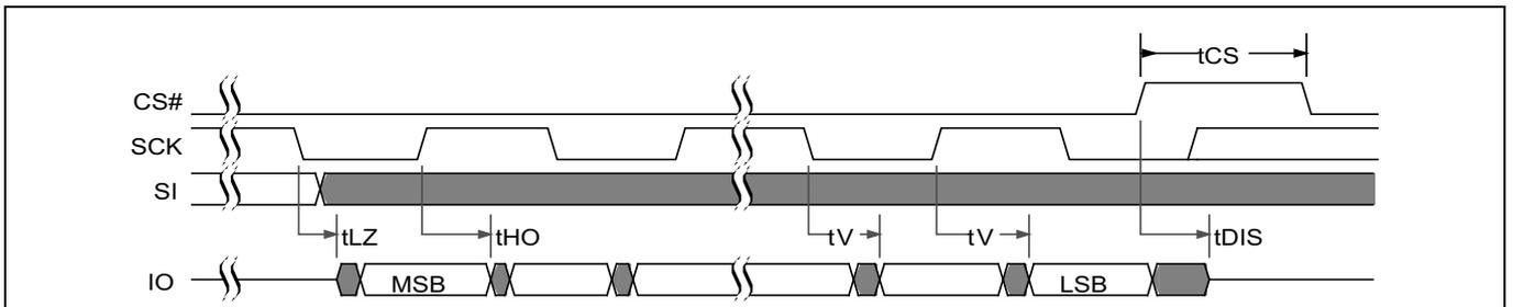
Figure 25 SPI DDR output timing
