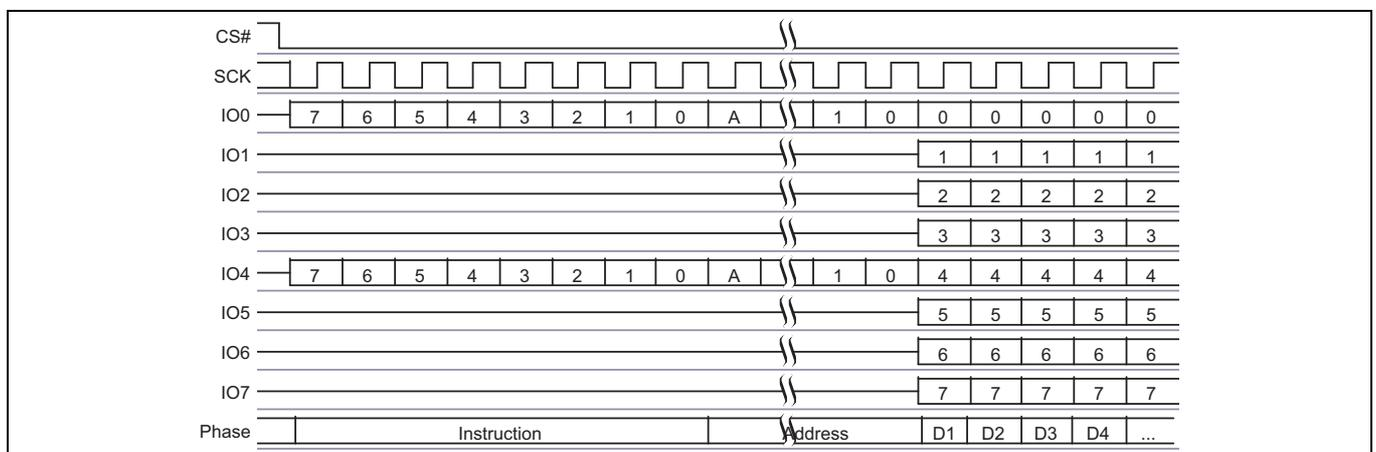
**Figure 61** Dual-Quad, Quad Page Program command sequence
