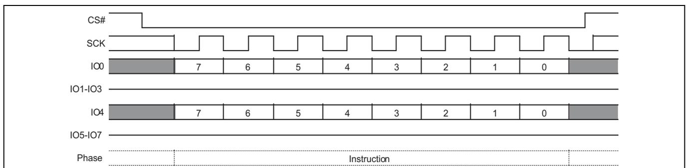
Figure 81 Dual-Quad Software Reset (RESET F0h) command sequence
