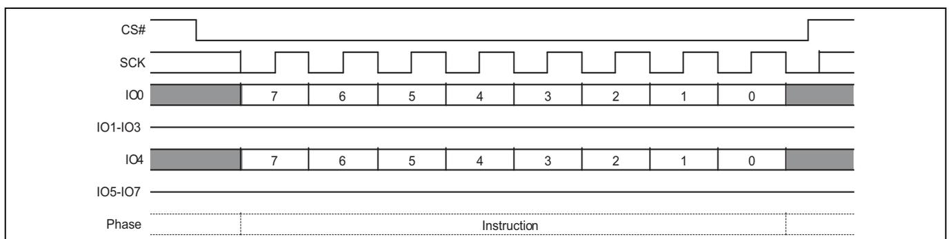
Figure 82 Dual-Quad SPI Mode Bit (MBR FFh) Reset command sequence
