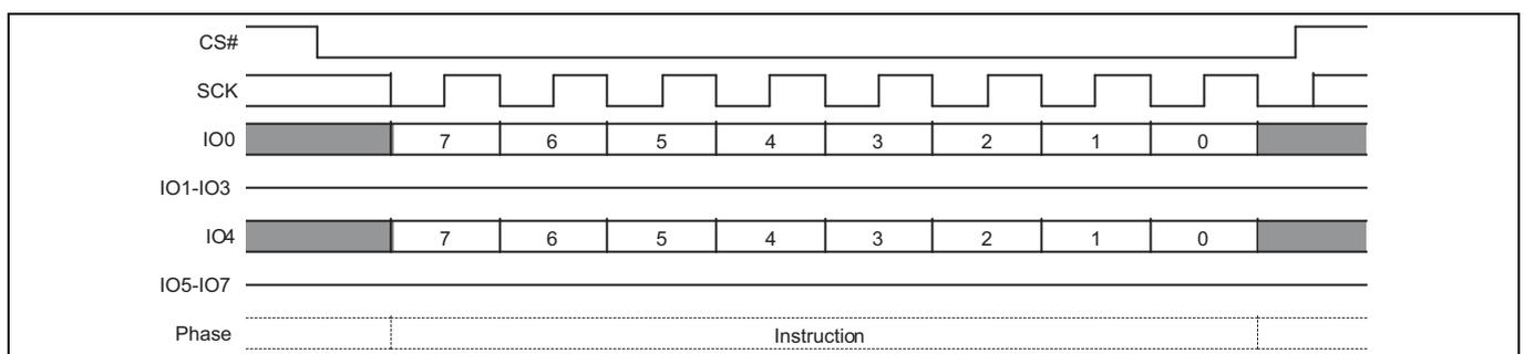
Figure 44 Dual-Quad Write Disable (WRDI 04h) command sequence
