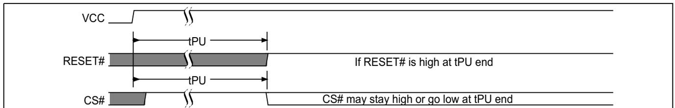
Figure 19 Reset HIGH at the end of POR
