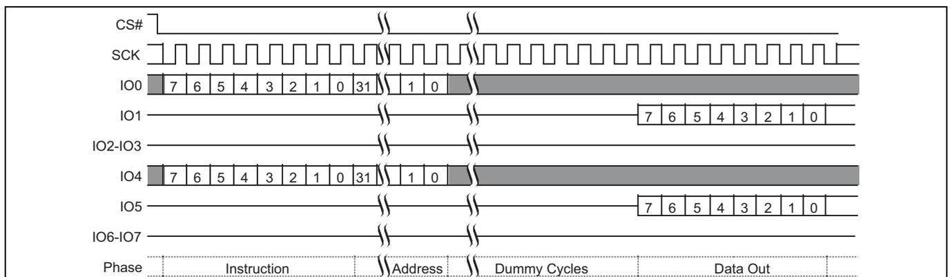
Figure 46 ECC Status Register Read command sequence
