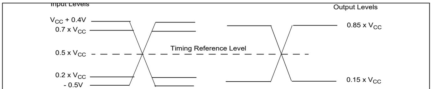
Figure 16 Input, output, and timing reference levels
