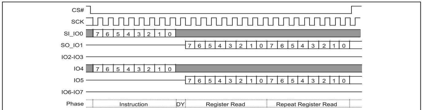
Figure 73 PPBRD (E2h) command sequence
