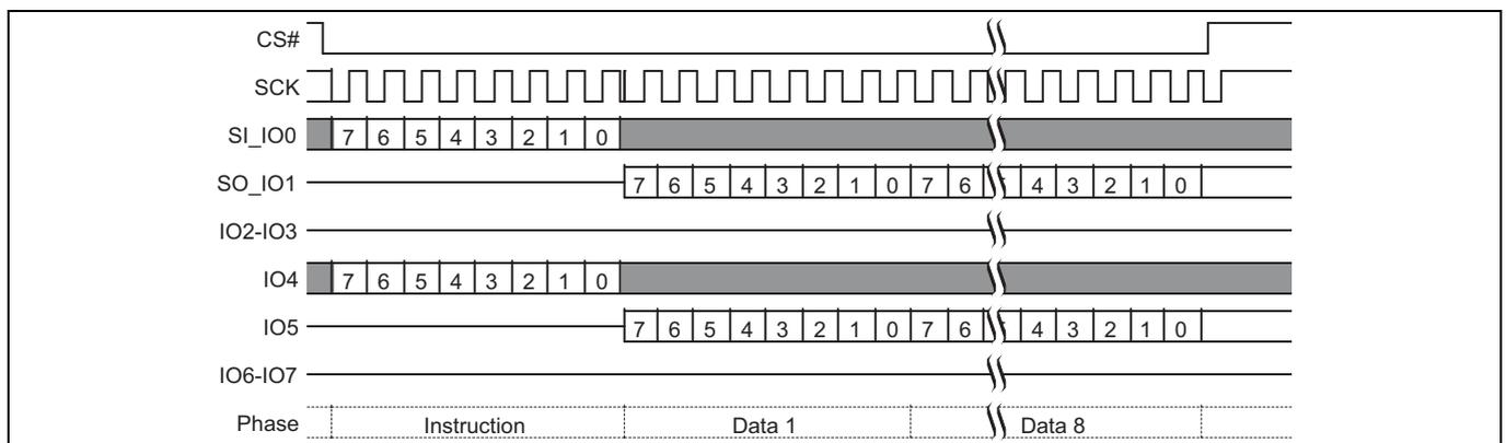
Figure 78 Password Read (PASSRD E7h) command sequence
