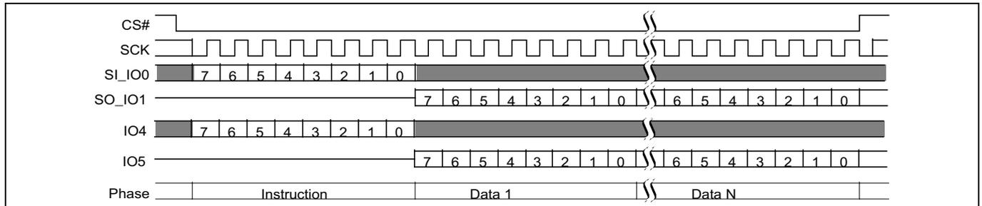
**Figure 52 Dual-Quad DLP Read (DLPRD 41h) command sequence**
