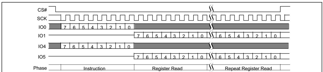
**Figure 38 Read Bank Register (BRRD 16h) command**
