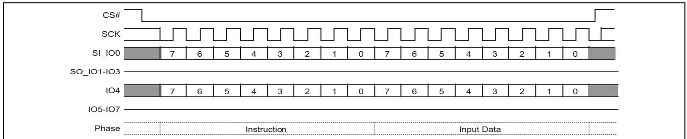
**Figure 39 Bank Register Write (BRWR 17h) command**
