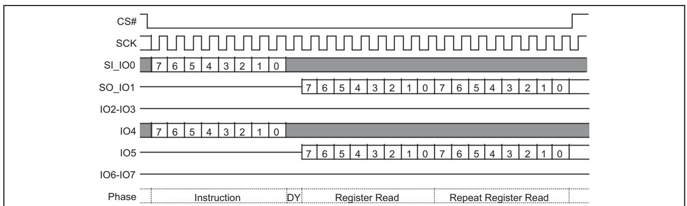
Figure 76 PPB Lock Register Read command sequence
