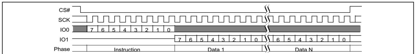
**Figure 32 Read Identification (RDID 9Fh) command sequence**
