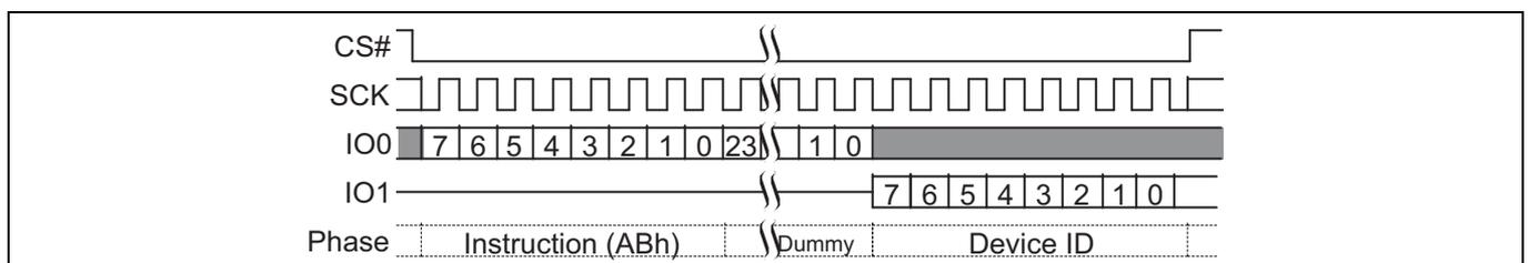
Figure 33 Read Electronic Signature (RES ABh) command sequence
