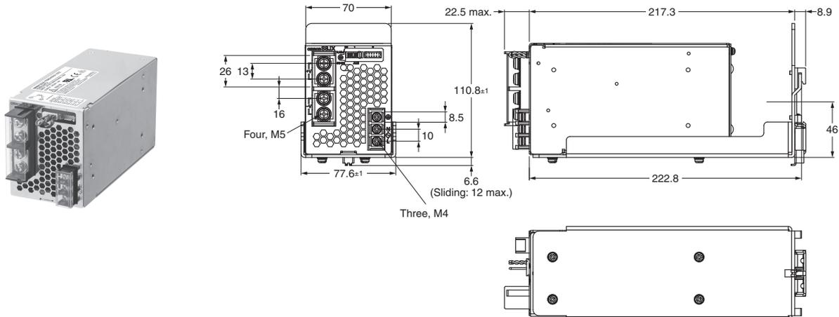
**Note:** Use a metal DIN Rail when mounting a 300-W model to a DIN Rail.
