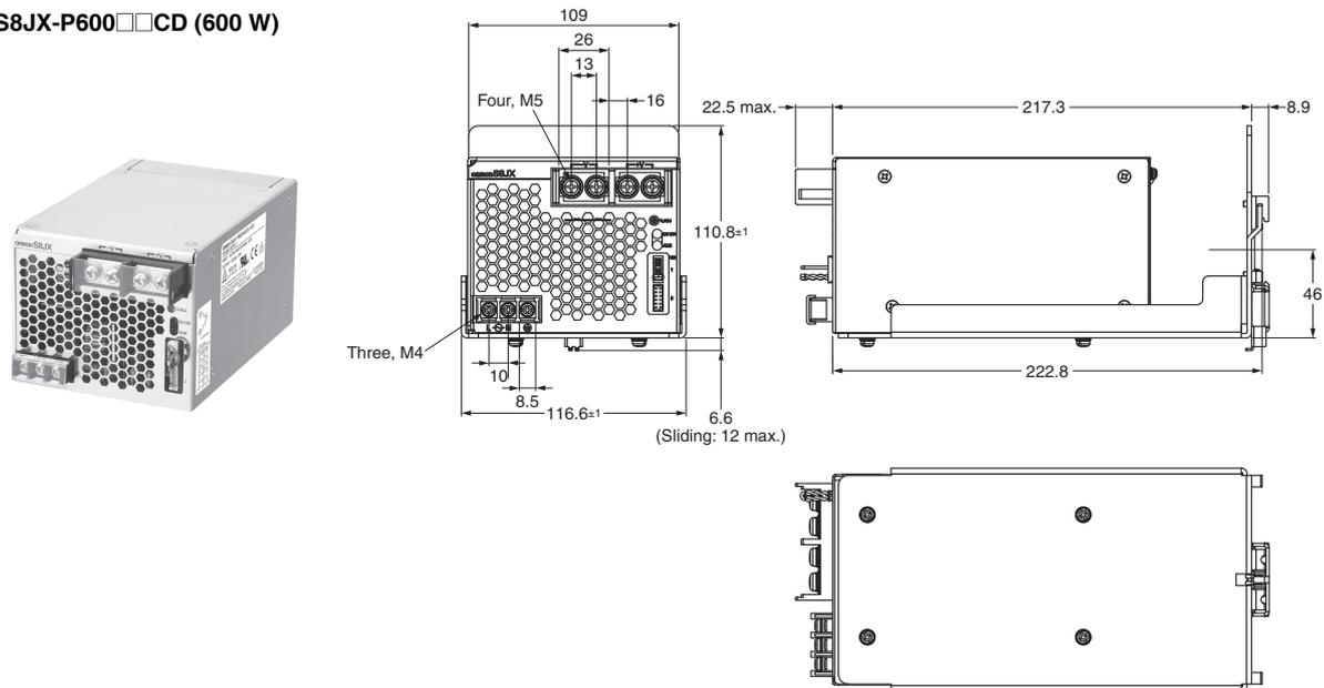
**Note:** Use a metal DIN Rail when mounting a 600-W model to a DIN Rail.
