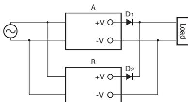
The same model should be used for power supplies A and B.
