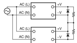
**Note: 1.** If the load is short-circuited, a reverse voltage will be generated inside the Power Supply. If this occurs the Power Supply may possibly deteriorate or be damaged. Always connect a diode as shown in the figure. Select a diode having the following ratings.
