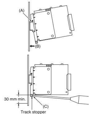
To dismount the Power Supply, pull down portion (C) with a flat-blade screwdriver and pull out the Power Supply.
