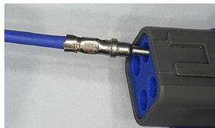
Line the contact up with the grommet.
