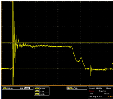
IEC 61000-4-2 +8 kV Contact ESD Clamping Voltage
