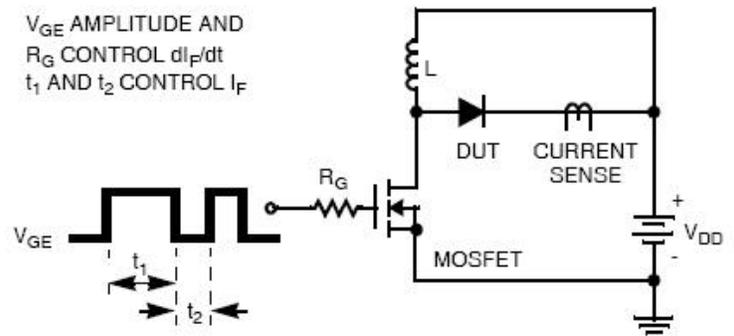
Fig.4-Diode Test Circuit
