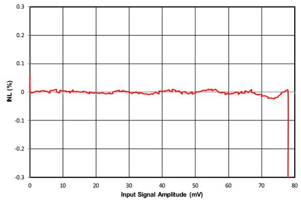
Figure 12. Si8922A Nonlinearity (%) vs. Input Signal Amplitude (mV)
