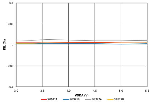
Figure 8. Nonlinearity (%) vs. VDDA Supply (V)
