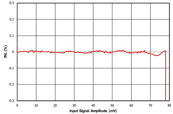
Figure 10. Si8921A Nonlinearity (%) vs. Input Signal Amplitude (mV)
