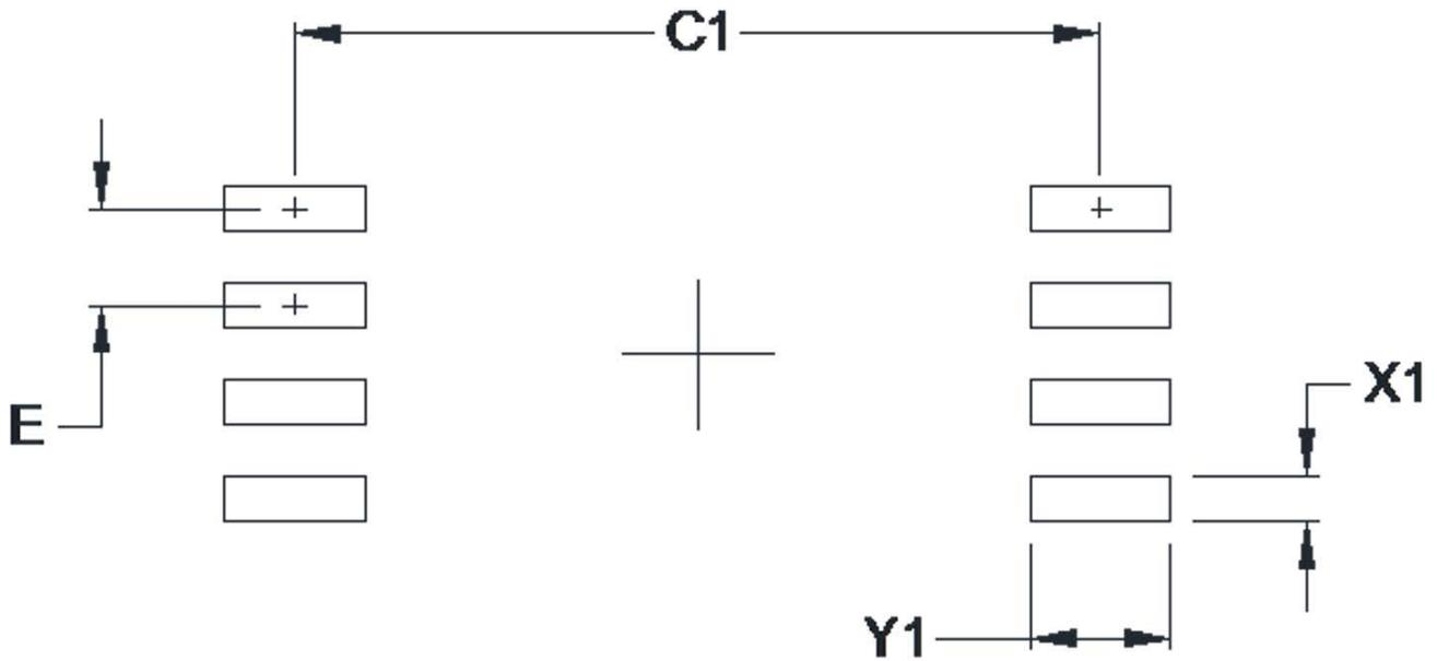
Figure 45. 8-Pin Wide Body Stretched SOIC Land Pattern
