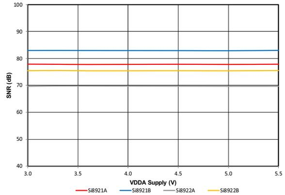
Figure 14. Signal-to-Noise Ratio (dB) vs. VDDA Supply (V)
