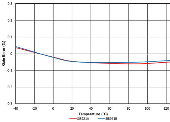
Figure 27. Gain Error (%) vs. Temperature (°C)
