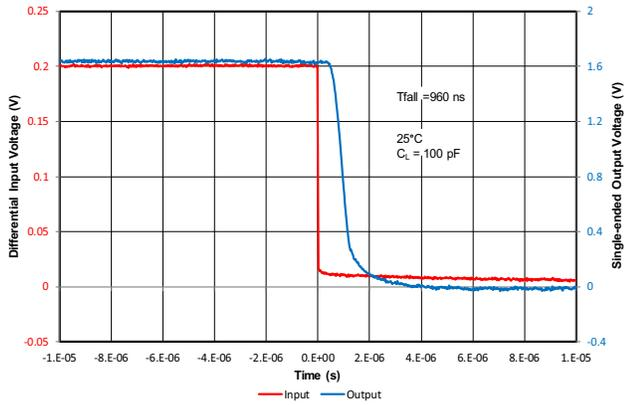
Figure 37. Si8922B High-to-Low Step Response
