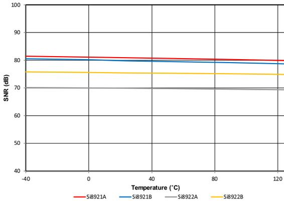
Figure 13. Signal-to-Noise Ratio (dB) vs. Temperature (°C)
