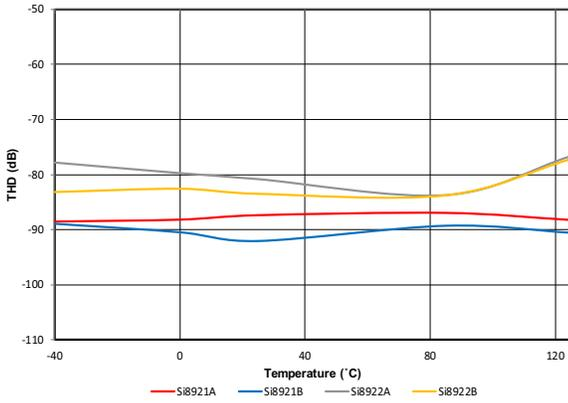
Figure 19. Total Harmonic Distortion (dB) vs. Temperature (°C)
