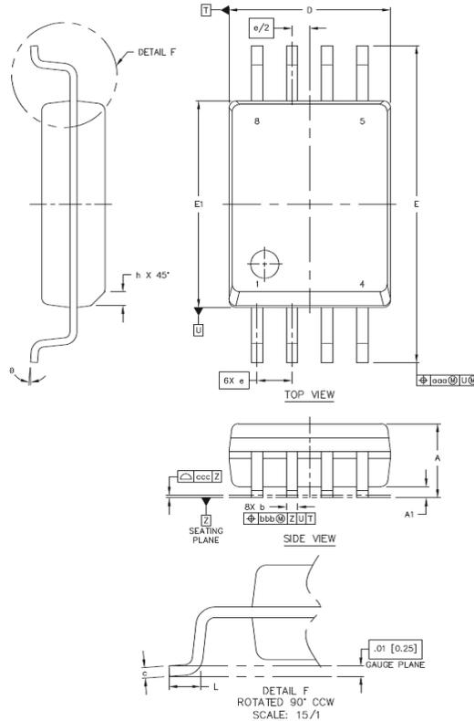
Figure 43. 8-Pin Wide Body Stretched SOIC Package
