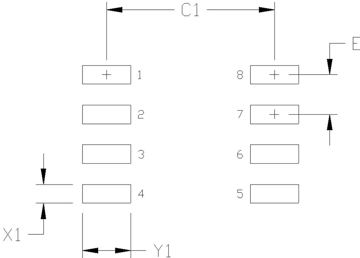
Figure 46. 8-Pin Narrow Body SOIC Land Pattern
