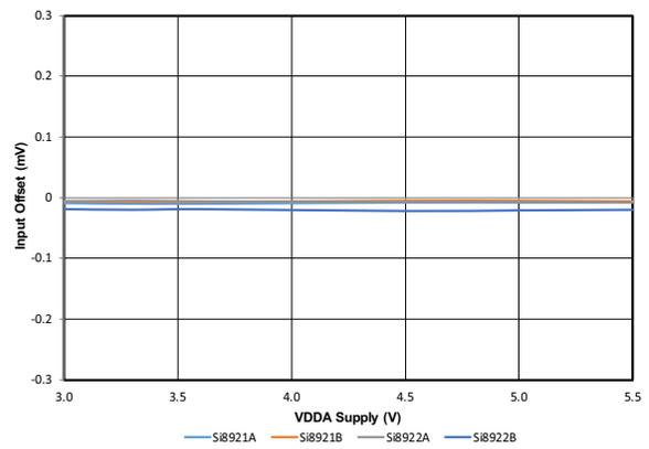
Figure 26. Input Offset (mV) vs. VDDA Supply (V)
