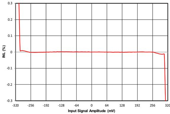
Figure 9. Si8921B Nonlinearity (%) vs. Input Signal Amplitude (mV)
