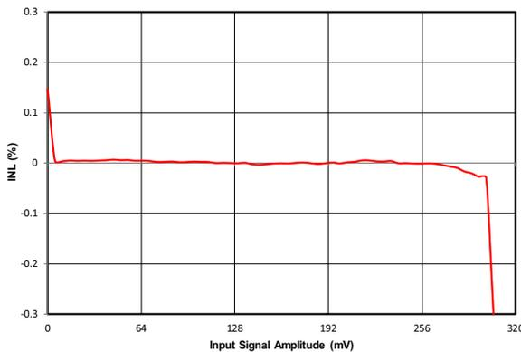
Figure 11. Si8922B Nonlinearity (%) vs. Input Signal Amplitude (mV)
