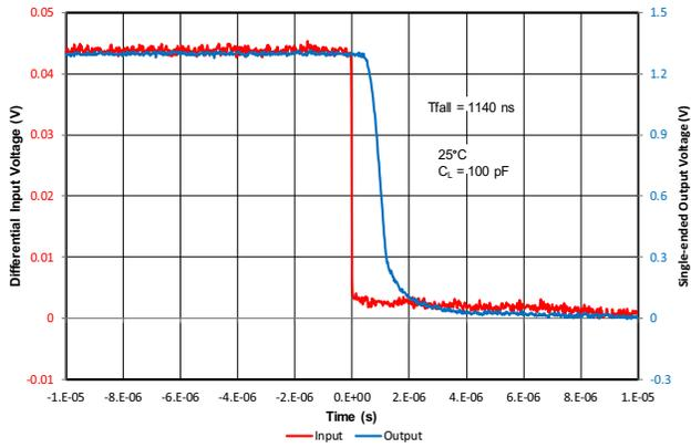
Figure 39. Si8922A High-to-Low Step Response
