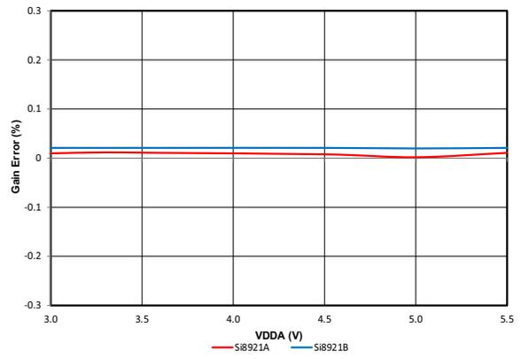
Figure 28. Gain Error (%) vs. VDDA Supply (V)
