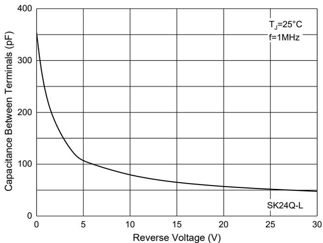
Fig. 8 - Capacitance Characteristics
