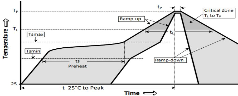
The part may be reflowed 2 times without degradation (typical for lead free processing).
