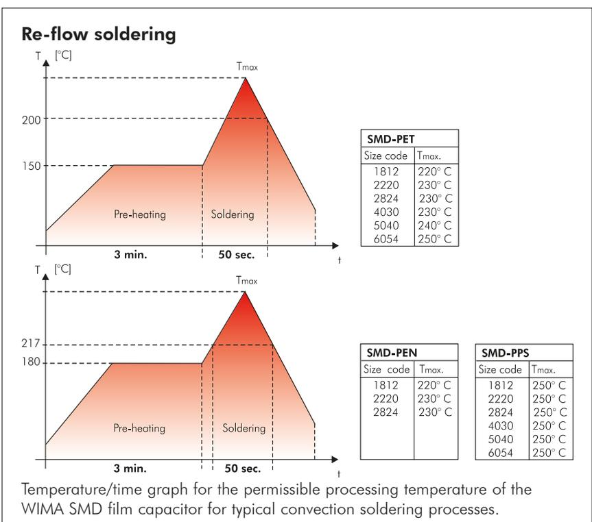
Due to versatile procedures exact processing parameters for re-flow soldering processes cannot be specified. The graph depicted is to be understood as a recommendation to help establishing a suitable soldering profile fulfilling the requirements
