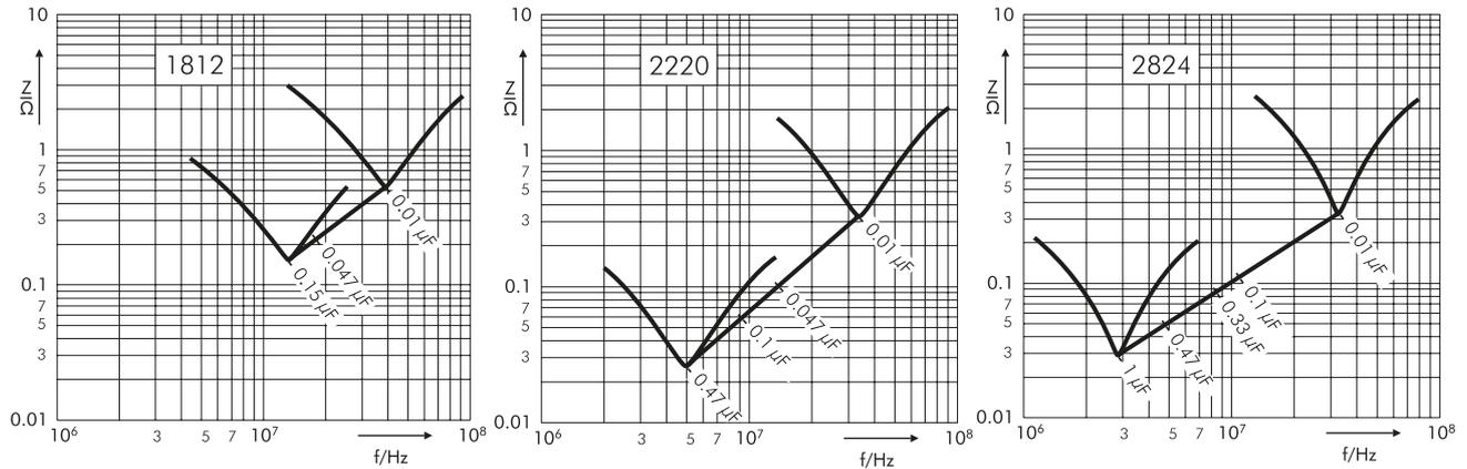
Permissible AC voltage in relation to frequency at 10° C internal temperature rise
