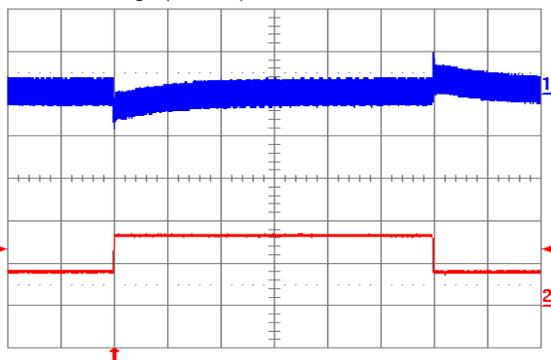
Fig. 11: Output voltage response to load current step-change (0.825 A – 1.65 A – 0.825 A) at  $V_{in} = 24\text{ V}$ . Top trace: output voltage (200 mV/div.). Bottom trace: load current (1 A/div.). Current slew rate: 0.1 A/ $\mu\text{s}$ .  $C_o = 1\ \mu\text{F}$  ceramic. Time scale: 0.5 ms/div.
