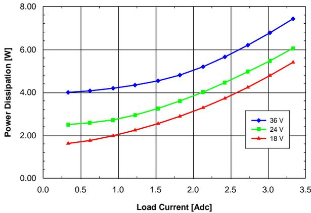
Fig. 7: Power dissipation vs. load current and input voltage for SQ24T/S03150 converter mounted vertically with air flowing from pin 3 to pin 1 at a rate of 300 LFM (1.5 m/s) and  $T_a = 25^\circ\text{C}$ .
