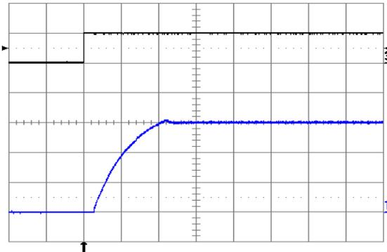
Fig. 10: Turn-on transient at full rated load current (resistive) plus 1,000  $\mu\text{F}$  at  $V_{in} = 24\text{ V}$ , triggered via ON/OFF pin. Top trace: ON/OFF signal (5 V/div.). Bottom trace: output voltage (5 V/div.). Time scale: 5 ms/div.
