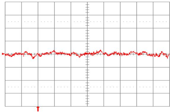
Fig. 16: Input reflected ripple current,  $i_s$  (10 mA/div.), measured through  $10 \mu\text{H}$  at the source at full rated load current and  $V_{in} = 24 \text{ V}$ . Refer to Fig. 14 for test setup. Time scale:  $1 \mu\text{s}/\text{div}$ .
