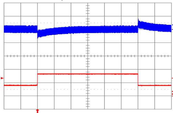
Fig. 12: Output voltage response to load current step-change (0.825 A – 1.65 A – 0.825 A) at  $V_{in} = 24\text{ V}$ . Top trace: output voltage (200 mV/div.). Bottom trace: load current (1 A/div.). Current slew rate: 5 A/ $\mu\text{s}$ .  $C_o = 47\ \mu\text{F}$  tantalum + 1  $\mu\text{F}$  ceramic. Time scale: 0.5 ms/div.
