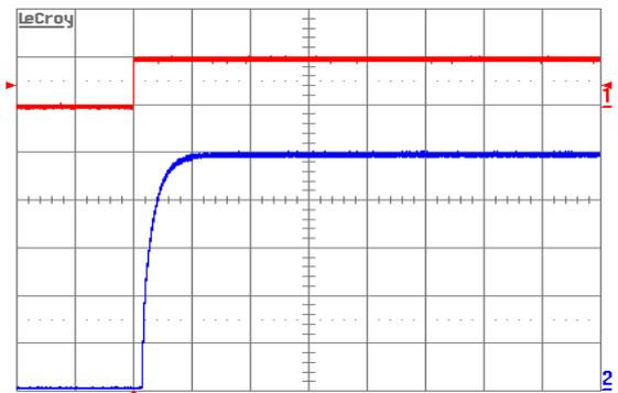
Figure 6. Turn-on transient at full rated load current (resistive) with no output capacitor at  $V_{in} = 48\text{ V}$ , triggered via ON/OFF pin. Top trace: ON/OFF signal (5 V/div.). Bottom trace: Output voltage (1.0 V/div.). Time scale: 5 ms/div.
