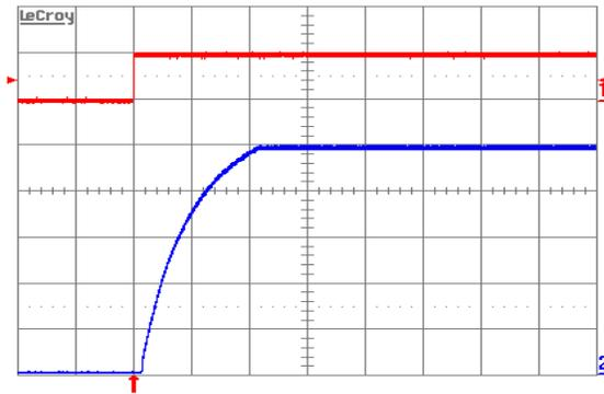
Figure 7. Turn-on transient at full rated load current (resistive) plus 10,000  $\mu\text{F}$  at  $V_{in} = 48\text{ V}$ , triggered via ON/OFF pin. Top trace: ON/OFF signal (5 V/div.). Bottom trace: Output voltage (1 V/div.). Time scale: 5 ms/div.
