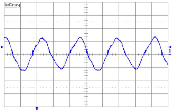
Figure 10. Output voltage ripple (20 mV/div.) at full rated load current into a resistive load with  $C_o = 10\mu\text{F}$  tantalum + 1  $\mu\text{F}$  ceramic and  $V_{in} = 48\text{ V}$ . Time scale: 1  $\mu\text{s}$ /div.
