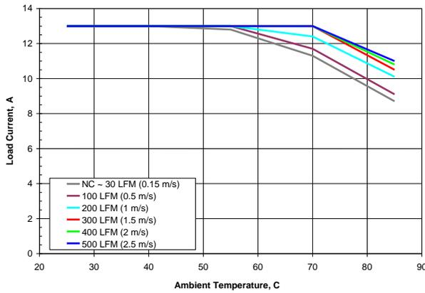
Figure 1. Available load current vs. ambient air temperature and airflow rates for SSQE48T13050 converter mounted vertically with air flowing from pin 1 to pin 3,  $V_{in} = 48\text{ V}$ .
