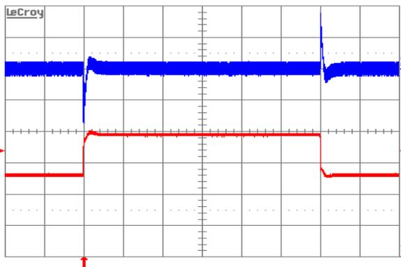
Figure 9. Output voltage response to load current step-change (12.5A–18.75A–12.5A) at  $V_{in} = 48\text{ V}$ . Top trace: output voltage (100 mV/div.). Bottom trace: load current (5A/div.). Current slew rate: 5A/ $\mu\text{s}$ .  $C_o = 470\mu\text{F POS} + 1\mu\text{F cer}$ . Time scale: 0.2ms/div.
