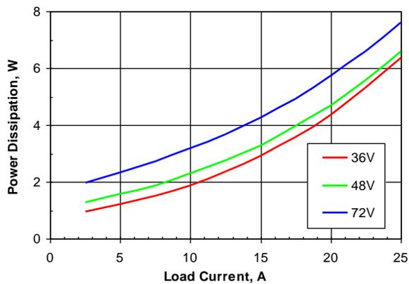
Figure 4. Power dissipation vs. load current and input voltage for SSQE48T25015 converter mounted vertically with air flowing from pin 1 to pin 3 at a rate of 300 LFM (1.5 m/s) and  $T_a = 25^\circ\text{C}$ .
