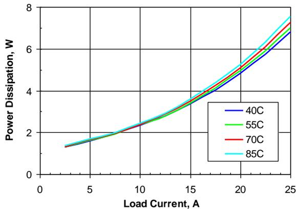
Figure 5. Power dissipation vs. load current and ambient temperature for SSQE48T25015 converter mounted vertically with  $V_{in} = 48\text{ V}$  and air flowing from pin 1 to pin 3 at a rate of 200 LFM (1.0 m/s).
