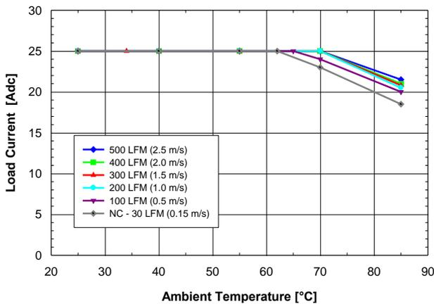
Figure 1. Available load current vs. ambient air temperature and airflow rates for SSQE48T25015 converter mounted vertically with air flowing from pin 1 to pin 3,  $V_{in} = 48\text{V}$ . Note: NC – Natural convection
